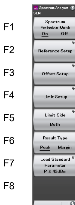
Figure 7.6-1 Spectrum Emission Mask function menu
