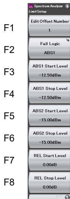
Figure 7.6-4 Limit Setup function menu
