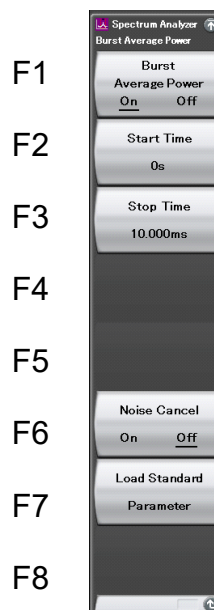
Figure 7.3-1 Burst Average Power function menu
