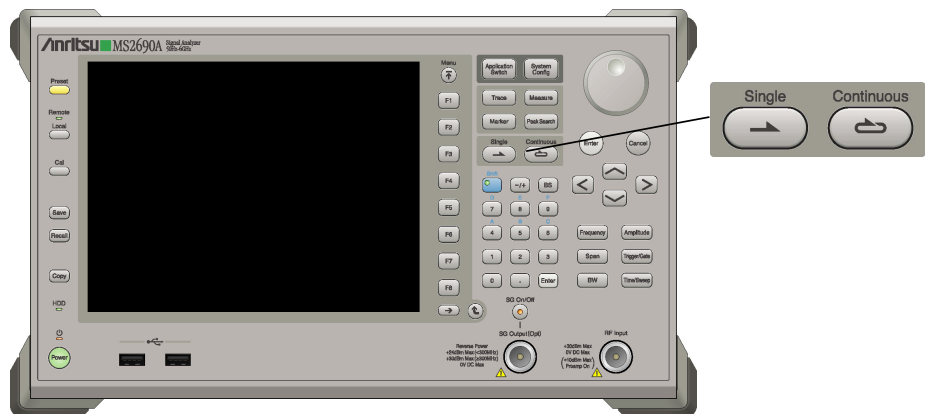
Figure 2.2-1 Single key and Continuous key
