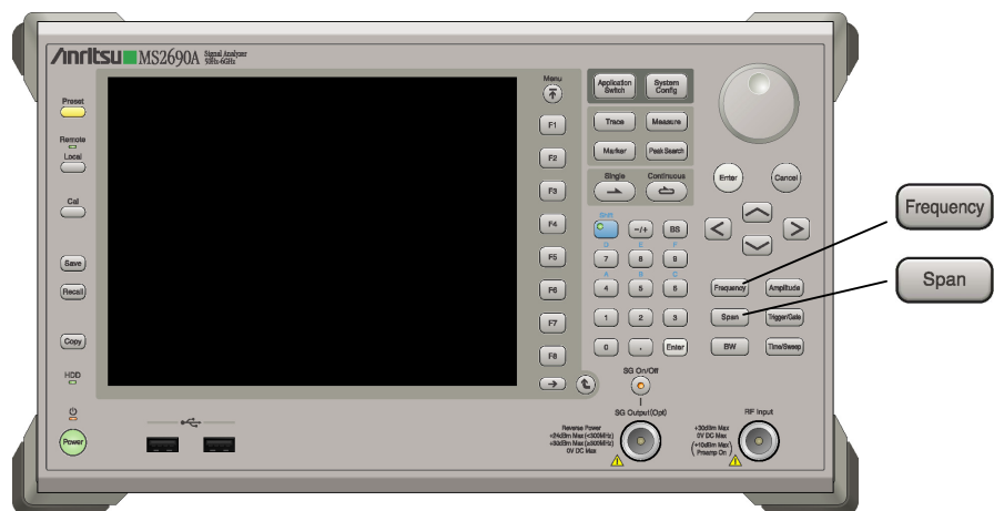
Figure 2.3-1 Frequency key and Span key
