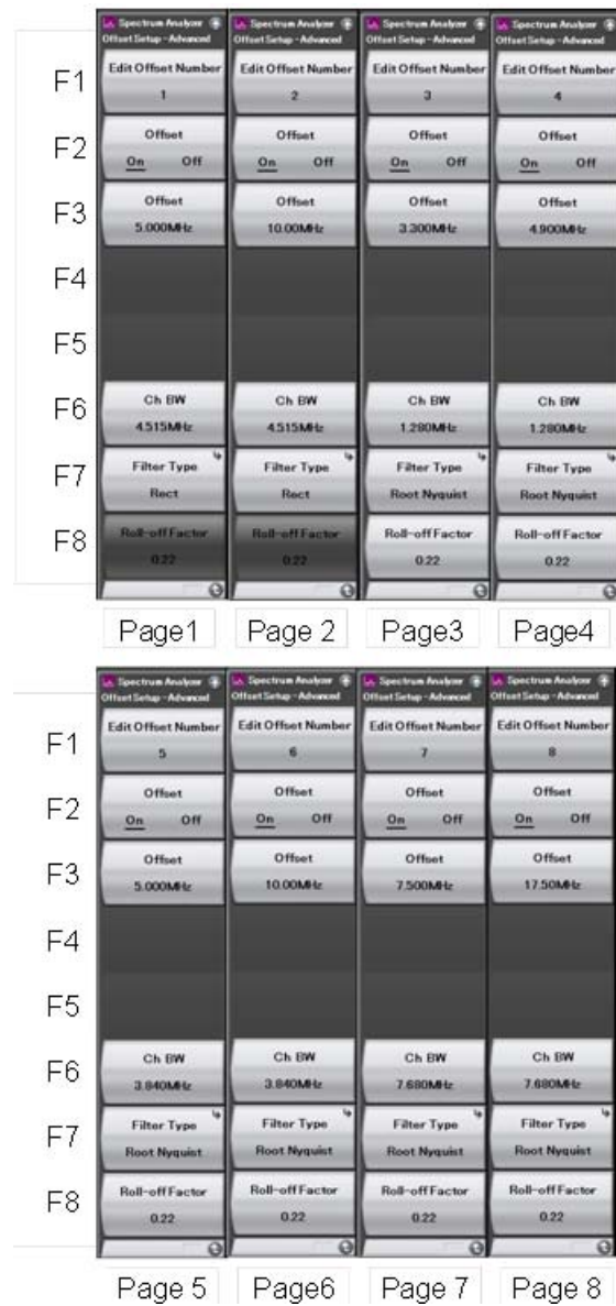
Figure 7.2-4 Offset Setup (Advanced) function menu
