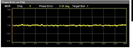
Figure 3.5.8.4-1 Phase Error vs. Chip
