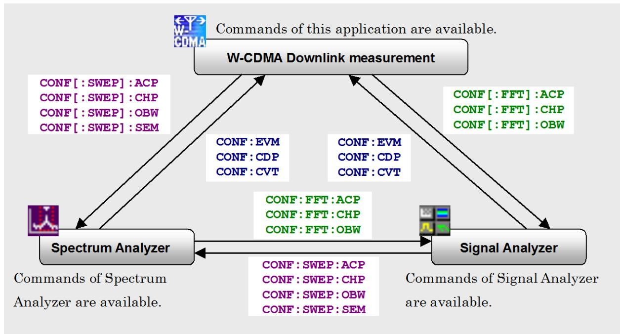
Figure 1.2.11-1 Switching of Measurement Functions among Applications
