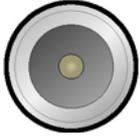
RF Output connector (when MS269xA-020/120, MS2830A-020/120/021/121 installed)
