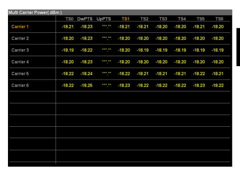
Fig. 3.13-1 Multi Carrier Power Display
