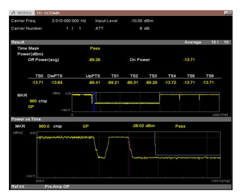
Fig. 3.14-1 Power vs Time Display
