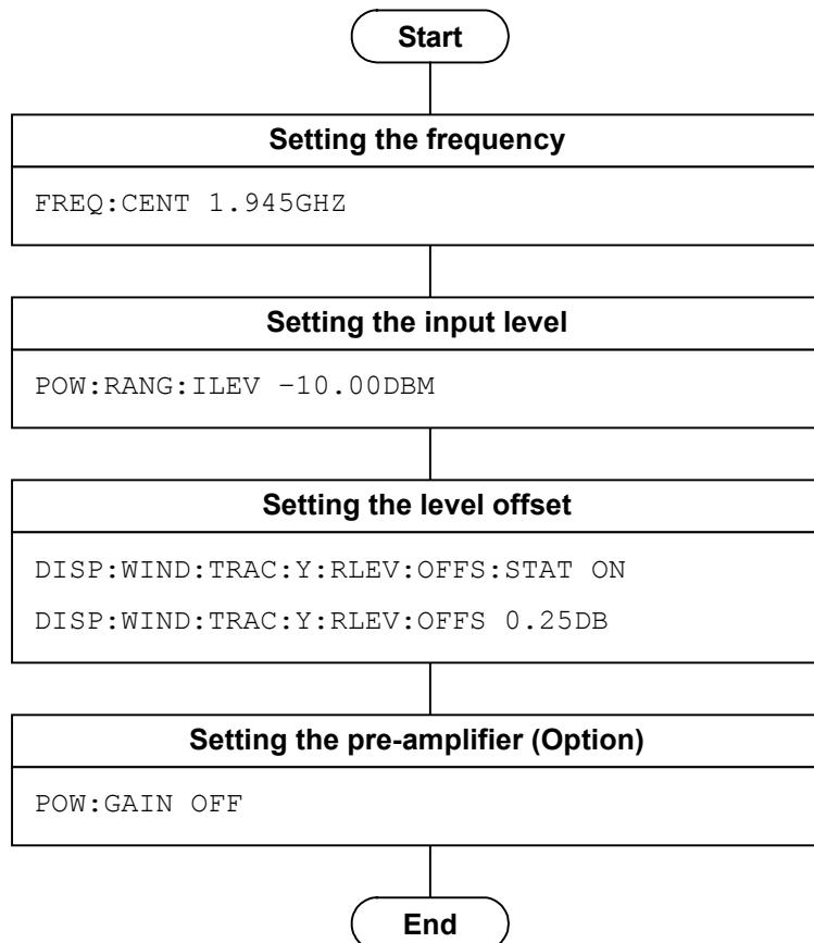
**Figure 1.2.2-1 Basic Parameter Setting Flow and Command Examples**
