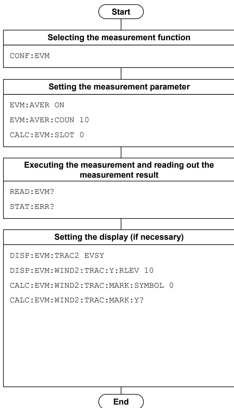
Figure 1.2.4-1 Flow of Modulation Analysis and Command Examples
