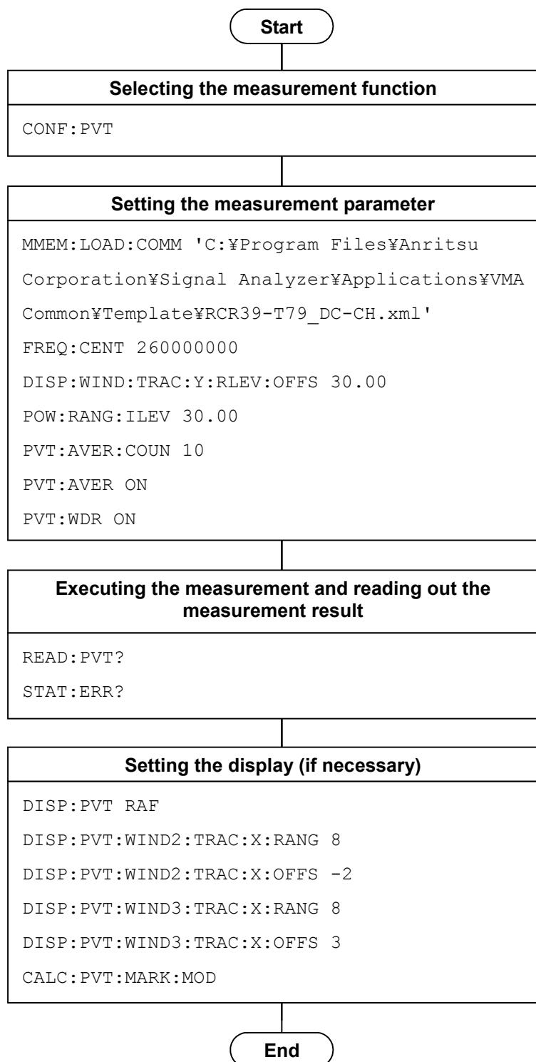
Figure 1.2.5-1 Flow of Power vs Time and Command Examples
