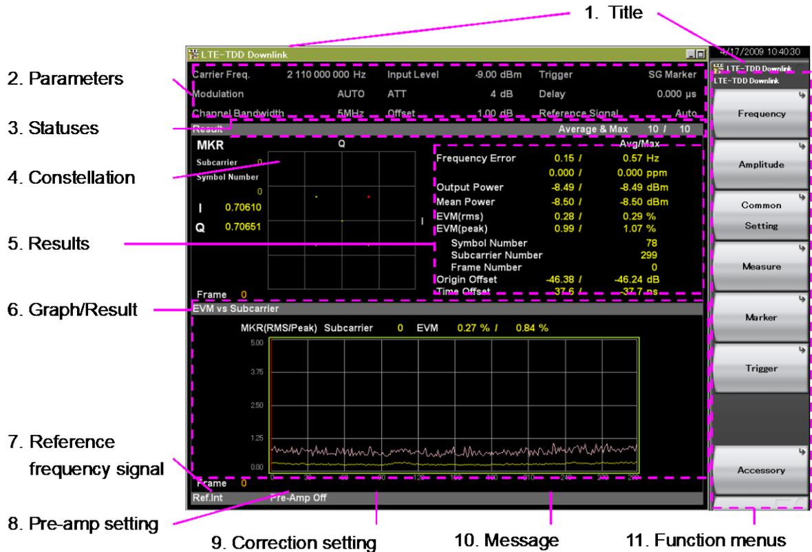
Figure 3.1.1-1 Screen Appearance (Modulation Analysis)
