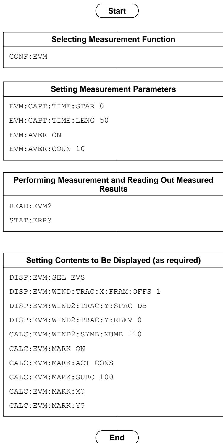
**Figure 1.2.4-1 Flow of Modulation Measurement and Command Example**
