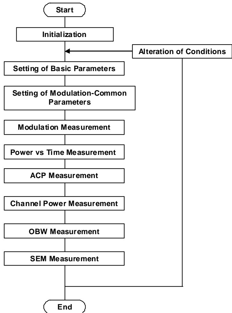
Figure 1.2-1 Flow of Basic Test
