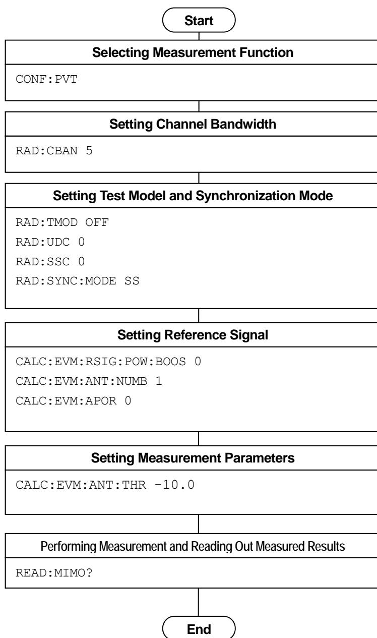
Figure 1.2.6-1 Flow of MIMO Summary Measurement and Command Example
