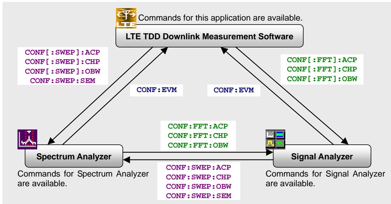
**Figure 1.2.11-1     Switching of Measurement Functions among Applications**
