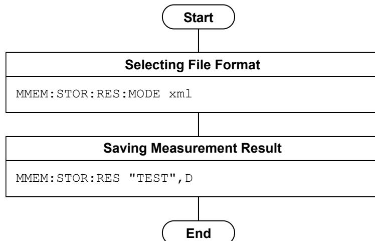
**Figure 1.2.9-1 Saving Measurement Results Flow and Command Example**
