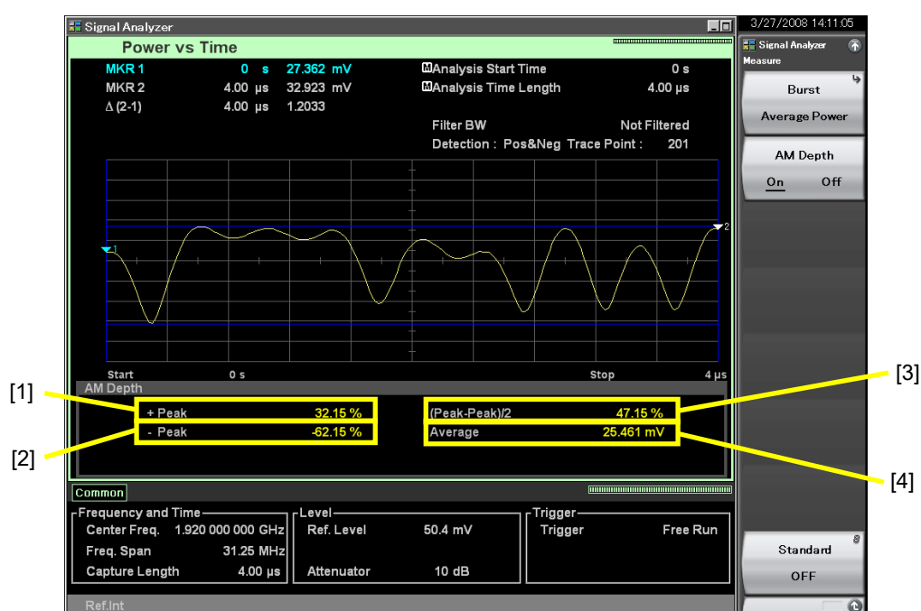
Figure 4.3.11-6 AM Depth measurement result
