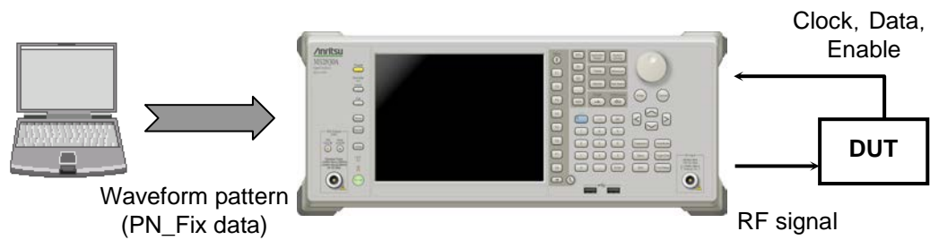
Figure 8.8-6 BER measurement using PN_Fix data
