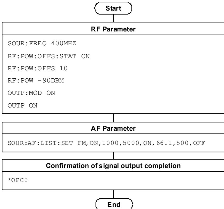
**Figure 1.2.5-3 RX Measurement Setting Flow and Command Example**
