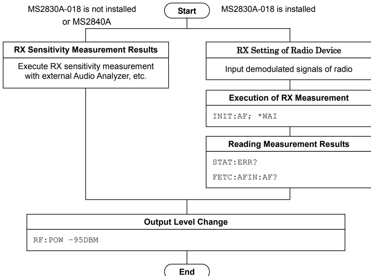
**Figure 1.2.6-1 RX Measurement Execution Flow and Command Example**
