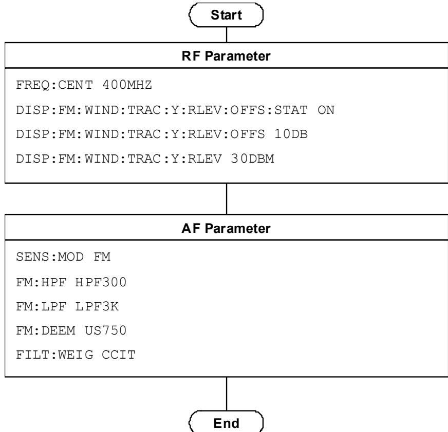
Figure 1.2.3-3 TX Measurement Setting Flow and Command Example
