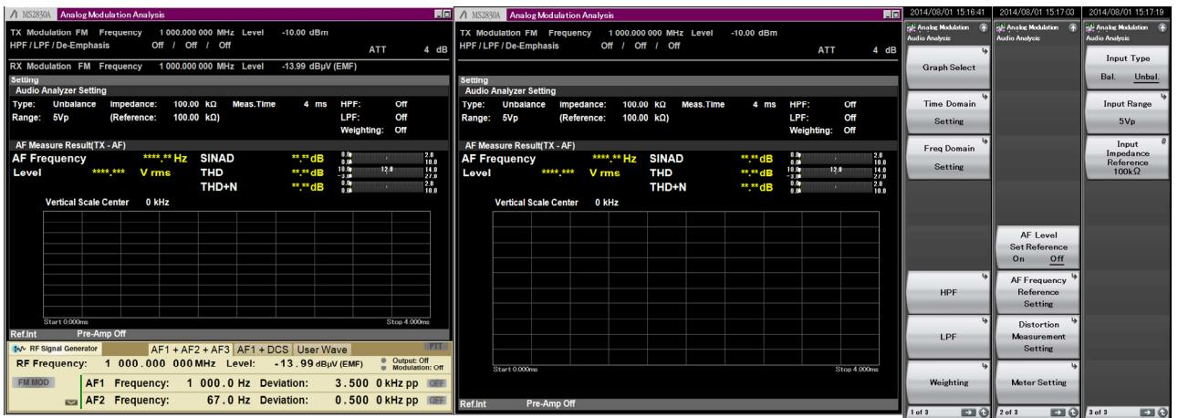
RX mode window when the SG application (MS2830A-029/129/088/188) and MS2830A-018/118 is installed.
