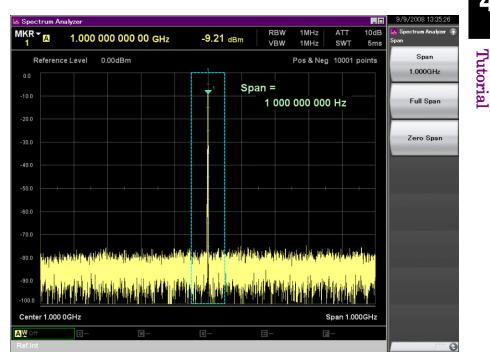
Figure 4.2.1-4 Waveform display using Spectrum Analyzer
