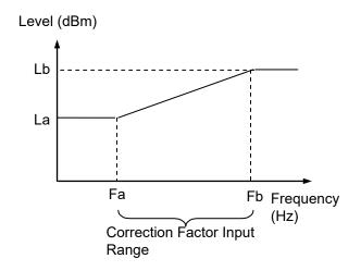
Figure 3.4.10-1 Operation When Correction Factors Are Entered
