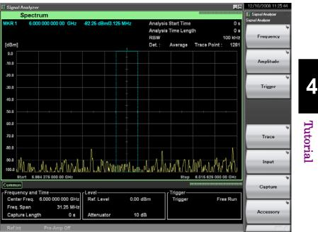
Figure 4.1.1-4 Waveform display using Signal Analyzer
