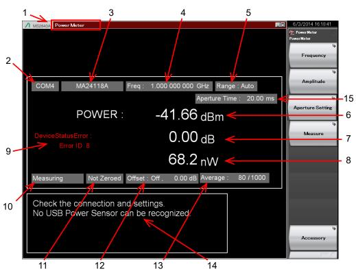
Figure 7.2-1 Power meter application main screen
