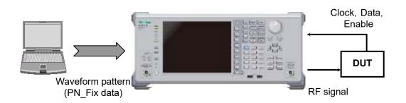
Figure 8.8-6 BER measurement using PN\_Fix data
