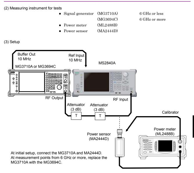
Figure 6.2.4-1 RF frequency characteristics test
