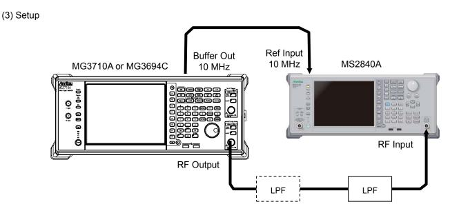
Figure 6.2.6-1 Second harmonic wave distortion test
