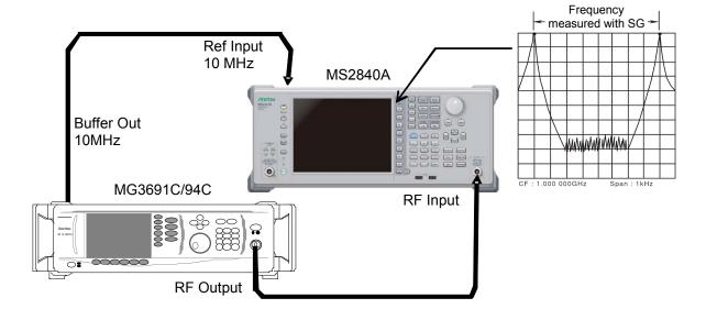
Figure 6.2.2-1 Frequency span display accuracy test
