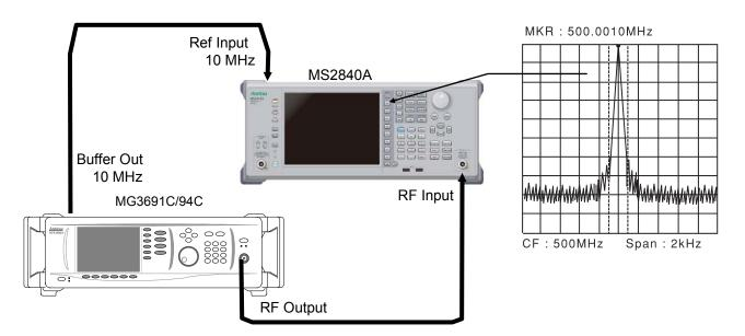
Figure 6.2.1-1 Display frequency accuracy test
