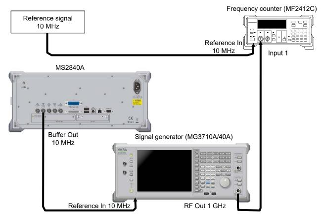
Figure 9.3.3-1 Connections for frequency calibration using frequency counter
