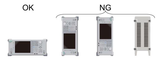
Figure 2.1.1-1 Installation orientation
