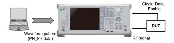
Figure 8.8-6 BER measurement using PN\_Fix data
