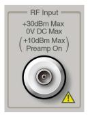
When Option 046 is installed: Type K connector
