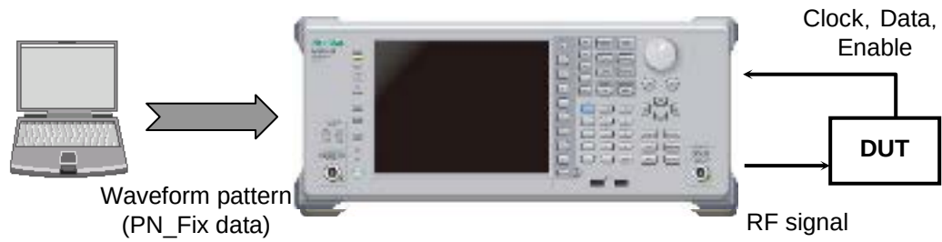
Figure 8.8-6 BER measurement using PN_Fix data
