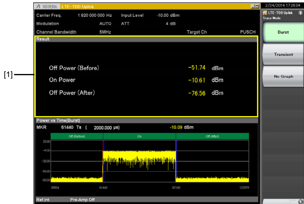
Figure 3.18-1 The display of Power vs Time
