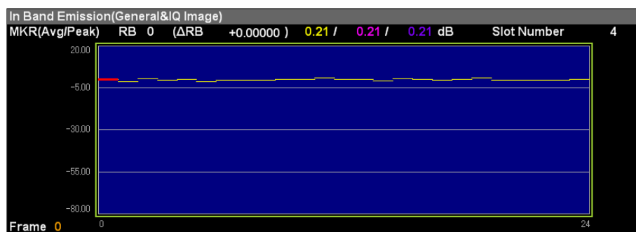
Figure 3.16-1 In-Band Emission Display (PUSCH)
