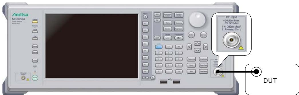
Figure 2.1-1 Signal path setup example
