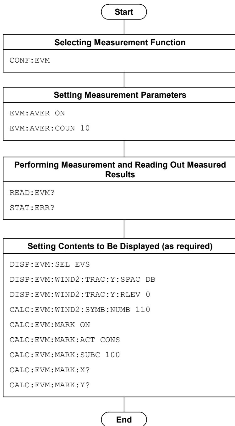
**Figure 1.2.4-1 Flow of Modulation Measurement and Command Example**
