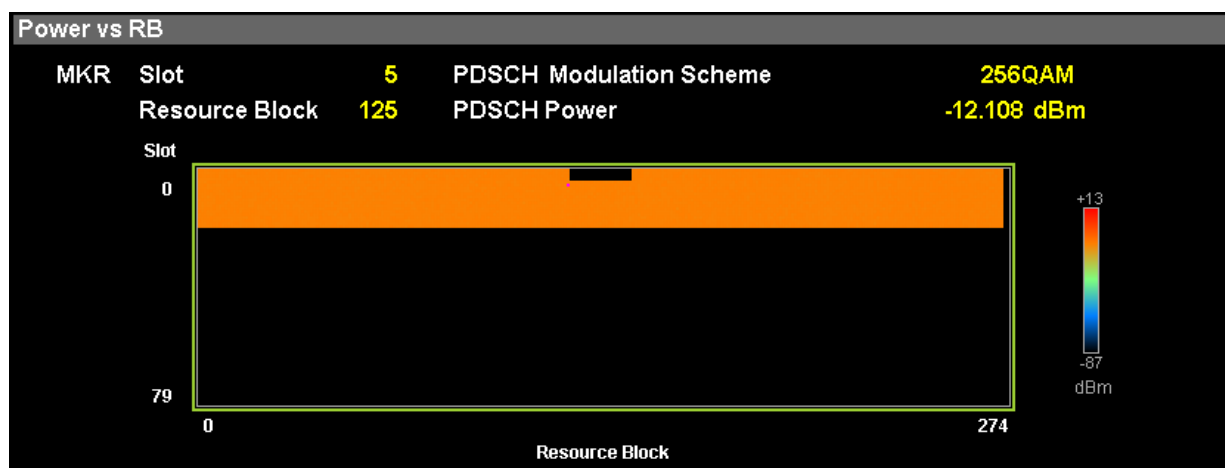
Figure 3.15-1 Power vs Resource Block display
