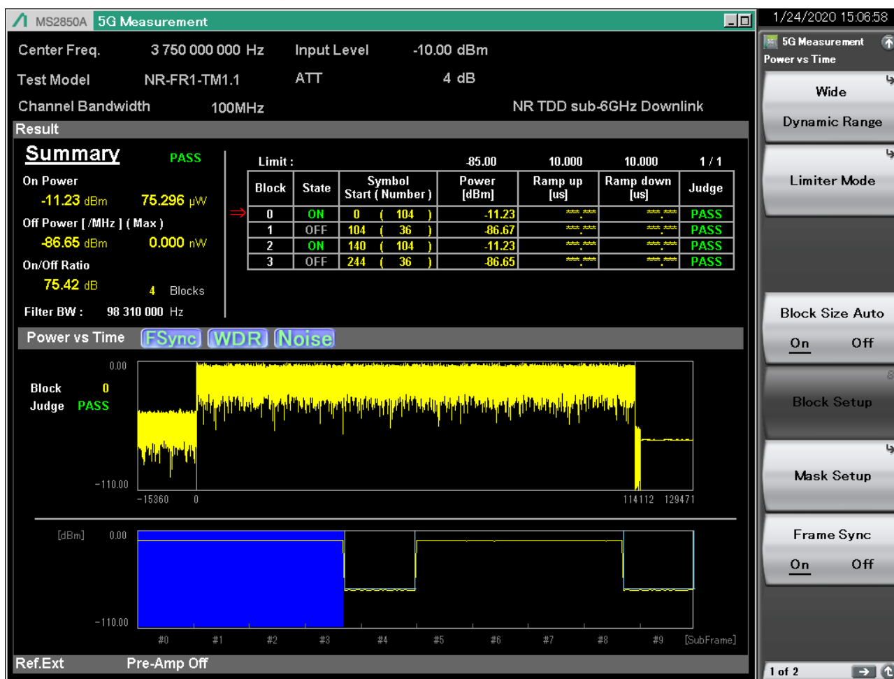
Figure 3.6.3-1 Power vs Time Measurement Screen
