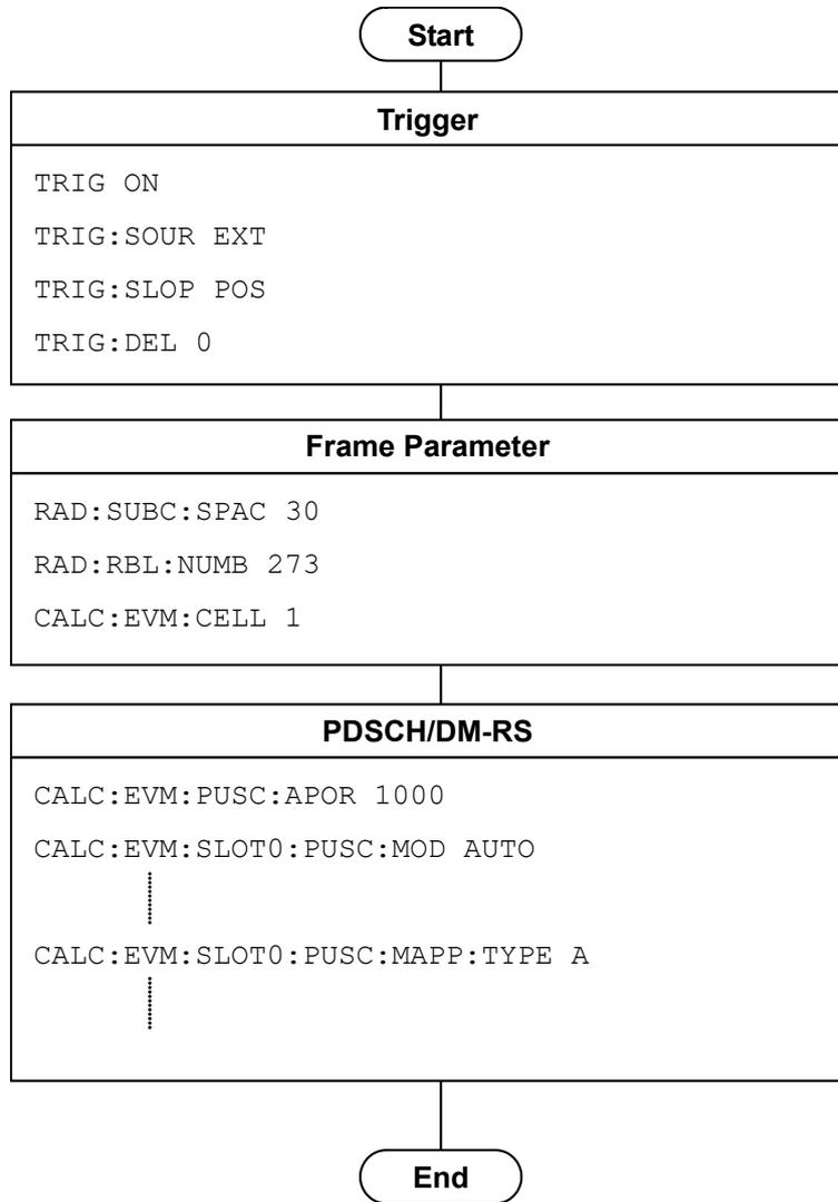
Figure 1.2.3-2 Flow of Common Settings for Modulation and Command Example
