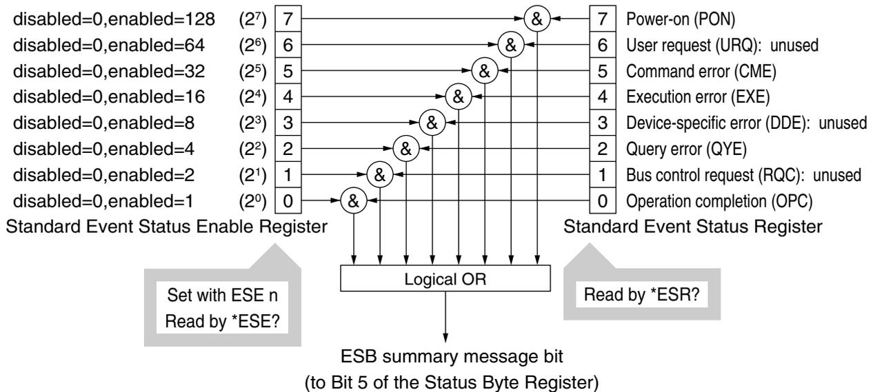
The Standard Event Status Enable register on the left side selects whether the summary message should be set to True when any bit of the corresponding Event register is set to 1.
