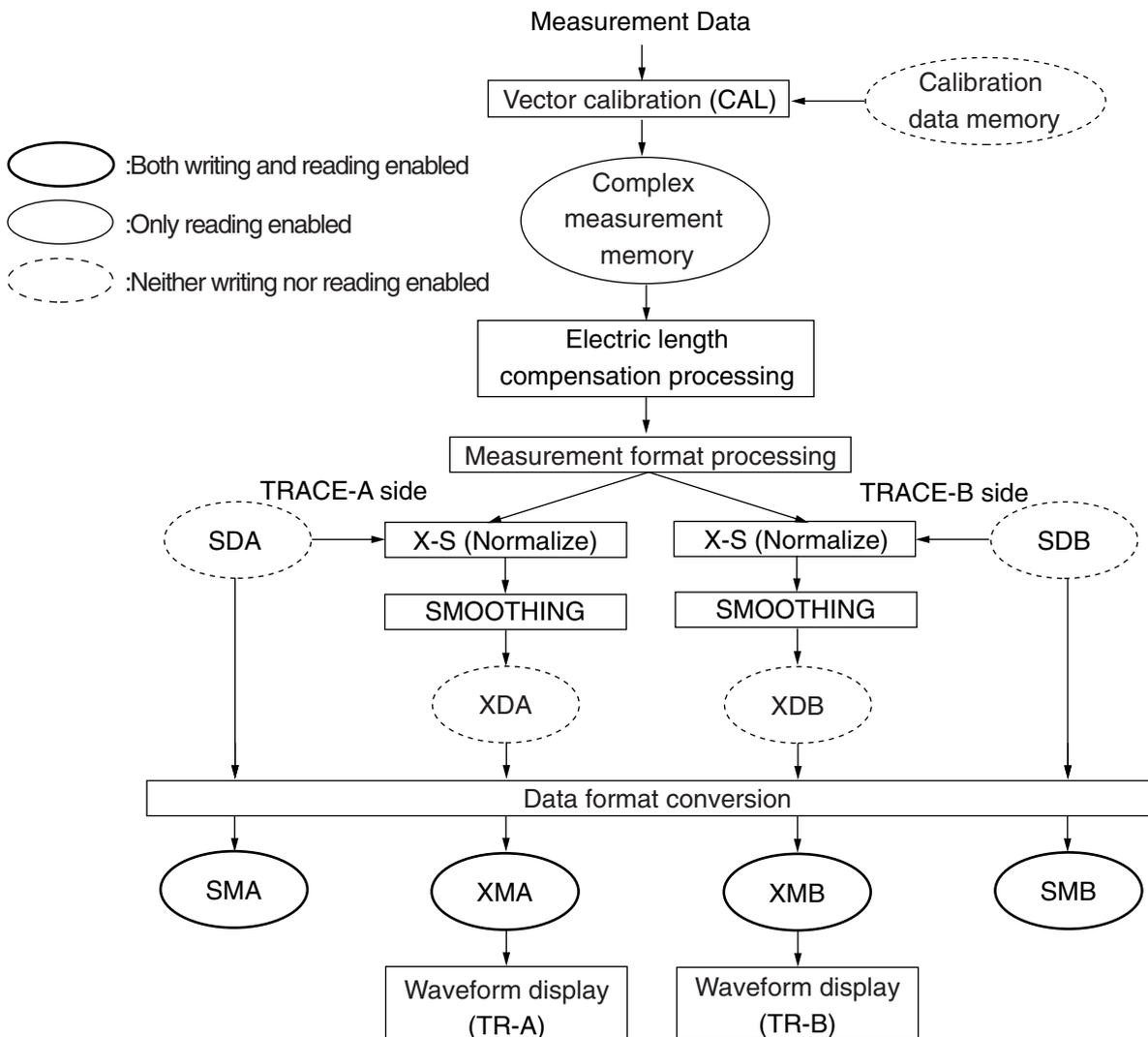
**Measurement Memory/Waveform Memory Calibration Flow**
