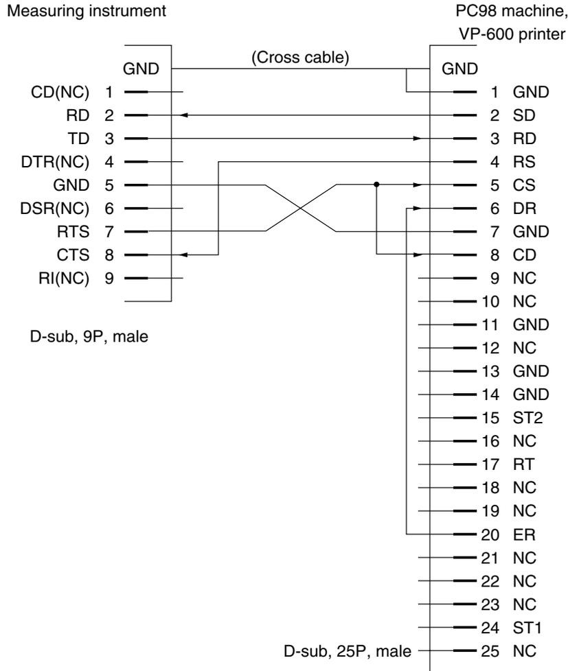
**Connection diagram with a PC98 machine, or VP-600 printer**
