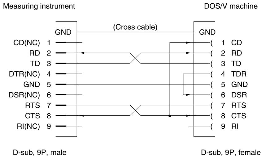
**Connection diagram with a DOS/V machine**
