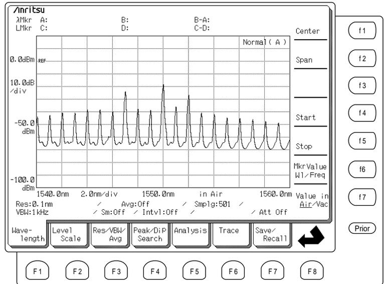
Set the best measurement conditions while using the Repeat Sweep function. Press the Single key **Single** of Sweep keys after confirming the measurement conditions, that completes measurement after one sweep. To terminate a measurement during the sweep, press the Stop key **Stop** of the Sweep keys.
