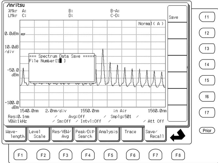
This example explains how to save the data to file number 1. When 1 is input as the file number, a file called “data001.dat” is created on the FD. The name of the file created at this time may be different such as “data001,bmp” or “data001.txt” depending on the File Option settings of Save/Recall card.
