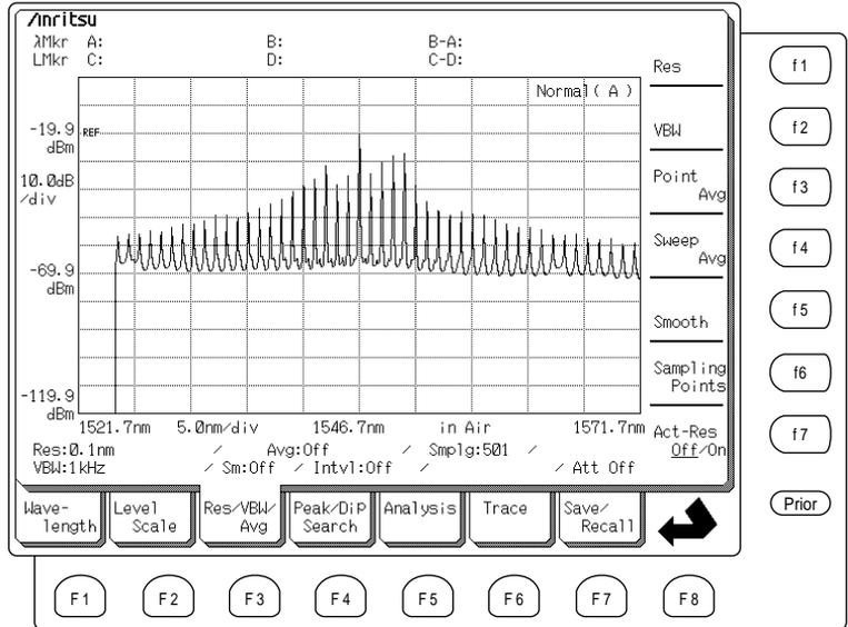
(11) Set the Span (sweep width) to 20 nm.
