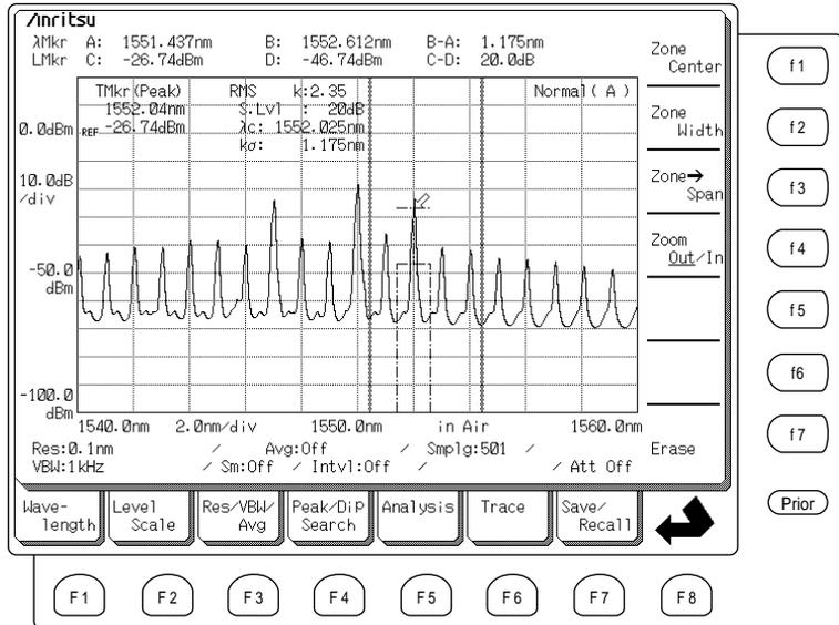
This Zone Marker function is useful for analyzing a specific spectrum individually while monitoring several spectra simultaneously as in WDM applications, etc.
