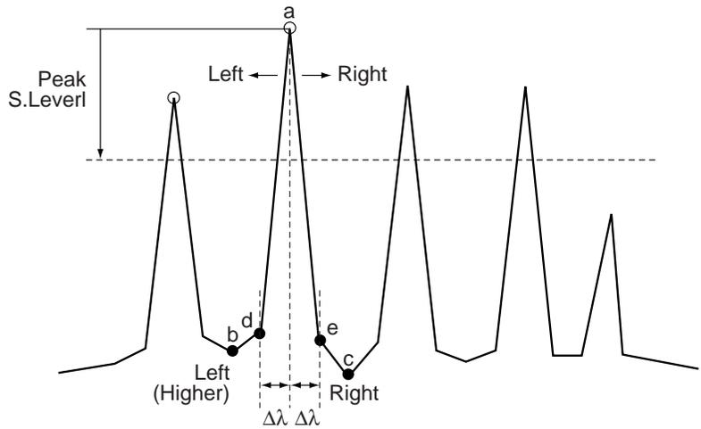
The peak level  $L_p$  [dBm] detects the value of peak point a. The peak wavelength  $\lambda_p$  is the wavelength of peak a when Peak Type of Peak Prmtr is set to MAX and the half-width center wavelength of the peak when Peak Type is set to Threshold.
