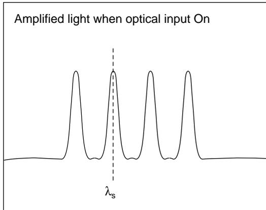
Measurement is performed with automatical evaluation whether or not wavelength of the optical signal is modulated by switching the optical input On and Off.
