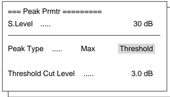
Set the target for peaks to be analyzed up to X dB below the maximum peak at S.Level in the Peak Prmtr window. Select whether to use the wavelength of the point with the maximum measured level (MAX), or the center wavelength using Threshold analysis (Threshold) as the peak wavelength detection method at Peak Type. In both cases, the peak level is the level of the point measured as the peak.
