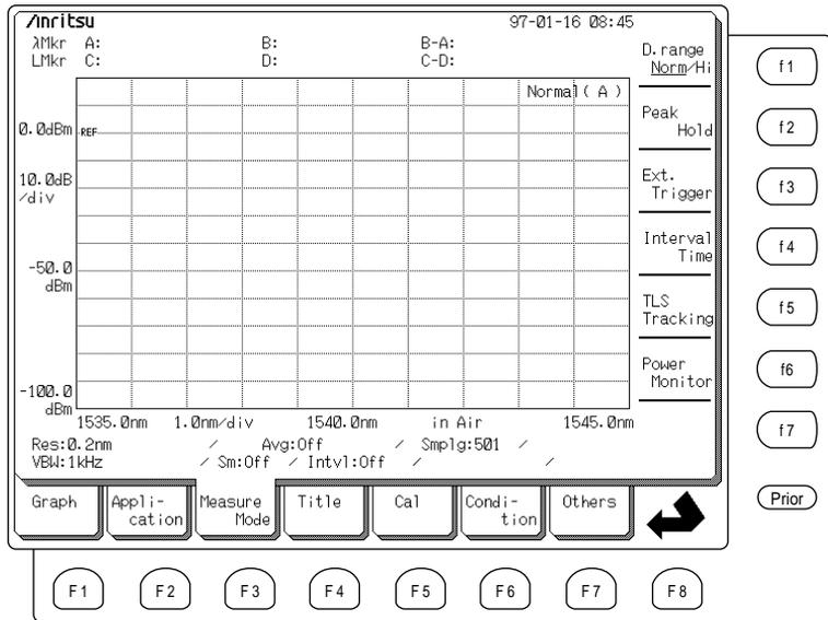
Press the Adjust to TLS function key (f2) then select Execute by pressing the function key (f1), which sets the measurement conditions automatically and start calibration. Calibration of the tracking wavelength will take about a few minutes.
