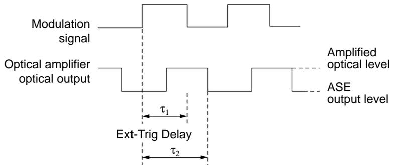
To measure the amplified optical level the Ext. Trig Delay should be set to  $\tau_1$ . The ASE output level is measured when the Ext. Trig Delay is set to  $\tau_2$ .
