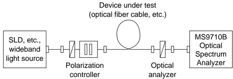
Convert the light from a wideband light source to a polarized wave using a polarization controller; pass this polarized light through the device under test, and input it to the MS9710B through an analyzer. The MS9710B measures the optical power polarization wavelength changes and calculates the PMD.
