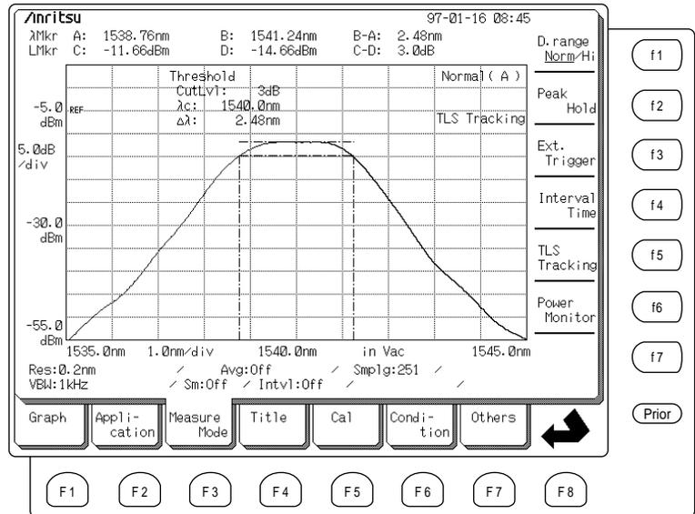
Note that during tracking measurement, the Auto measurement and the W1 Offset function key (F1) of the Cal card selected by pressing (F5) key is not possible to be used.
