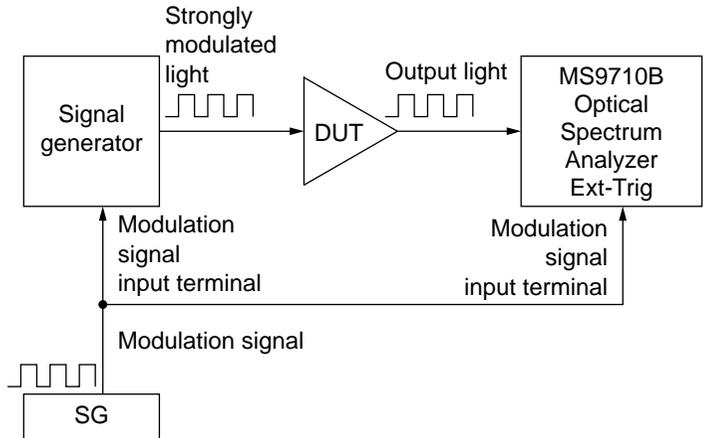
A measurement is taken  $\tau$  msec after the Ext. Trig signal rising edge. This  $\tau$  is called the Ext. Trig Delay and is set by pressing (f6). The settable Ext. Trig Delay range is 0 to 5 s. The modulated input signal is measured first and then the modulated amplified light is measured.
