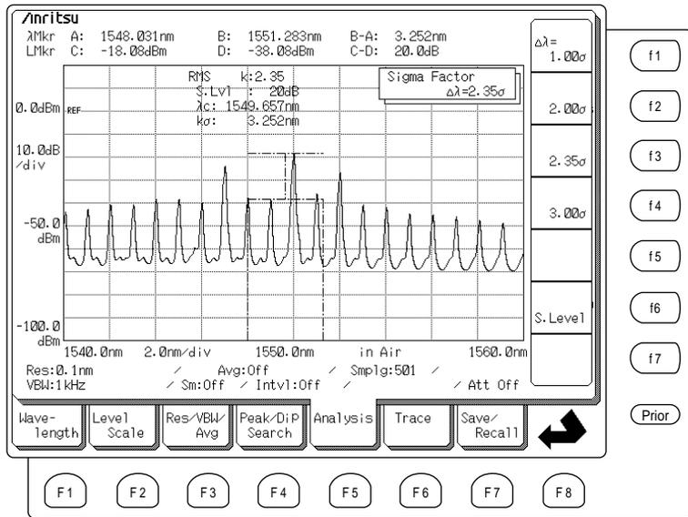
In this state, by selecting  $\Delta\lambda$  function key from the function key ability display area on the right of the screen, you can set one of analysis expressions from "1.00  $\sigma$  / 2.00  $\sigma$  / 2.35  $\sigma$  / 3.00  $\sigma$ ". In this example, 2.35  $\sigma$  is set as the expression. Also, by selecting the S. Level function key **(f6)** and using the ten keys and encoder, you can set the slice level. In this example, the slice level is set to 20 dB.
