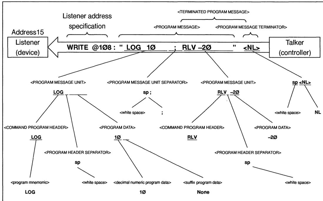
A program message is a sequence of functional elements, the minimum units that can represent functions. In the above figure, functional elements are indicated by capital characters with them enclosed in `<>`. Functional elements are further classified into coding elements which are indicated by lowercase characters with them enclosed in `<>`.
