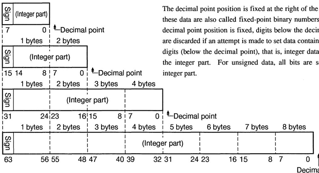
The decimal point position is fixed at the right of the LSB bit, these data are also called fixed-point binary numbers. As the decimal point position is fixed, digits below the decimal point are discarded if an attempt is made to set data containing these digits (below the decimal point), that is, integer data is set in the integer part. For unsigned data, all bits are set in the integer part.
