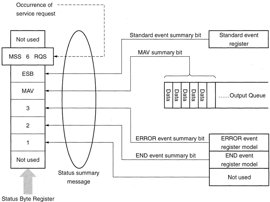
Let's take a look at definition, read, write, and clearing of END and ERROR extended event register model bits.
