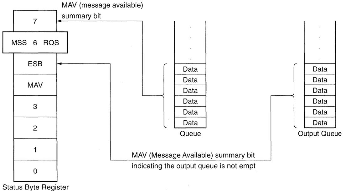
The queue that outputs an MAV summary bit to status byte register bit 4 is called an "output queue." This queue is mandatory. The queue that can output an MAC summary message to one of status byte register bits 0 to 3 and 7 is simply called a "queue." It is optional. A summary message from the register model can also be output to status byte register bits 0 to 3 and 7, so the summary message type depends on the device type.
