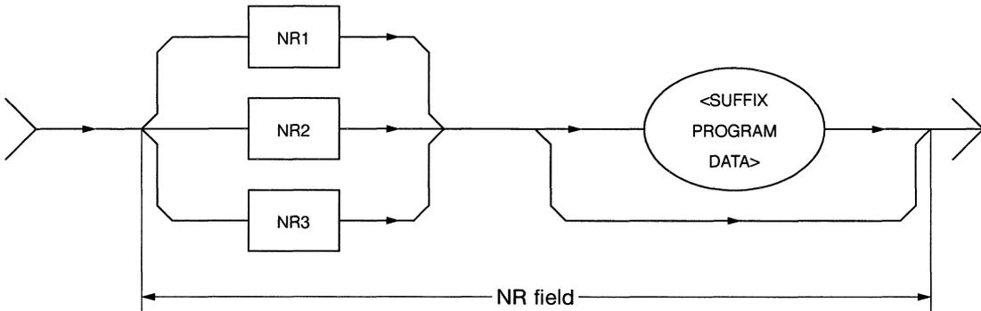
A suffix is added at the end of decimal numeric program data only when the data requires a unit of measure. It is a combination of a suffix unit and a suffix multiplier. The syntactical chart is shown below. Bold-line routes are used frequently.
