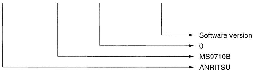
When the manufacturer of the product whose type name, serial number, and software/hardware version number are Anritsu, 0, and 1 respectively, sending a common query \*IDN? to a device will return a response message consisting of the above four fields.
