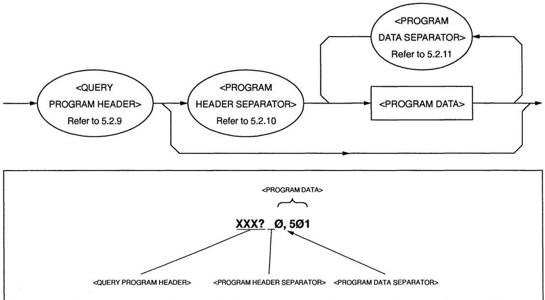
When a program header <COMMAND MESSAGE UNIT> or <QUERY MESSAGE UNIT> is followed by program data, a space is inserted between them. A program header indicates the application, function, and operation of the program. If a program header is not followed by program data, the program header solely indicates the application, function, and operation to be performed in the device.
