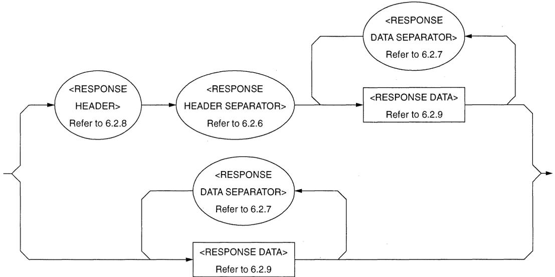
One is a response message unit with header, which returns the result of processing the program-message-set information accurately. The other is a response message unit without header, which returns only the measurement result.
