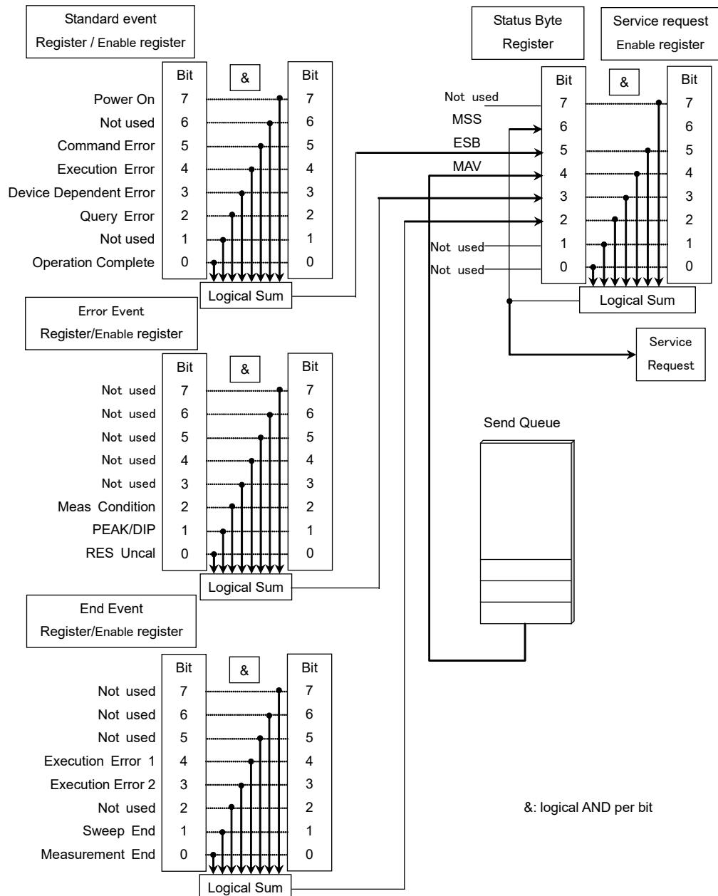
Figure 2.6.1-1 Register Structure
