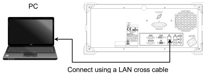
**Figure 2.2.1-1 Sample Connection with One External Device**
