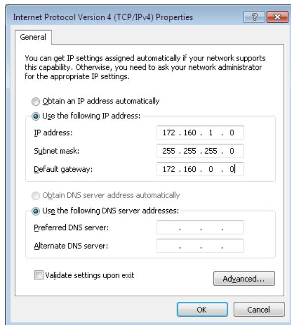
**Figure 2.3.1-9 Internet Protocol Version 4 (TCP/IPv4) Properties Dialog Box**
