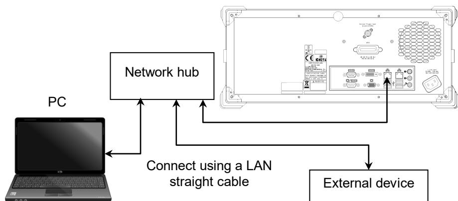
**Figure 2.2.1-2 Sample Connection with Multiple External Devices**
