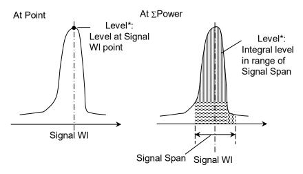
Figure 5.6.1-4 Measurement Method for Level
