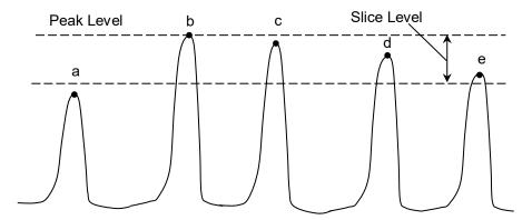
Figure 5.5.2-2 WDM Analysis Target Peaks
