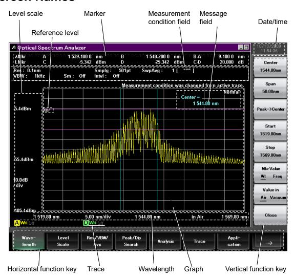
Figure 2.12-1 Measurement Screen
