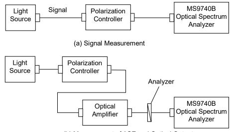
(b) Measurement of ASE and Optical Output
