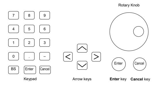
Figure 3.3-1 Data Input Keys and Rotary Knob
