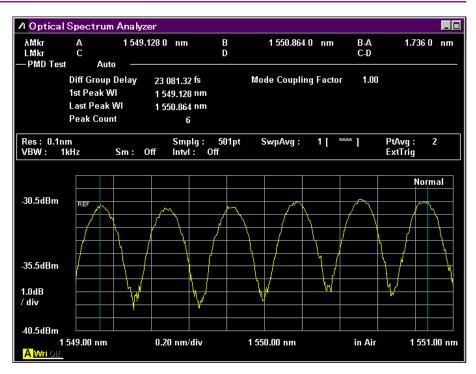
Figure 5.4-2 PMD-Test Example
