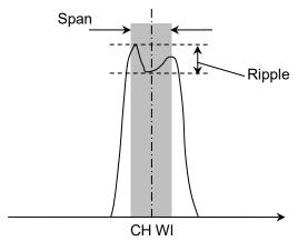
Figure 5.9.3-5 Measurement Method for Ripple
