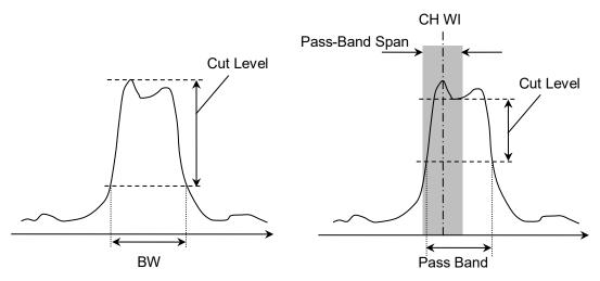
Figure 5.9.3-4 Measurement Method for Bandwidth
