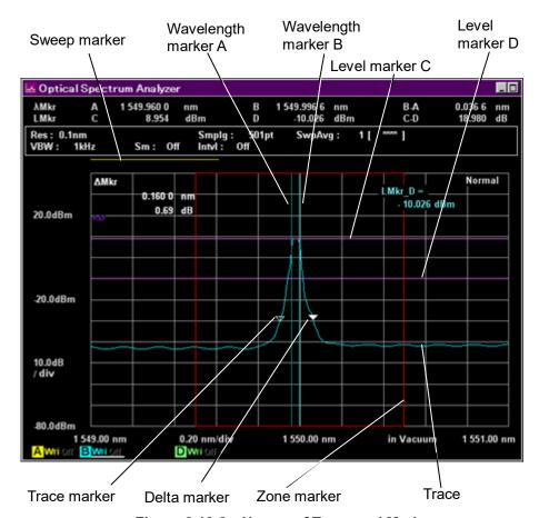
Figure 2.12-2 Names of Trace and Marker
