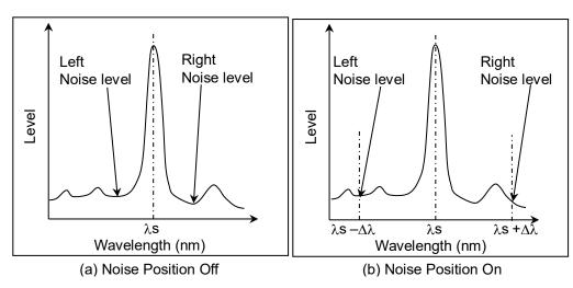
Figure 5.6.2-3 Measurement of Noise at Noise Position
