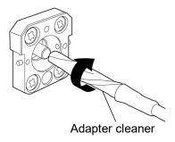
Figure 7.4-2 Cleaning the Ferrule End Surface 2
