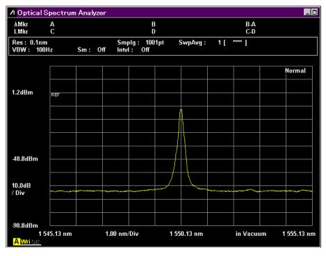
Figure 1.3-3 Example of Measurement at VBW 100Hz
