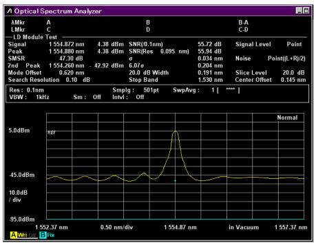
Figure 5.6-1 LD Module-Test Example
