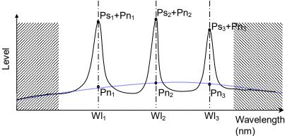
Figure 5.5.4-2 Fitting Curve and Noise Level when Area Type is User Specify
