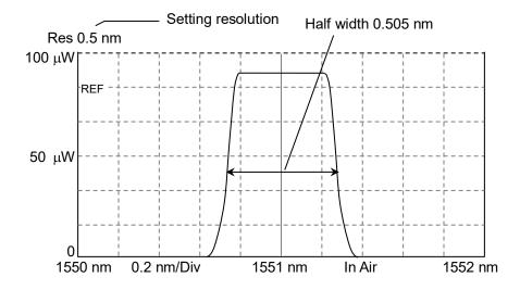
Figure 1.3-6 Measurement Example of Resolution 0.5 nm
