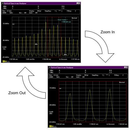
Figure 3.7.1-6 Enlarged Zone Marker Display
