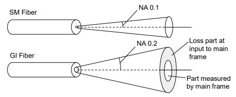
Figure 2.7-1 Difference in light radiated from optical fibers
