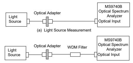
(b) Measurement of Light Passed Through WDM Filter
