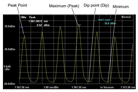
Figure 4.4-1 Waveform Peaks and Dips
