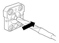
Figure 7.4-3 Cleaning the Ferrule End Surface 3
