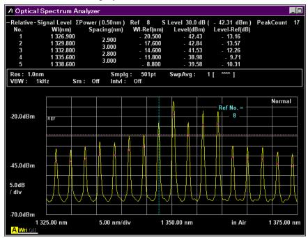
Figure 5.5.1-3 WDM Relative Display Example
