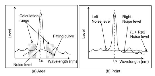
Figure 5.6.2-2 Detection Method for Noise Level
