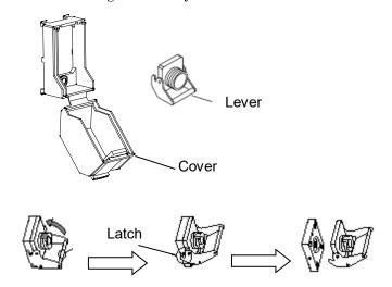
Figure 7.3-2 How to Remove the Optical Connector
