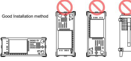
Figure 2.1.2-1 Installation Orientation
