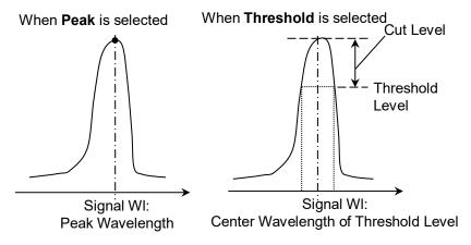
Figure 5.5.2-3 Measurement Method for Signal Wavelength
