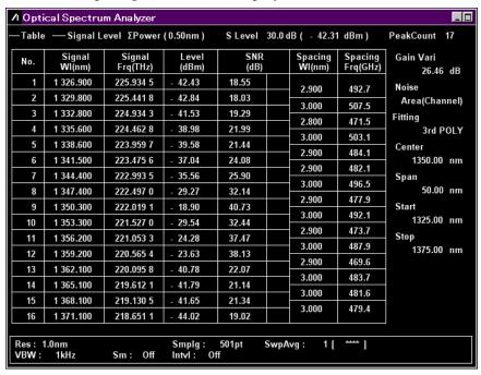
Figure 5.5.1-4 WDM Table Display Example
