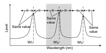
Figure 5.8.4-1 Integration Range for Signals in Multiple Channels
