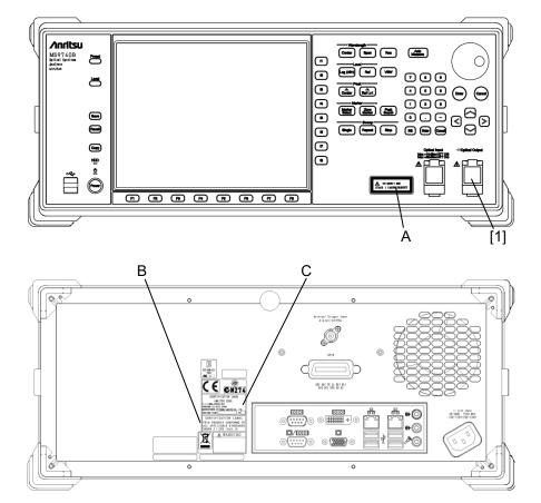
Figure 1 Locations of Laser Beam Apertures and Affixed Labels
