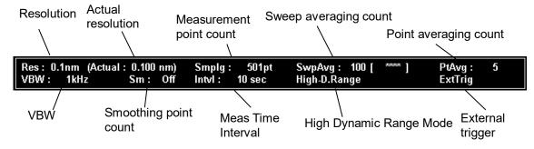
Figure 2.12-4 Measurement Condition Setting Display Field
