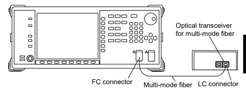
Figure 3.2-1 Connection Example of Optical Transceiver
