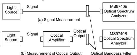
Figure 5.7.3-1 Optical Amplifier Measurement System
