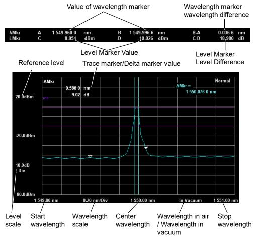
Figure 2.12-3 Marker, Level Scale, Wavelength Displays
