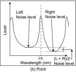
Figure 5.5.3-2 Detection Method for Noise Level
