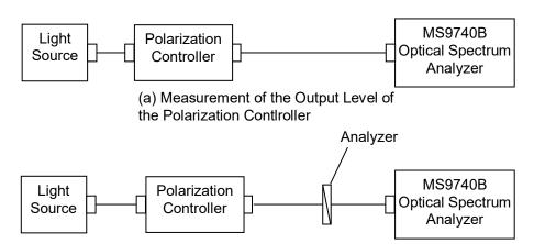
(b) Measurement of Analyzer Output Level
