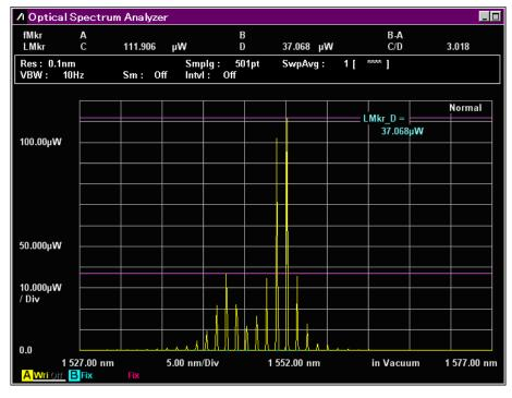
Figure 3.7.1-2 Level Marker Display
