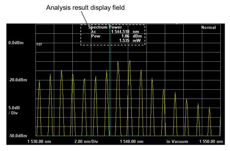
Figure 4.5.6-1 Spectrum Power Example
