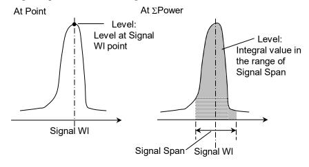
Figure 5.5.2-4 Measurement Method for Signal Level
