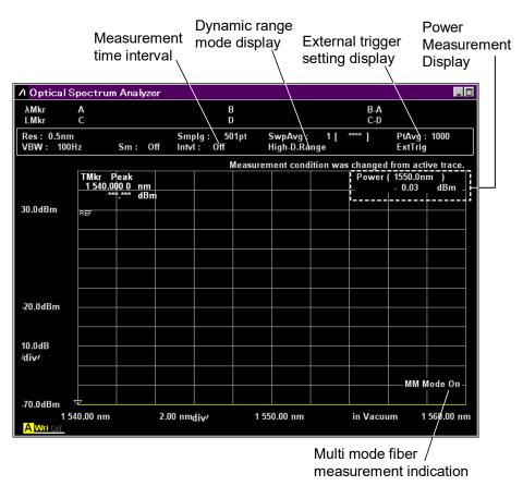
Figure 4.7-1 Measurement Settings Field and Power Measurement Display
