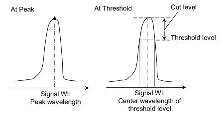
Figure 5.6.1-3 Measurement Method for Wavelength
