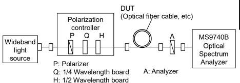
Figure 5.4.2-1 PMD Measurement System
