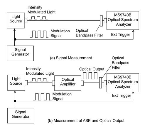
Figure 5.7.5-1 Pulse Method Measurement System
