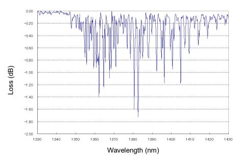
Figure 2.7-2 Water Vapor Absorption Spectrum
