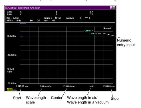
Figure 4.1-1 Names of Wavelength Display
