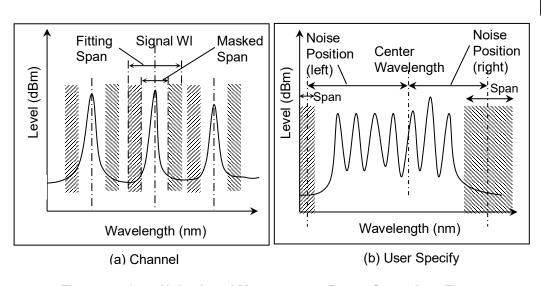
Figure 5.5.3-4 Noise Level Measurement Range Set at Area Type
