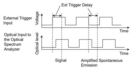
Figure 5.7.5-2 Definition of Ext Trigger Delay
