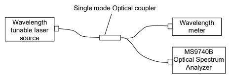
Figure 7.2.1-1 Wavelength Accuracy Test Setup
