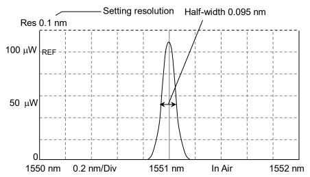
Figure 1.3-5 Measurement Example of Resolution 0.1 nm
