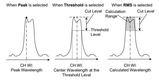
Figure 5.9.3-3 Measurement Method for Signal Wavelength
