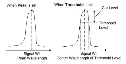
Figure 5.8.2-3 Signal Wavelength Measurement Method
