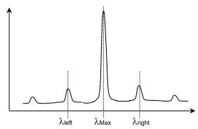
Figure 5.6.3-1 Position of Peak Wavelength and Side Modes
