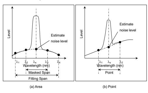
Figure 5.8.3-2 Detection Method for Estimated Noise Level
