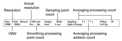
Figure 4.3-1 Measurement Condition Display Field
