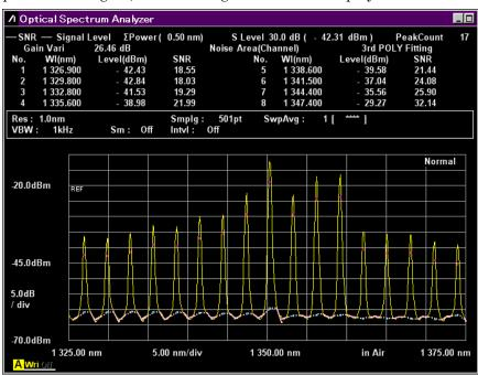
Figure 5.5.1-2 SNR Display Example
