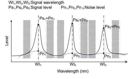
Figure 5.5.4-1 Fitting Curve and Noise Level When Area Type is Channel
