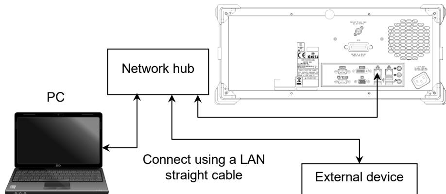
Figure 2.2.1-2 Sample Connection with Multiple External Devices
