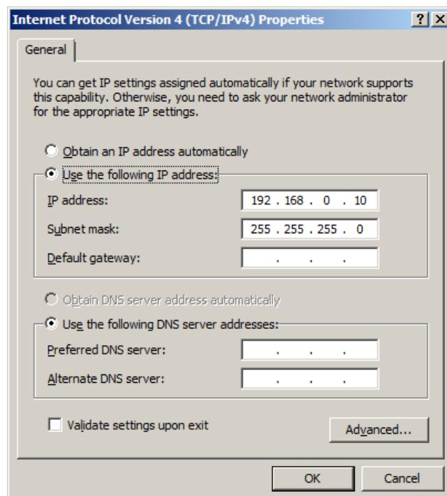
**Figure 2.3.1-6 Internet Protocol Version 4 (TCP/IPv4) Properties Dialog Box**
