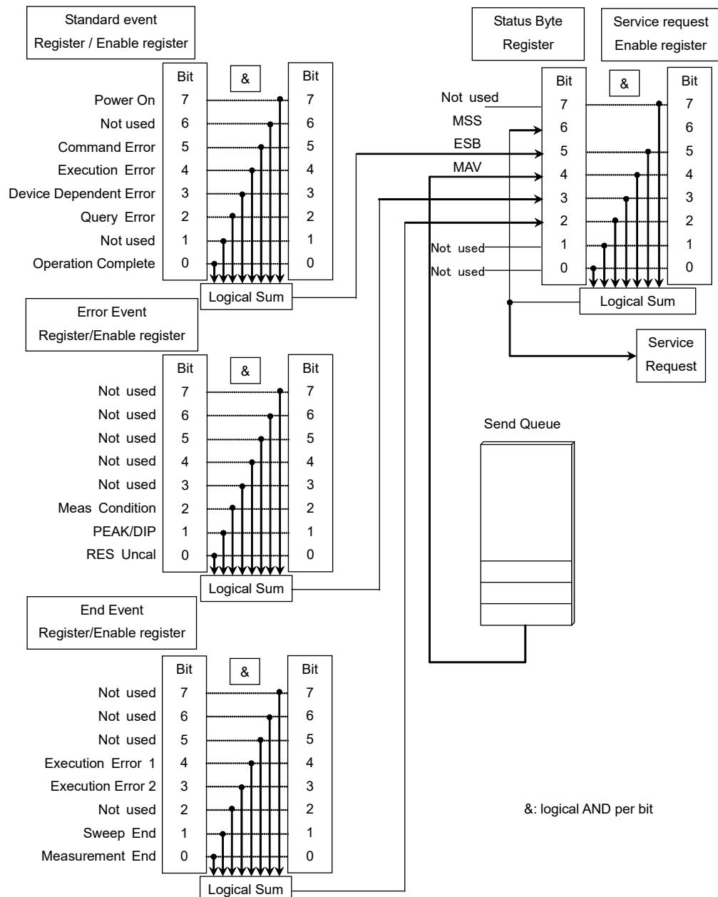
Figure 2.6.1-1 Register Structure
