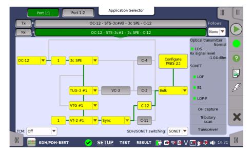
The manner of setting up the SONET interface of receiver is the same as that of transmitter. Refer to <u>SONET Frame Setup</u>.
