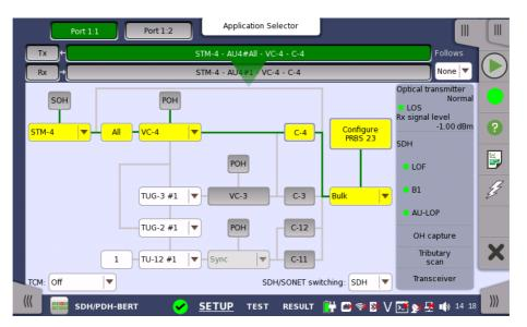
The general principle in setting up the SDH frame is to select the relevant values for the various containers in the multiplexing structure. This is done either via a drop-down menu or via a launched dialog box, by touching a drop-down menu or a button in the frame structure diagram.
