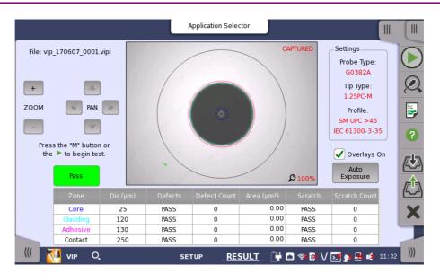
This screen displays the image captured by the Video Inspection Probe. Analyzing an image of the fiber edge surface is also available.
