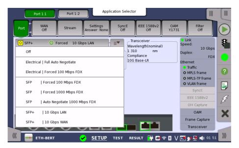
The quick setup menu contains a number of predefined port configurations (e.g. **Electrical | Forced 100 Mbps FDX**). The detailed mode dialog allows you to specify the configuration yourself.
