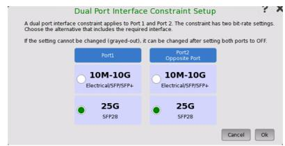
The Dual Port Interface Constraint Setup dialog box allows users to select a bit rate which can be used in the eCPRI/RoE BERT application.
