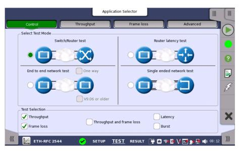
This screen allows you to specify your test mode and select which RFC 2544 tests to carry out.
