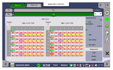
This screen provides information on the frame alignment when available. The frame alignment information includes the 16 first FAS/NFAS words of the CRC4 multiframe.
