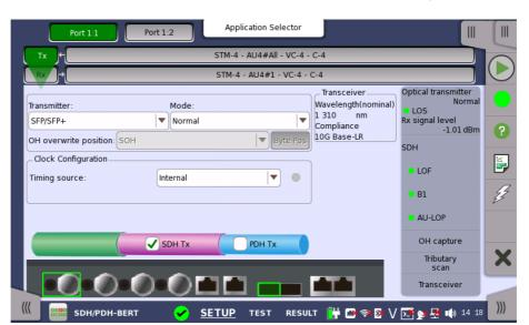
This screen allows you to enable the optical or electrical interface of the SDH transmitter. It can also be used to confirm the current status of the selected port.
