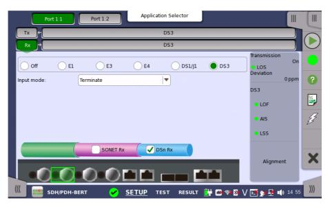
For the switching method between PDH Rx and DSn Rx, refer to <u>Physical Setup</u> in "E1 Setup and Status". Touch **DS3** radio button. Touching **Off** radio button disables the receiver. This screen allows you to make the physical setup of the PDH receiver in DS3 mode. It can also be used to inspect the current status of the selected port.
