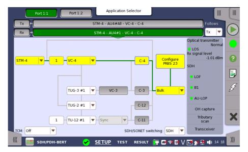
The manner of setting up the SDH interface of receiver is the same as that of transmitter. Refer to <u>SDH Frame Setup</u> in "Transmitter Setup".
