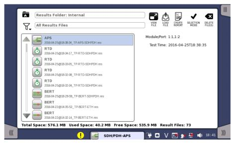
Creating a *workspace* for a previous test allows you to view the test results in the GUI and also to rerun the test if required (either with the same setup or with changed parameter settings). You are brought directly to the *Test Results* screen when you touch the **View/Load File** button, but can navigate to the other screens in the workspace from there.
