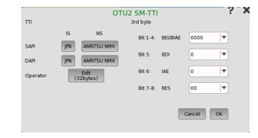
The TTI byte and 3rd byte can both be edited by launching the **OTUk SM-TTI** dialog box.
