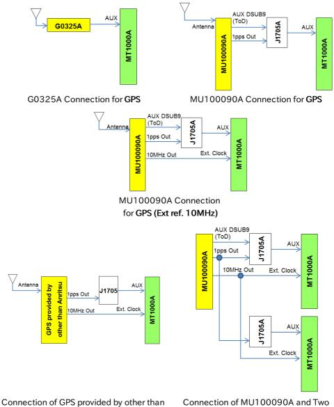
Connection of GPS provided by other than Anritsu for **1PPS(Ext ref. 10MHz)**  Connection of MU100090A and Two MT1000As for **1PPS(Ext ref. 10MHz)**
