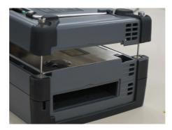
5. Tighten the four screws.
