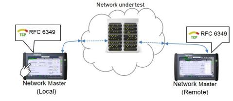
The required setup to perform RFC 6349 test is transferred from the 'local' Network Master to 'remote' Network Master when the test is started.
