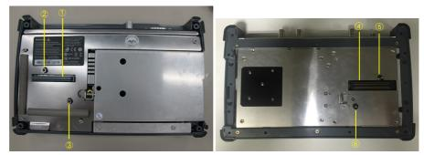
3. Remove four screws of the 10G Multirate module and replace to screws 2U in B0728A Rear Panel Kit.
