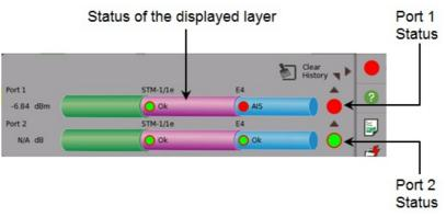
Port Status is the summary of all ports under test. If a failure occurs in any layer, Port Status turns into red.
