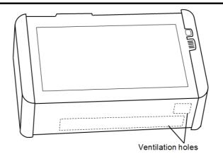
In this instrument, cooling air is taken in through the side panel, and hot air is exhausted through the bottom panel. When using MT1000A on a desk, open the <u>support stand</u> on the rear panel
