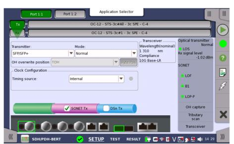
This screen allows you to enable the optical or electrical interface of the SONET transmitter. It can also be used to inspect the current status of the selected port.
