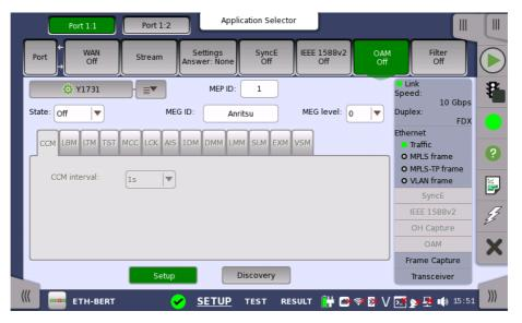
The screen contains two views: the default Setup view and the Discovery view. Use the **Setup** and **Discovery** buttons at the bottom of the screen to switch between the two views.
