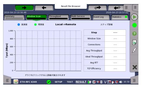
This screen presents the results from the Window Scan test. The ideal throughput and the actual throughput are shown in the chart. If touching on the Graph bars, step details appear in the right hand table.
