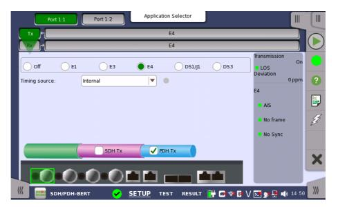
For the switching method between PDH Tx and DSn Tx, refer to <u>Physical Setup</u> in "E1 Setup and Status". Touch **E4** radio button. Touching **Off** radio button disables the transmitter.
