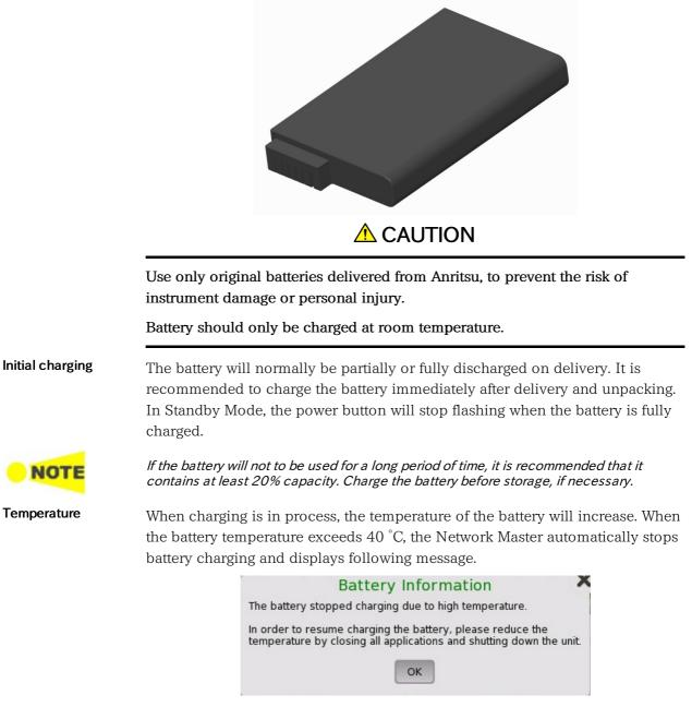
In order to resume battery charging as soon as possible, use the Network Master in the environment with lower ambient temperature. Or, close the application and shut down the Network Master.
