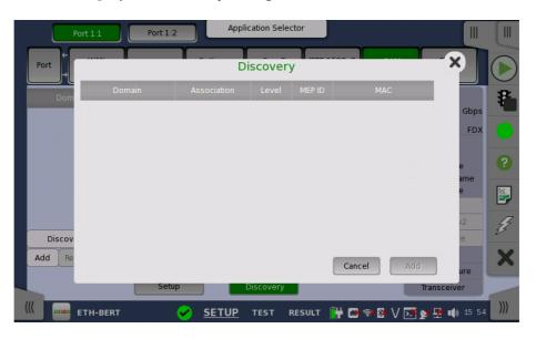
Devices will appear in the dialog's list as they are discovered. Select the device in the list and touch the **Add** button in the dialog box. The device is added to the list displayed on the Discovery view screen.
