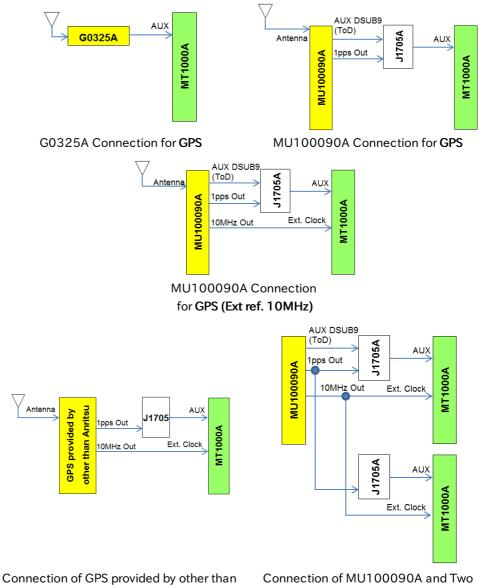
Connection of GPS provided by other thar Anritsu for **1PPS(Ext ref. 10MHz)**  Connection of MU100090A and Two MT1000As for **1PPS(Ext ref. 10MHz)**
