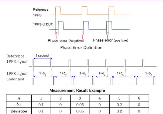
The difference between two BNC cable lengths makes time difference of 1PPS signals. Therefore it affects the phase error measurement result. You can set the correction of the time difference caused from the cable length difference at **1PPS cable correction** in the Control screen.
