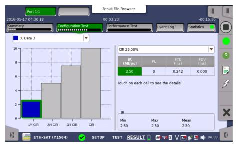
This screen presents the detailed Configuration Test results for a specific service. Use the drop-down menu at the top of the screen to select which service to view.
