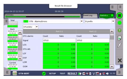
This screen presents a detailed analysis of the test results. You can choose to view either the current results (i.e. results measured during one second) or the total results from measurement start. You can also zoom in on a specific result item. The results can be displayed either in table (list) form or as a graph.
