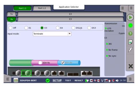
For the switching method between PDH Rx and DSn Rx, refer to <u>Physical Setup</u> in "E1 Setup and Status". Touch **E3** radio button. Touching **Off** radio button disables the receiver.
