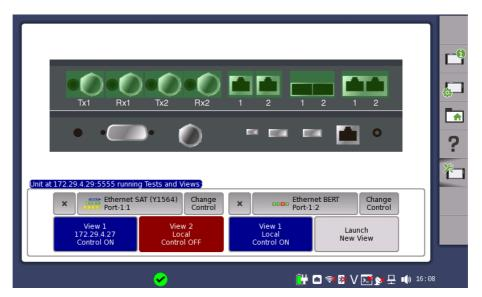
Each application is associated with up to two Views, Only one View can have control at a time. Having control gives user full access to all application functions, including modification of setting parameters, load and save functions, and running the test. Without control, users are only allowed to browse the current application settings and results.
