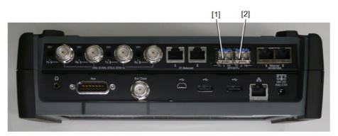
Figure 1: Locations of Laser Beam Aperture (MU100010A)
