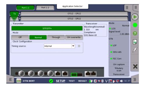
This screen allows you to enable the optical interface of the OTN transmitter. It can also be used to inspect the current status of the selected port by the button in Navigation area.
