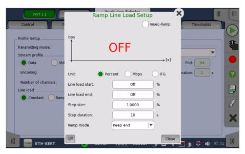
The line load unit can be specified from Percent, Mbps, and IFG.
