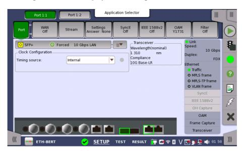
This screen allows you to specify the physical port configuration of the currently selected <u>Ethernet</u> port. It can also be used to inspect the current status of the selected port.
