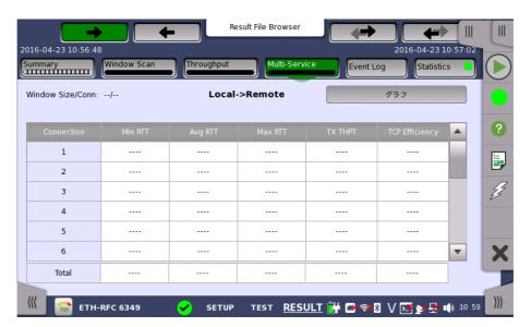
This screen presents results by each TCP connection of RTT, Throughput and TCP Efficiency. Use the **Graph** and **Table** buttons to switch between the tabular form and a graphical presentation of the results.
