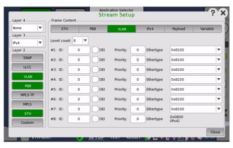
Virtual LAN (VLAN) is used to create independent logical networks within a physical network. When enabled, it adds a 16 bit IEEE 802.1Q field and a 16 bit Ethertype field to the header. The 802.1Q is separated into 3 parts.
