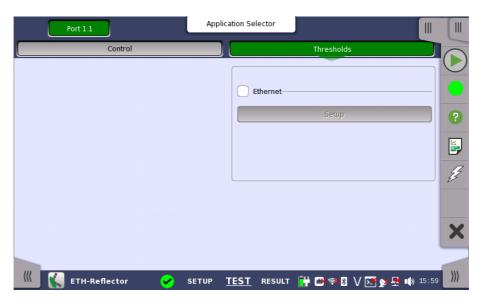
This screen allows you to set up a number of special monitoring items related to the various interface types. When specified and enabled, these threshold values (i.e. limits) for errors and Pass/Fail status will be used during the monitoring.
