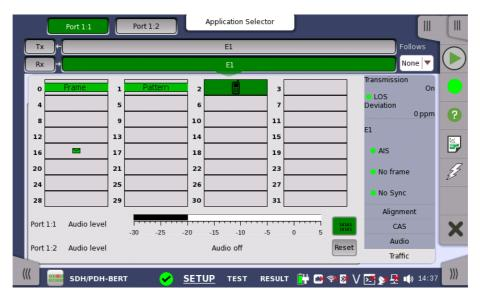
This screen shows the activity of the speech channels represented on the 2 Mbps line. You can switch between a traffic display and a view of the time slot content.
