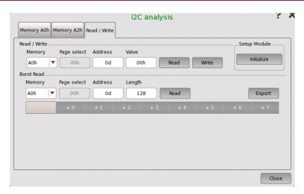
This dialog box allows reading/writing information into the registers of the optical transceiver via  $\rm I^2C$  (Inter-Integrated Circuit) interface.
