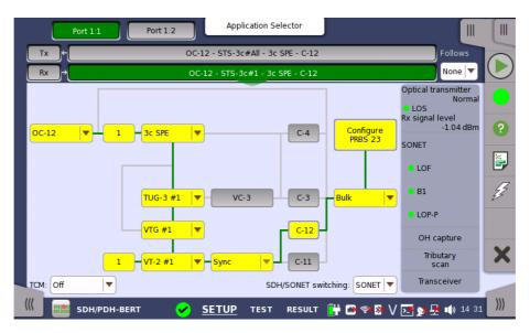
The manner of setting up the SONET interface of receiver is the same as that of transmitter. Refer to *SONET Frame Setup*.
