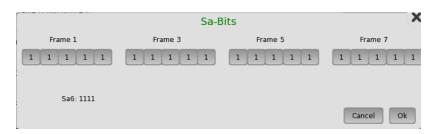
In the Sa-Bits dialog box, change the individual Sa-bits by touching on the relevant bit keys - this will toggle the bit key's binary value from logic 1 to 0 or vice versa. Touch Ok to accept the changes and close the dialog.
