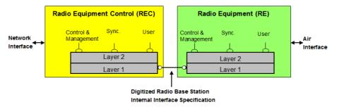
OBSAI (Open Base Station Architecture Initiative) defines the architecture of the cellular base station, including the interface between base band block and RF block. In the OBSAI specifications, this interface is defined as **RP3** (Reference Point 3).
