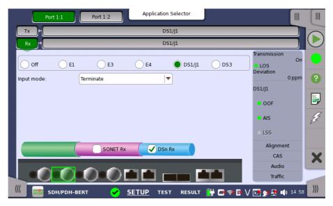
For the switching method between PDH Rx and DSn Rx, refer to <a href="Physical Setup">Physical Setup</a> in "E1 Setup and Status". Touch <a href="DS1/J1">DS1/J1</a> radio button. Touching <a href="Off">Off</a> radio button disables the receiver.
