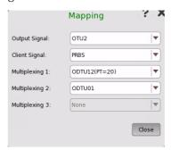
This dialog box allows you to define OTUk frame mapping.
