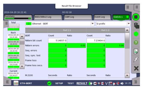
This screen presents a detailed analysis of the test results. You can choose to view either the total results from measurement start or the results of a specific interval during the test. You can also zoom in on a specific result item. The results can be displayed either in table (list) form or as a graph.
