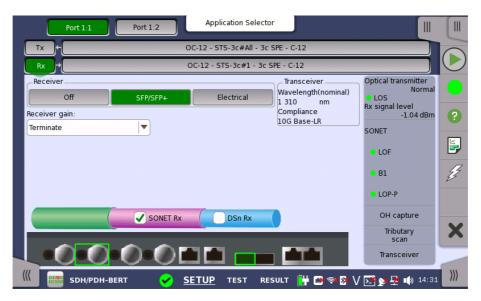
This screen allows you to make the physical setup of the receiver in SONET mode. It can also be used to inspect the current status of the selected port.
