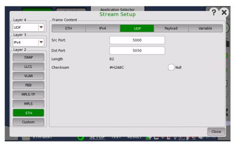
*User Datagram Protocol* is a core protocol of the Internet protocol suite. The UDP provides a minimal and simple interface between a network layer below and a session layer or application above. This protocol does not guarantee reliable and in-order delivery from sender to receiver.
