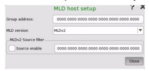
Touch the **Group address** box to set the multicast address of the group. (All the first eight bits are "1".)
