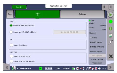
This screen is where you configure the traffic loop by specifying how addresses and/or ports are to be swapped and reflected.
