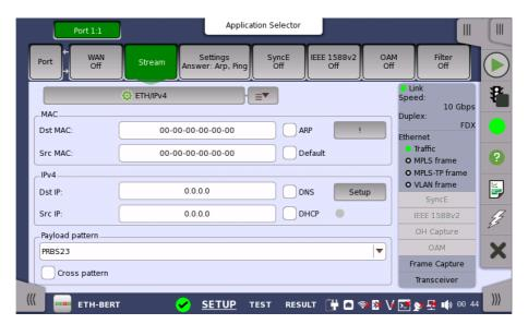
This screen contains the setup of the Ethernet frame content transmitted by the Network Master. The exact layout depends on the current selection of layers (i.e. the various encapsulation and protocol headers composing the Ethernet frame). Touching the button in the top left-hand part of the screen will display the dialog box to set options related to the layers.
