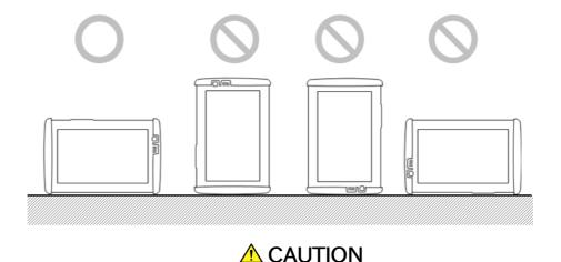
If the MT1000A is not installed in a "good" direction as above, a small shock may turn it over and harm the user.
