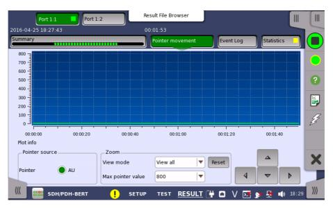
This screen presents a detailed analysis of pointer movements in the monitored signal. The results are displayed as a graph, showing the positions of a specific pointer over time.
