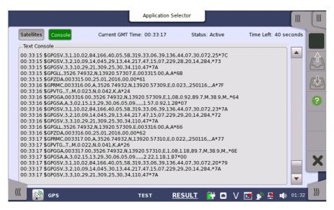
The log data format follows NMEA 0183 rev4.0 that is widely used in the GPS technology.
