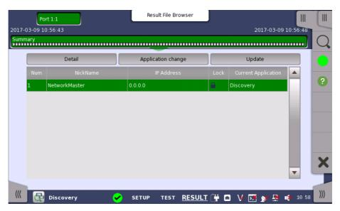
In this screen, up to 16 results of searching for Network Masters are displayed. If password is set to the Network Master, an icon appears in **Lock** row. Selecting a line by touching the table enables button operation.
