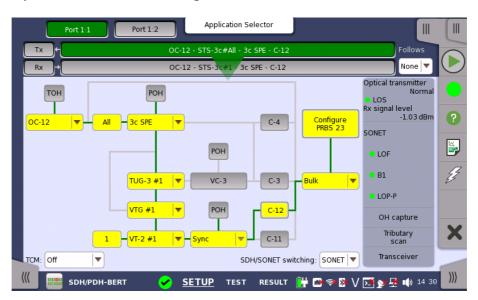
The general principle in setting up the SONET frame is to select the relevant values for the various containers in the multiplexing structure. This is done either via a drop-down menu or via a launched dialog box, by touching a drop-down menu or a button in the frame structure diagram.
