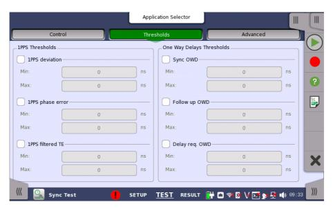
This screen contains the parameters for setting up the various threshold values (i.e. limits) for Pass/Fail status that are used during the monitoring. If measured results are out of the threshold, they will be marked in red on the
