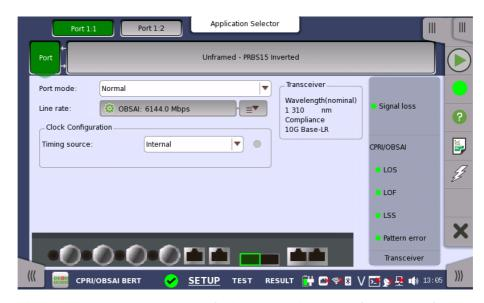
This screen allows you to specify the physical port configuration of the currently selected CPRI/OBSAI port. It can also be used to inspect the current status of the selected port.
