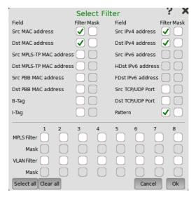
The filter editor dialog box contains a number of check boxes for enabling filters and masks on different addresses. Selectable check boxes depend on frame structure. The selected filters appear in row of the table.
