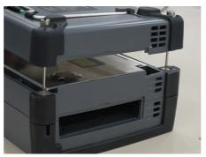
5. Tighten the four screws.
