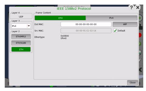
In the IEEE 1588v2 Protocol dialog box, the buttons on the left-hand side allow you to select the relevant layers. The current selection is shown at the top of the Frame Content area. Touching one of the layer buttons in the Frame Content area will display the setup parameters for that layer.
