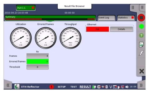
This screen contains a summary of the results of the Ethernet Reflector test. The information includes such things as number of errored frames and number of exceeded thresholds.
