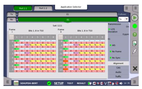
This screen provides information on the frame alignment when available. The frame alignment information includes the 16 first FAS/NFAS words of the CRC4 multiframe.
