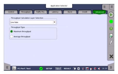
This screen sets the measurement method of *Measured Throughput* for the results of subsequent tests. The displays of the measurement results are not changed even of the Advanced settings are changed after completing the measurement.
