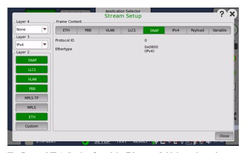
The  $Protocol\ ID$  is fixed to 0, and the Ethertype field depends on the upper protocol layer.
