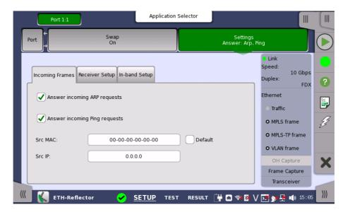
In **Src MAC** and **Src IP**, set the source MAC address and the source IP address of ARP request and Ping request.
