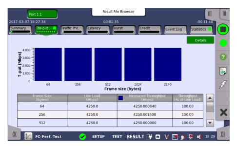
This screen displays the results of the Throughput test.
