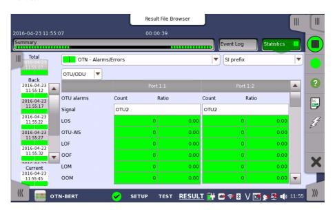
This screen presents a detailed analysis of the test results. You can choose to view either the current results (i.e. results measured during one second) or the total results from measurement start. You can also zoom in on a specific result item. The results can be displayed either in table (list) form or as a graph.
