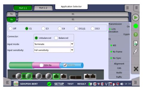
Switching between PDH Rx and DSn Rx is done in the SDH/SONET receiver setup screen.
