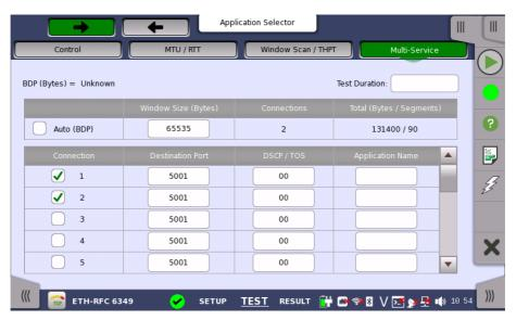
This screen allows you to set of connections by specifying TOS (Type of Service) or DSCP (differentiated Service Codepoint) used for Diffserv. Touch the **Test Duration** field to set the duration of Multi-service test.
