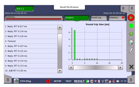
This screen presents the detailed results of an Ethernet Ping test. The results relate to a specific port and consist of the Round Trip Times of the individual Ping requests. The data is shown in both list-form and in a graphical representation.
