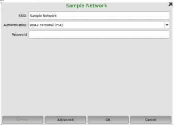
If backslashes (\) and double quotes (") are used in the SSID name, the **WLAN Setup** dialog box displays them with a backslash as  $\$  and  $\$  respectively when the Network Master connects to the network.
