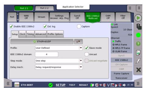
This screen allows you to configure the IEEE 1588 clock (based on the IEEE 1588 Precision Time Protocol (PTP), which is used to distribute absolute time across the Ethernet network). An IEEE 1588 clock can act either as a timing master or as a slave. The screen also contains information about the current status of the selected port.
