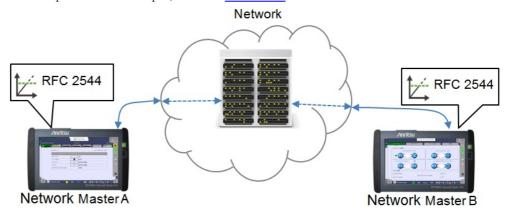
When the test mode is set to **Single ended network test** in the RFC 2544 application, test can be performed cooperating with opposed side reflecting equipment by switching Network Master B application to Reflector as shown in figure below.
