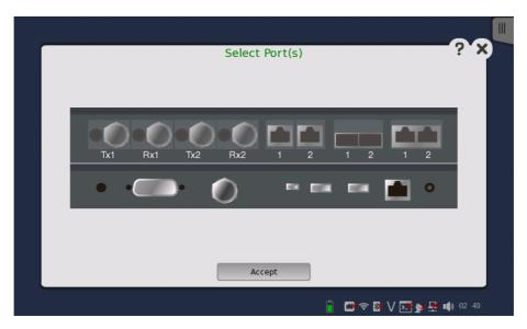
After the selection of resources, the Ports Setup screen is displayed, with the interface type(s) relevant for the selected application.
