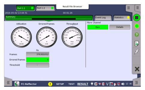
This screen contains a summary of the results of the FC Reflector test. The information includes such things as number of errored frames and number of exceeded thresholds.
