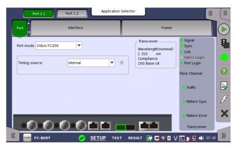
This screen allows you to specify the physical port configuration of the currently selected <u>Fibre Channel</u> port. It can also be used to inspect the current status of the selected port.
