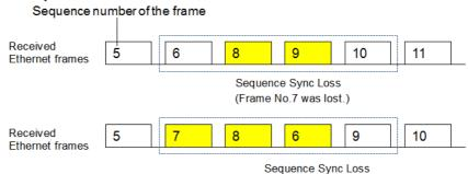
(Frame No.6 has delayed by two frames.)
