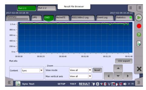
In this screen, the one way delay test results are displayed as a graph, showing the positions of a time error over time.
