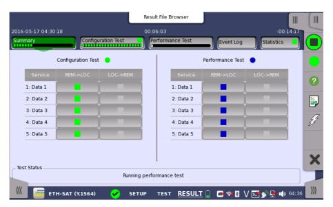
This screen presents a summary of the results of the Service Activation Test. Touching the result button for a specific service in either the **Configuration Test** or **Performance Test** result panel will display the relevant screen with detailed results information.
