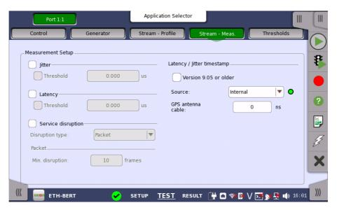
Select one or more of the measurements (Jitter, Latency and Service disruption) and then specify a threshold value for each. This screen allows you to configure Jitter, Latency and Service disruption.
