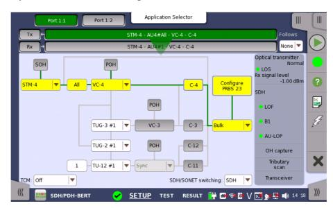
The general principle in setting up the SDH frame is to select the relevant values for the various containers in the multiplexing structure. This is done either via a drop-down menu or via a launched dialog box, by touching a drop-down menu or a button in the frame structure diagram.
