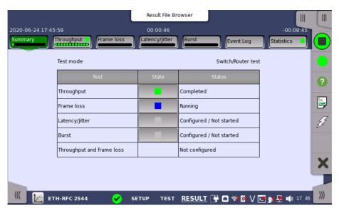
This screen presents the current status of the test(s) (Configured / Not Started, Running, Completed or Not Configured). Touching the status button for a specific test will display the result screen of the test.
