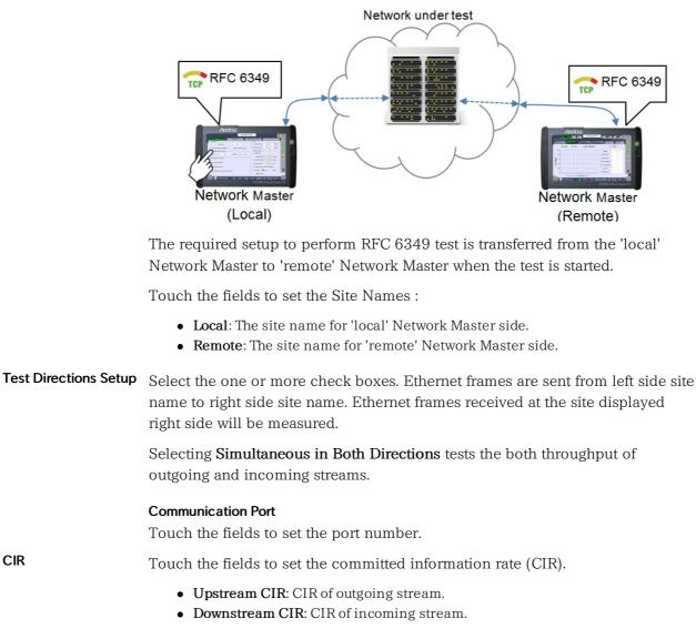
**Test Sequence** Select the check boxes of the test defined in RFC 6349, which you wish to run.
