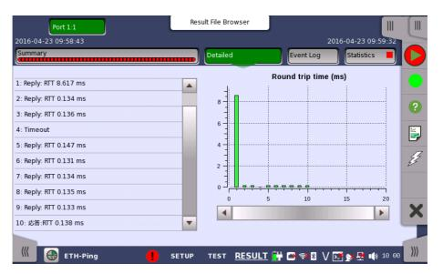
This screen presents the detailed results of an Ethernet Ping test. The results relate to a specific port and consist of the Round Trip Times of the individual Ping requests. The data is shown in both list-form and in a graphical representation.
