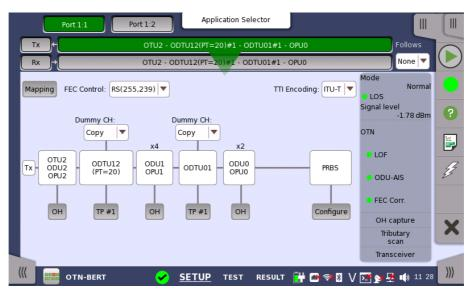
This screen allows you to configure OTUk frame of the currently selected transmitter. It can also be used to inspect the current status of the selected port in a separated screen.
