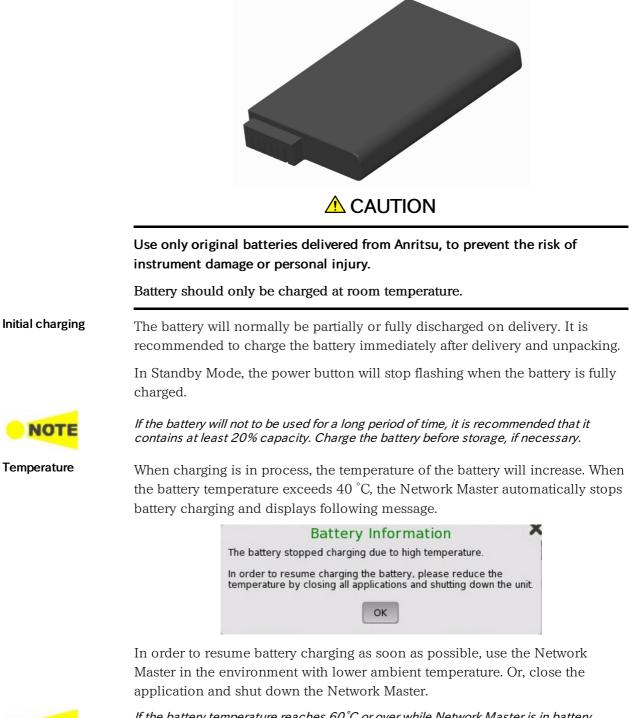
If the battery temperature reaches 60 °C or over while Network Master is in battery operation, Network Master shuts down automatically. In this case, leave the Network Master for approximately one hour to cool itself at room temperature (around 25 °C) before using Network Master again.
