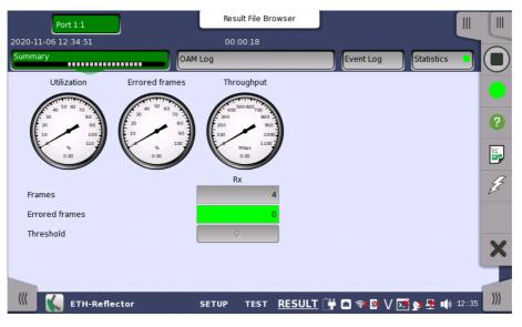
This screen contains a summary of the results of the Ethernet Reflector test. The information includes such things as number of errored frames and number of exceeded thresholds.
