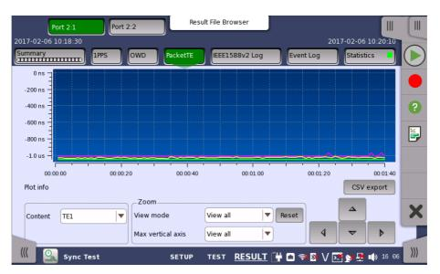
In this screen, the one way delay test results are displayed as a graph, showing the positions of a time error over time.
