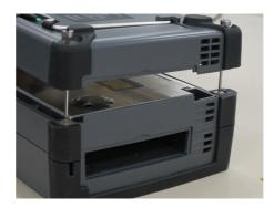
5. Tighten the four screws.
