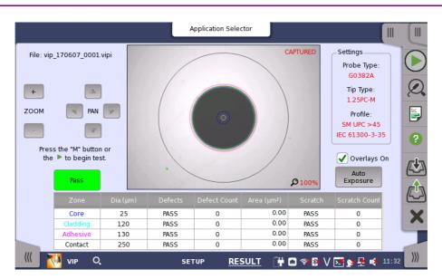
This screen displays the image captured by the Video Inspection Probe. Analyzing an image of the fiber edge surface is also available.
