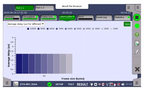
On the test-specific result screen, you switch between the two modes by using the **Graph** and **Table** buttons.
