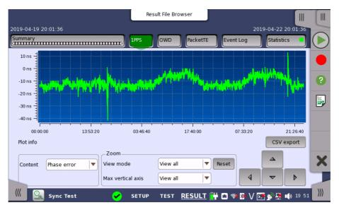
In this screen, the 1PPS test results are displayed as a graph, showing the positions of a time error over time.
