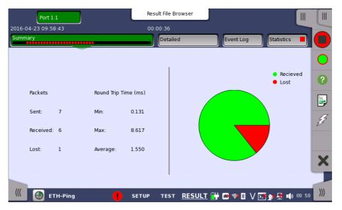
This screen presents a summary of the results of an Ethernet Ping test. The results relate to a specific port and consist of information about sent/received/lost packages and the minimum/maximum/average Round Trip Time.
