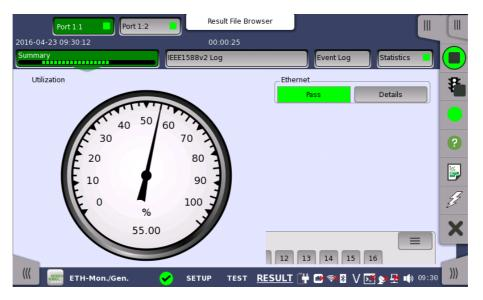
To view throughput information, select **Throughput** in the drop-down menu and then expand the dial. Use the drop-down menu above the expanded dial to select the relevant layer. When **Ethernet** is selected on Threshold of the Test Setup screen, the **Ethernet** information appears in the upper right-hand corner, shows pass/fail status summary. Touching the **Details** button allows you to inspect the individual pass/fail status.
