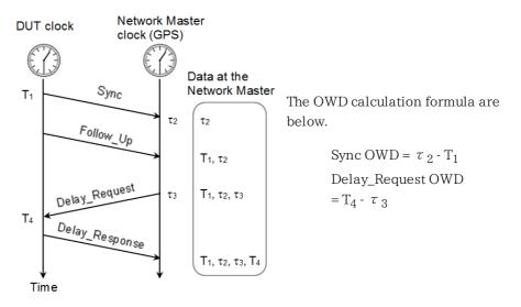
OWD contains the delay of the optical fiber cable between DUT and Network Master. To calculate Packet TE (TE1, TE4, Terr), TEs (Time error) that the cable delay is subtracted from OWD are defined as:
