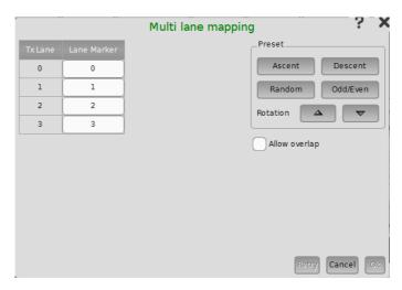
The number of lanes depends on the interface type. Touching Lane Marker field allows to set the PCS lane marker.
