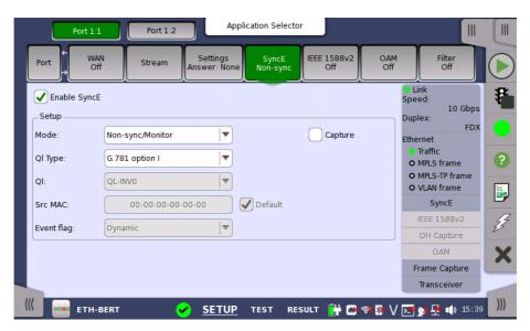
This screen allows you to configure the setup parameters related to Synchronous Ethernet. It can also be used to inspect the current status of the selected port.
