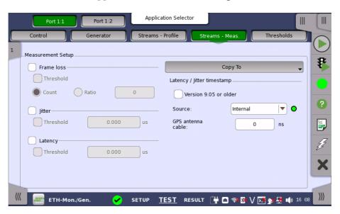
This screen allows you to configure Frame Loss, Jitter, and Latency.
