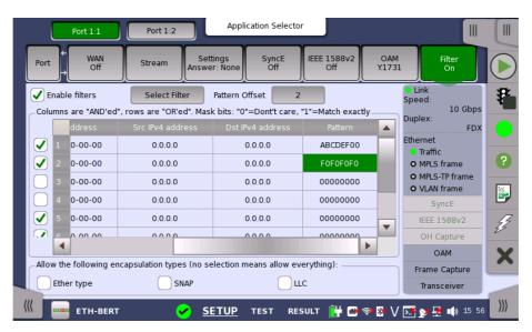
This screen allows you to set up filters and masks for the reception of Ethernet frames. It can also be used to inspect the current status of the selected port.
