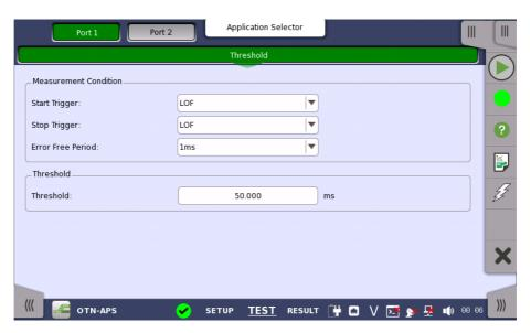
This screen contains the parameters for setting up the threshold values for errors and Pass/Fail status.
