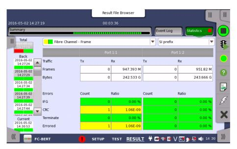
This screen presents a detailed analysis of the test results. You can choose to view either the results of a specific time interval or the total results from measurement start. The results can be displayed either in table (list) form or as graphs. You can also zoom in on a specific result item and display either a zoom or a histogram.
