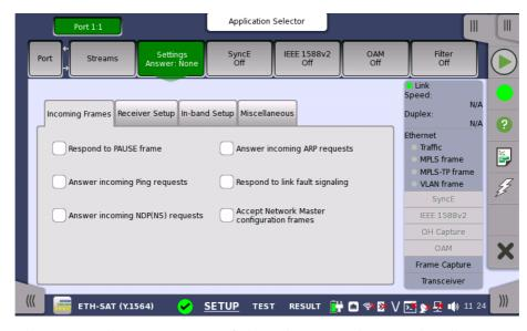
This screen allows you to specify how the Network Master handles incoming frames on the currently selected Ethernet port. It can also be used to inspect the current status of the selected port.
