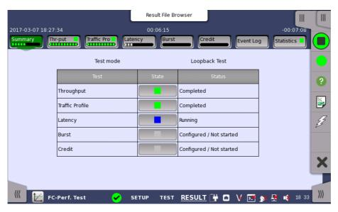
This screen presents the current status of the test(s) (**Configured / Not started**, **Running**, **Completed** or **Not Configured**). Touching the State button of the specific test displays the screen where the detailed result information is displayed.
