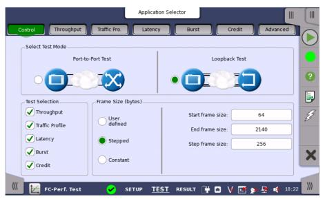
Specify the test mode and select the test to be performed in this screen.
