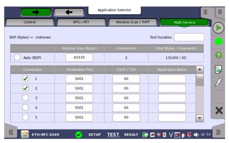
This screen allows you to set of connections by specifying TOS (Type of Service) or DSCP (differentiated Service Codepoint) used for Diffserv. Touch the **Test Duration** field to set the duration of Multi-service test.
