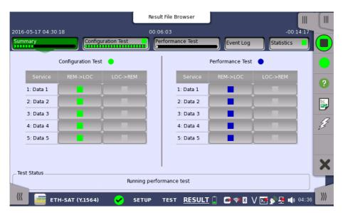
This screen presents a summary of the results of the Service Activation Test. Touching the result button for a specific service in either the **Configuration Test** or **Performance Test** result panel will display the relevant screen with detailed results information.
