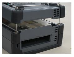
5. Tighten the four screws.
