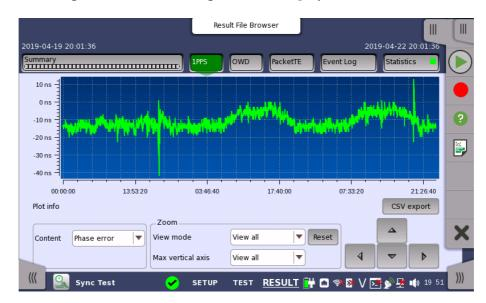
In this screen, the 1PPS test results are displayed as a graph, showing the positions of a time error over time.
