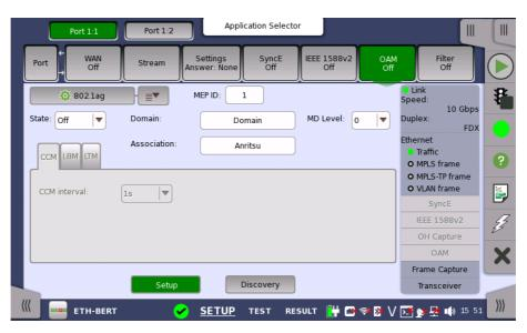
The screen contains two views: the default Setup view and the Discovery view. Use the **Setup** and **Discovery** buttons at the bottom of the screen to switch between the two views.
