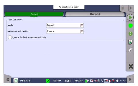
This screen allows you to configure the *RTD test* conditions for the currently selected port(s).
