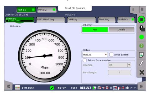
To view throughput information, select Throughput in the drop-down menu and then expand the dial. Use the drop-down menu above the expanded dial to select the relevant layer.
