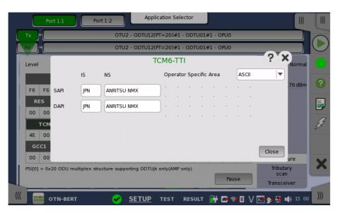
In the byte-specific dialog box, select the display format (ASCII or Hex) using the **Operator Specific Area** drop-down menu.
