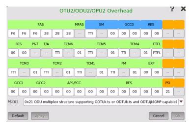
This dialog box presents detailed information about the overhead and allows you to configure it. Blue fields are OTU overhead. Green fields except FAS and MFAS are ODU overhead. Orange fields are OPU overhead.
