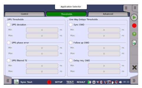
This screen contains the parameters for setting up the various threshold values (i.e. limits) for Pass/Fail status that are used during the monitoring.
