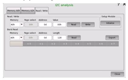
This dialog box allows reading/writing information into the registers of the optical transceiver via  $I^2C$  (Inter-Integrated Circuit) interface.
