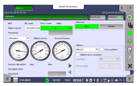
This screen contains a summary of the results of the Ethernet BERT test. The information includes such things as number of pattern errors, average and maximum disruption time, and number of exceeded thresholds.
