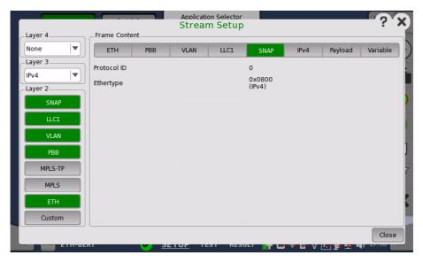
The **Protocol ID** is fixed to **0**, and the **Ethertype** field depends on the upper protocol layer.
