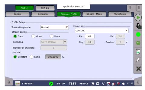
This screen contains the parameters for specifying a profile and pattern for each stream and for specifying which measurements are made.
