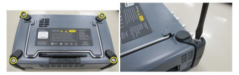
5. After loosing the four screws, lift up the 10G Multirate Module with holding both sides. If you cannot lift up, loosen the four screws again. You can see the panel as below.
