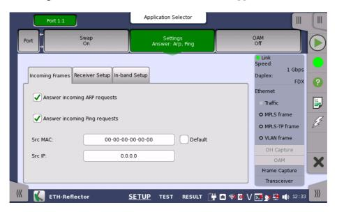
In Src MAC and Src IP, set the source MAC address and the source IP address of ARP request and Ping request.
