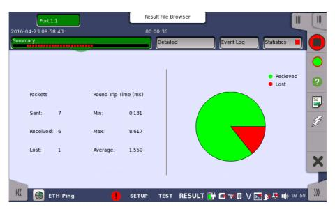
This screen presents a summary of the results of an Ethernet Ping test. The results relate to a specific port and consist of information about sent/received/lost packages and the minimum/maximum/average Round Trip Time.
