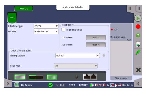
This screen allows you to specify the physical port configuration of the currently selected port. It can also be used to inspect the current status of the selected port.
