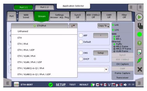
The quick selection menu contains a number of predefined frame configurations (e.g. ETH/VLAN/IPv4). The detailed mode dialog box allows you to specify the frame configuration yourself and also provides you with access to all configuration parameters available for the individual layers.
