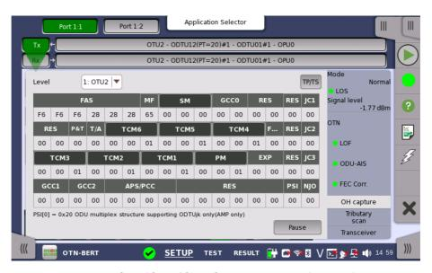
This screen shows OTU/ODU/OPU OH capture data for one frame at time. Use the **Level** drop-down menu to select which multiplexing level to display. For a description of the frame structure, see the <u>Overhead Dialog box</u> section under the ports setup of OTN.
