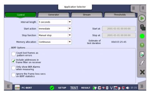
This screen contains the parameters that are generally required in a BERT test setup.
