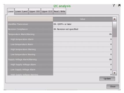
This dialog box allows reading/writing information into the registers of the optical transceiver via  $I^2C$  (Inter-Integrated Circuit) interface.
