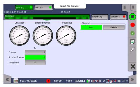
This screen contains a summary of the results of the Ethernet Pass Through test. The information includes such things as number of errored frames and number of exceeded thresholds.
