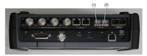
Figure 1: Locations of Laser Beam Aperture (MU100010A)
