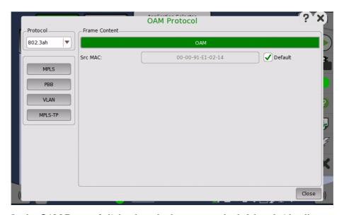
In the **OAM Protocol** dialog box the buttons on the left-hand side allow you to select the relevant layers. The current selection is shown at the top of the **Frame Content** area. Touching one of the layer buttons in the **Frame Content** area will display the setup parameters for that layer.
