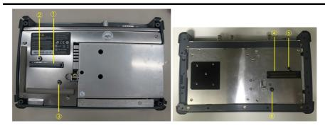
3. Remove four screws of the 10G Multirate module and replace to screws 2U in B0728A Rear Panel Kit.
