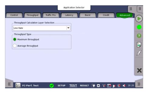
This screen sets the measurement method of *Measured Throughput* for the results of subsequent tests. The displays of the measurement results are not changed even of the Advanced settings are changed after completing the measurement.
