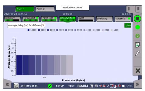
On the test-specific result screen, you switch between the two modes by using the **Graph** and **Table** buttons.
