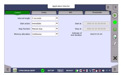
This screen contains the parameters that are generally required for BERT test.
