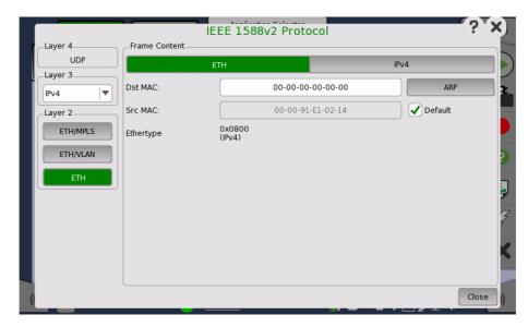
In the IEEE 1588v2 Protocol dialog box, the buttons on the left-hand side allow you to select the relevant layers. The current selection is shown at the top of the Frame Content area. Touching one of the layer buttons in the Frame Content area will display the setup parameters for that layer.
