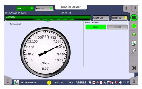
When Fibre Channel is selected on 'Threshold' of the Test Setup screen, the Fibre Channel information appears in the upper right-hand corner, shows pass/fail status summary. Touching the Details button allows you to inspect the individual pass/fail status.
