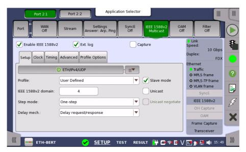
This screen allows you to configure the IEEE 1588 clock (based on the IEEE 1588 Precision Time Protocol (PTP), which is used to distribute absolute time across the Ethernet network). An IEEE 1588 clock can act either as a timing master or as a slave. The screen also contains information about the current status of the selected port.
