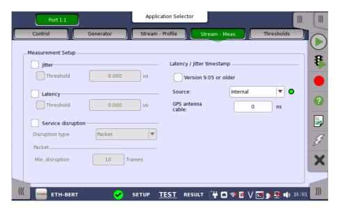
Select one or more of the measurements (Jitter, Latency and Service disruption) and then specify a threshold value for each. This screen allows you to configure Jitter, Latency and Service disruption.
