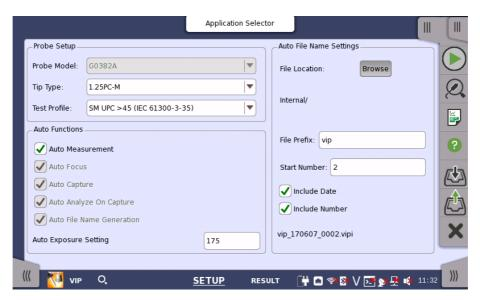
This screen allows you to configure the parameters related to a VIP test.
