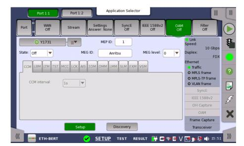
Y.1731 protocol setup Selecting the Y.1731 protocol will display the screen shown below.
