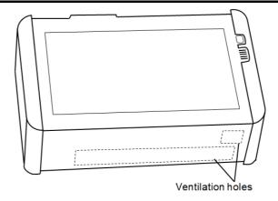
In the Network Master, cooling air is taken in through the side panel, and hot air is exhausted through the bottom panel. When using MT1000A on a desk, open the <u>support stand</u> on the rear panel
