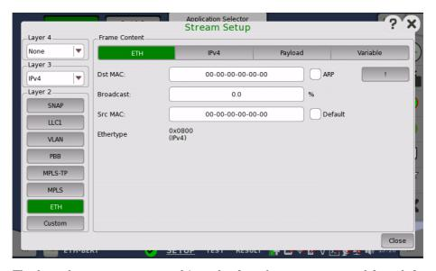
The layer buttons are arranged in order from bottom to top and from left to right. The TCP/UDP protocols are the uppermost layer and Ethernet the lowermost as depicted below compared to the OSI model.
