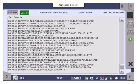
The log data format follows NMEA 0183 rev4.0 that is widely used in the GPS technology.
