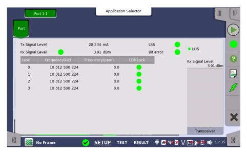
This screen presents detailed information about the current physical status of the received signal at the Device Test interface.
