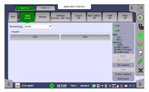
This screen allows you to specify the configuration of a WAN interface sublayer for the currently selected Ethernet port. It can also be used to inspect the current status of the selected port.
