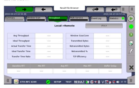
This screen presents the Throughput results in graph or table. Touch the **Graph** and **Table** buttons to switch between the tabular form and a graphical presentation of the results.
