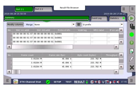
This screen presents the results of the Channel Statistics test. The screen contains two lists, one which lists the created channels and another which shows the results for each channel. Each channel is shown as a row in the two lists.
