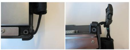
7. Remove the buckle cap from the handle and the carrying strap.
