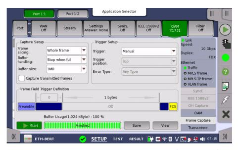
This screen allows you to set up and execute capture of transmitted frames.
