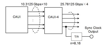
Block Diagram of MU100011A Tx Part (QSFP28, CFP4)
