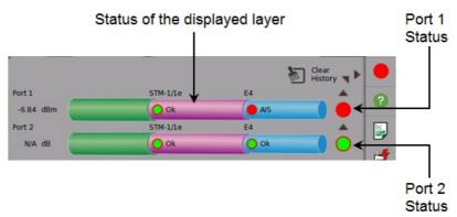
Port Status is the summary of all ports under test. If a failure occurs in any layer, Port Status turns into red.
