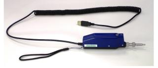
Connect the USB connector of the Video Inspection Probe to Network Master.
