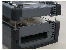
5. Tighten the four screws.
