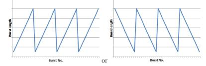
Touch the field of **Burst start** and **Burst end** to set the range that the burst length varies.
