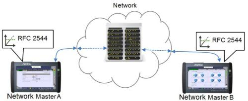
When the test mode is set to **Single ended network test** in the RFC 2544 application, test can be performed cooperating with opposed side reflecting equipment by switching Network Master B application to Reflector as shown in figure below.
