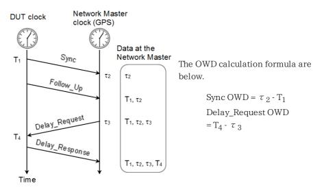
OWD contains the delay of the optical fiber cable between DUT and Network Master. To calculate Packet TE (TE1, TE4, Terr), TEs (Time error) that the cable delay is subtracted from OWD are defined as:
