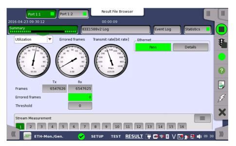
This screen contains a summary of the results of the Ethernet Monitor/Generate test. The information includes such things as number of errored frames and number of exceeded thresholds.
