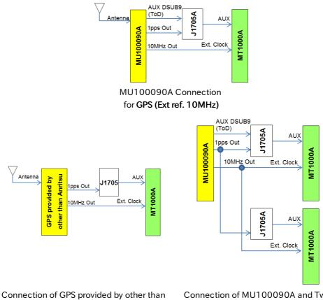
Connection of GPS provided by other thar Anritsu for **1PPS(Ext ref. 10MHz)**  Connection of MU100090A and Two MT1000As for **1PPS(Ext ref. 10MHz)**
