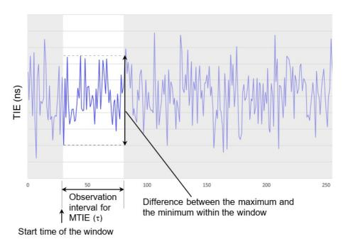
MTIE (Maximum time interval error) for observation interval  $\tau$  is the maximum of differences obtained for each window.
