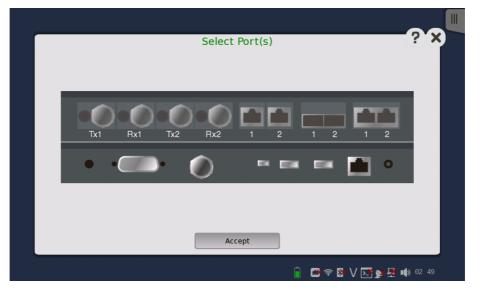
After the selection of resources, the *Ports Setup* screen is displayed, with the interface type(s) relevant for the selected application.
