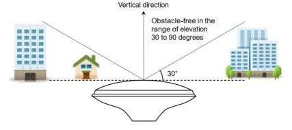
• Do not place the antenna near high-voltage cables, mobile-phone base stations, etc.
