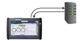
Fabric is the connection using fibre channel switch. Touch Fabric Login button to access to the fabric login server.
