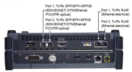
Port 1, Tx/Rx QSFP+/QSFP28 (SDH / SONET / OTN / Ethernet optical)
