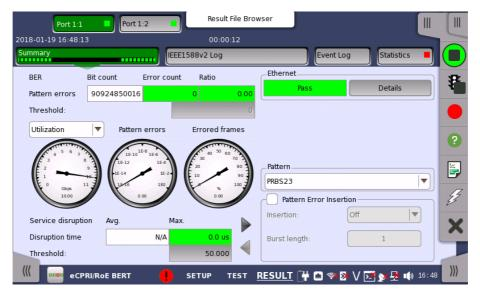
This screen contains a summary of the results of the eCPRI/RoE BERT test. The information includes such things as number of pattern errors, average and maximum disruption time, and number of exceeded thresholds.
