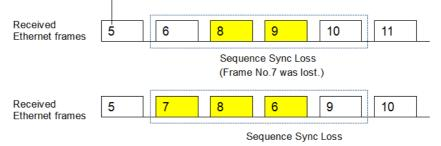
(Frame No.6 has delayed by two frames.)
