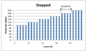
If the traffic duration is set to *Continuous* on the **Generator** screen, the step sequence will be repeated indefinitely. If traffic duration is set to *a number of seconds*, the step sequence will be terminated when the specified total period has elapsed. Similarly for traffic duration set to *a number of frames*, the step sequence will be terminated when the total number of transmitted frames reaches the specified count.
