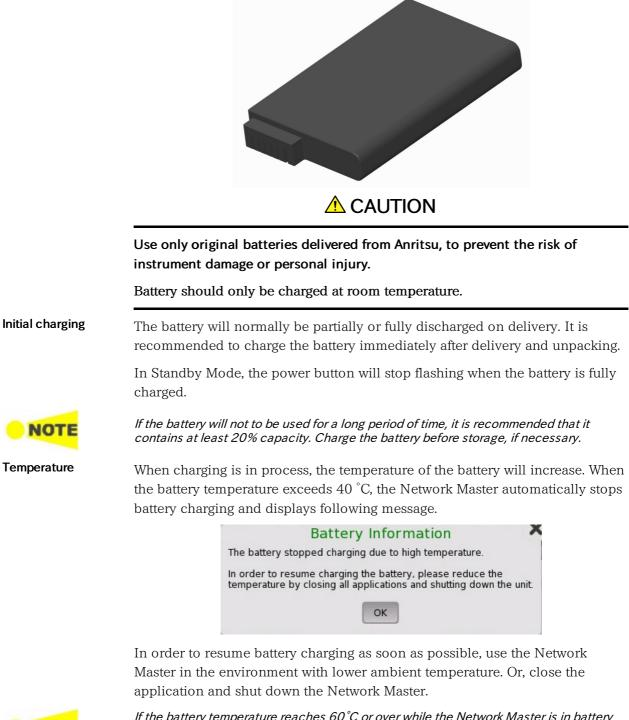
If the battery temperature reaches 60°C or over while the Network Master is in battery operation, the Network Master shuts down automatically. In this case, leave the Network Master for approximately one hour to cool itself at room temperature (around 25°C) before using the Network Master again.
