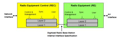
OBSAI (Open Base Station Architecture Initiative) defines the architecture of the cellular base station, including the interface between base band block and RF block. In the OBSAI specifications, this interface is defined as **RP3** (Reference Point 3).
