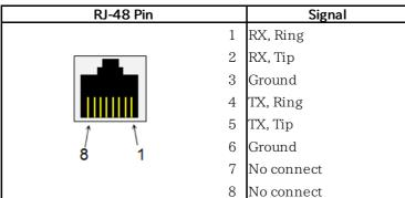
Be sure to confirm the cable type. For E1 cable, there are the straight cable and the cross cable.
