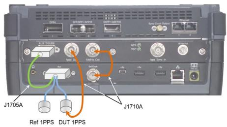
4. Turn MU100090B Power **On**, and set Sync mode to **GPS/GNSS**. Set 0 to **REF 1PPS Correction**.
