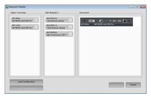
3. Set configuration of the Network Master by clicking options in **Select Controller**, and **Add Module(s)**.
