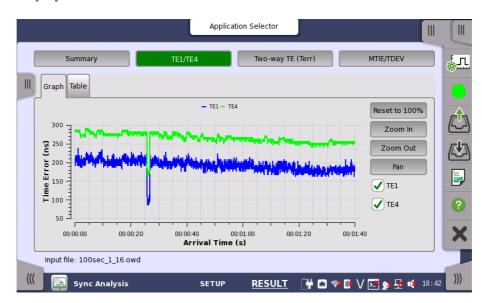
On this screen, you can view the graph and table of time errors, and Pass/Fail results.
