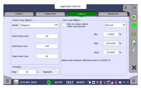
This screen allows you to configure the parameters related to an RFC 2544 Latency/Jitter test:
