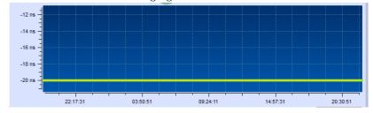
8. Set REF 1PPS Correction value so that 1PPS measurement result will be -1 ns, because BNC cable length is 0.2 m. In this case, set -19.
