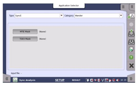
This screen allows you to configure the parameters related to a time error analysis.
