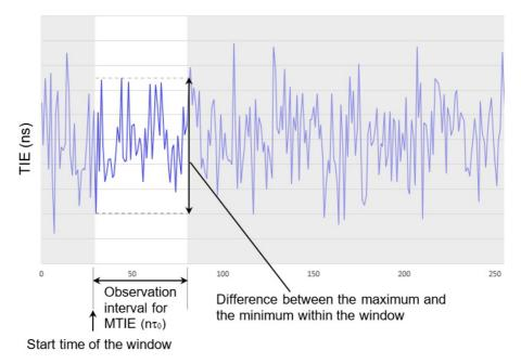
MTIE (Maximum time interval error) for observation interval n  $\tau_0$  is the maximum of differences obtained for each window.
