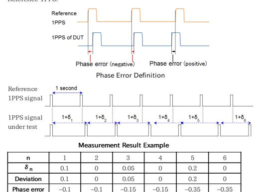
The difference between two BNC cable lengths makes time difference of 1PPS signals. Therefore it affects the phase error measurement result. You can set the correction of the time difference caused from the cable length difference at 1PPS cable correction in the Control screen.
