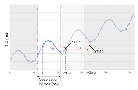
By calculating dTIE1 and dTIE2 for all the samples in the window, the variance of the clock frequency difference can be obtained. Find the variance of the frequency difference of each window while changing the window start time, and take the average of the average to obtain the TDEV.
