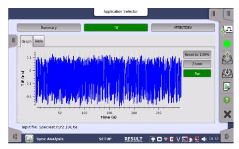
This screen presents the graph and the table of time interval errors, and Pass/Fail results.
