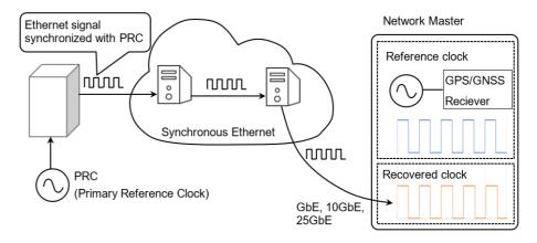
The time it takes for an Ethernet signal to reach the receiver over the network is not constant, so the frequency of the recovered clock will change slightly. This is the cause of wander.
