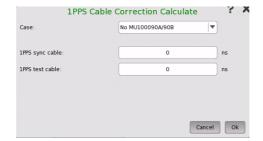
The measured phase error includes the phase error of **Reference 1PPS input** and **1PPS input under test**, as well as the phase error caused by the difference in the lengths of the two connected 1PPS cables.
