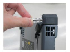
4. Attach the 10G Multirate module to the MU100090A. Place the 10G Multirate module on the MU100090A so as to connect the following pairs: 7 - 10, 8 - 11, 9 - 12.
