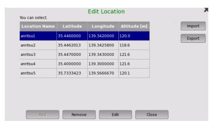
**Add**: Adds the location of fixed position while receiving GNSS signal. Up to 32 positions can be added.
