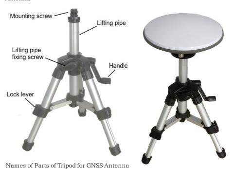
The tripod legs can be extended by opening the lock levers.
