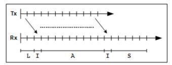
The Tx graph shows the transmitted periods, and the Rx graph shows the received periods. Due to latency the receiver will first see the transmitted frames some time later than when transmitter actually sent the frames (the L-period). This is also why the receiver may have more periods than the transmitter, in order to await delayed frames. However the receiver will maximum wait for 10 extra periods (seconds) before it times out, as frames may actually physically be lost somewhere in the network.
