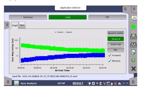
This screen presents the graph and the table of one way delays, and Pass/Fail results.
