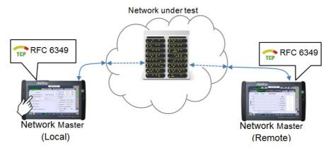
The required setup to perform RFC 6349 test is transferred from the 'local' Network Master to 'remote' Network Master when the test is started.
