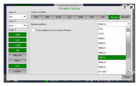
Open the **Payload pattern** drop-down menu to select the relevant pattern.
