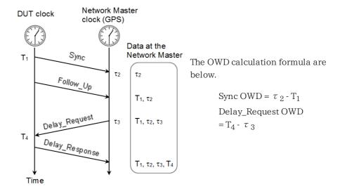
OWD contains the delay of the optical fiber cable between DUT and Network Master. To calculate Packet TE (TE1, TE4, Terr), TEs (Time error) that the cable delay is subtracted from OWD are defined as:
