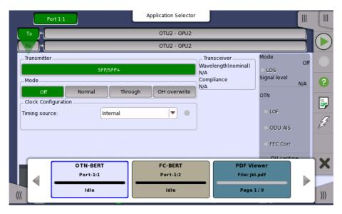
The running applications appear in the Applications Switcher. Touching the button switches the application on the screen.
