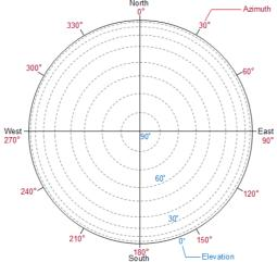
Radius of the circle corresponds to the elevation. The position at circle edge is where the elevation is 0 degree.
