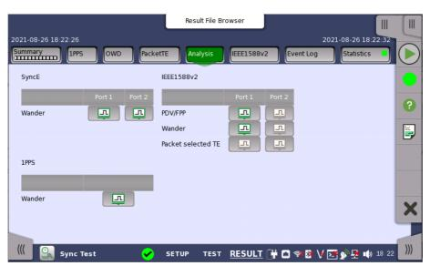
This screen presents the measurement status of 1PPS, SyncE, and IEEE1588v2. This screen also allows you to analyze the acquired data by starting the Sync Analysis application.
