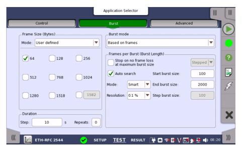
This screen allows you to configure the following parameters related to an RFC 2544 Burst test:
