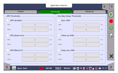
This screen contains the parameters for setting up the various threshold values (i.e. limits) for Pass/Fail status that are used during the monitoring.
