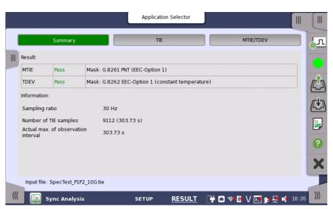
The analysis parameters are displayed on the slide panel left-hand of the screen.
