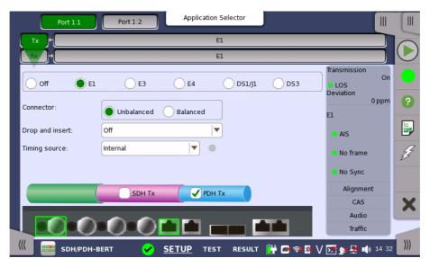
Switching between PDH Tx and DSn Tx is done in the SDH/SONET transmitter setup screen.
