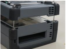
5. Tighten the four screws.
