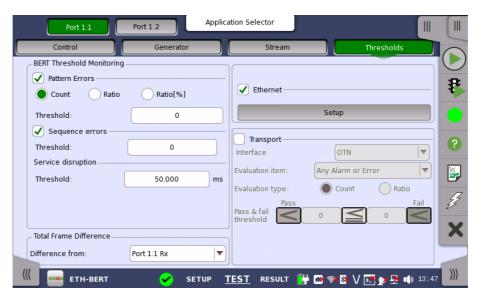
In addition to the various parameters, the **Test Setup** screen also contains the <u>Application toolbar</u> and the navigation tabs for horizontal and vertical navigation.
