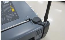
5. After loosing the four screws, lift up the 10G Multirate Module with holding both sides. If you cannot lift up, loosen the four screws again. You can see the panel as below.
