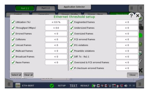
In the dialog box, select the check boxes for the relevant thresholds and then touch the **Close** button to list them on the **Thresholds** screen. You can select/deselect all check boxes in the dialog box by using the **Select all** / **Clear all** buttons. Touch the individual value fields either in the dialog box or in the list on the screen to specify the threshold values.
