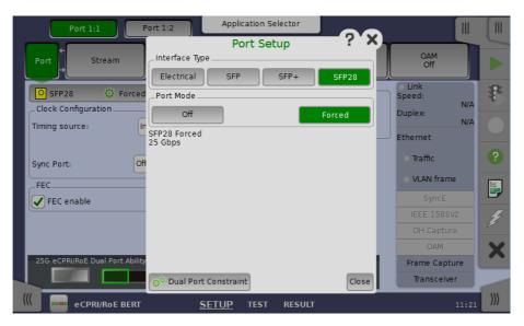
Touching Dual Port Constraint displays the Dual Port Interface Constraint Setup dialog box.
