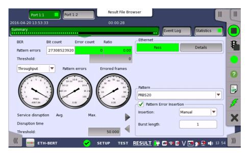
During a measurement, Measurement start time, Elapsed time, and Remaining time of measurement are displayed in Navigation area. Remaining time of measurement is not displayed if Stop function is set to **Manual stop** in Control screen.
