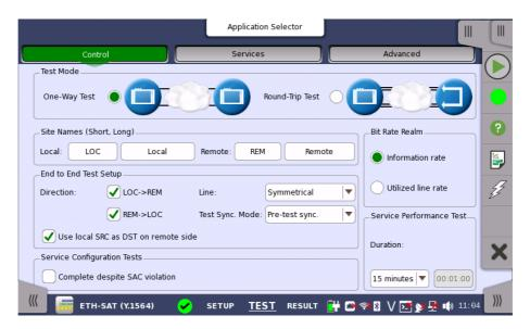
This screen allows you to configure the test mode and other general parameters related to a <u>Service Activation Test</u>.
