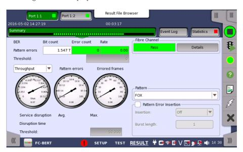
This screen contains a summary of the results of the Fibre Channel BERT test. The information includes such things as number of pattern errors, average and maximum disruption time, and number of exceeded thresholds.
