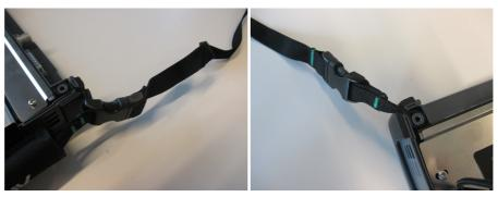
9. Attach the Network Master and MU100010A, insert the battery pack and mount the battery lid with the reverse sequence at the beginning.
