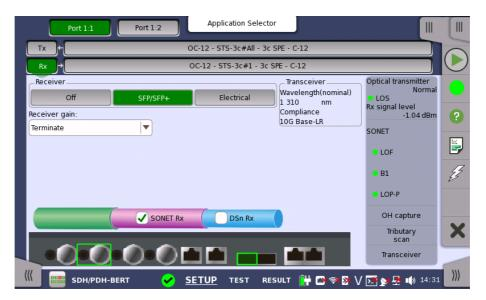
This screen allows you to make the physical setup of the receiver in SONET mode. It can also be used to inspect the current status of the selected port.
