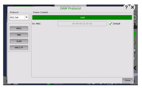
In the **OAM Protocol** dialog box the buttons on the left-hand side allow you to select the relevant layers. The current selection is shown at the top of the **Frame Content** area. Touching one of the layer buttons in the **Frame Content** area will display the setup parameters for that layer.
