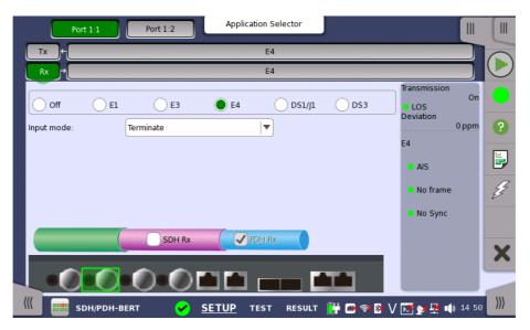
For the switching method between PDH Rx and DSn Rx, refer to <u>Physical Setup</u> in "E1 Setup and Status". Touch **E4** radio button. Touching **Off** radio button disables the receiver.
