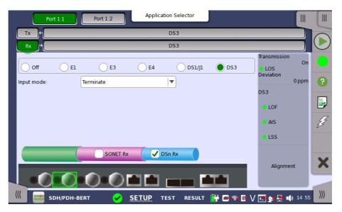
For the switching method between PDH Rx and DSn Rx, refer to <u>Physical Setup</u> in "E1 Setup and Status". Touch **DS3** radio button. Touching **Off** radio button disables the receiver.
