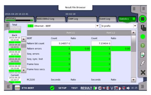
This screen presents a detailed analysis of the test results. You can choose to view either the total results from measurement start or the results of a specific interval during the test. You can also zoom in on a specific result item. The results can be displayed either in table (list) form or as a graph.
