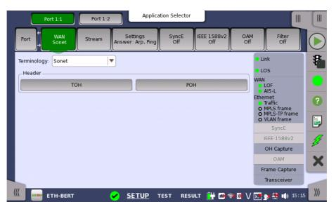
This screen allows you to specify the configuration of a WAN interface sublayer for the currently selected Ethernet port. It can also be used to inspect the current status of the selected port.
