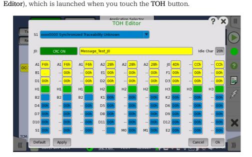
The setup principle is the same in this editor dialog box as in the SONET structure. Touching a button or opening a drop-down menu will open for new editor dialog boxes, new value selections etc.
