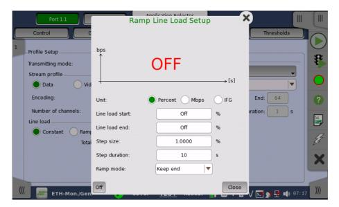
The line load unit can be specified from **Percent**, and **Mbps**. Touching **Off** at left-bottom stops sending the stream.
