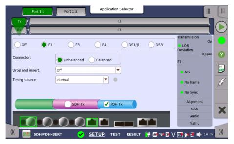
Switching between PDH Tx and DSn Tx is done in the SDH/SONET transmitter setup screen.
