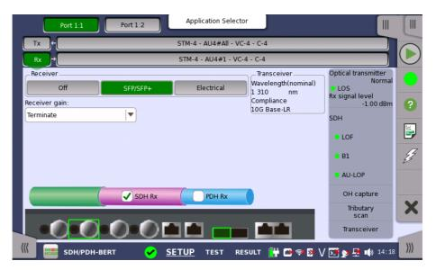
This screen allows you to make the physical setup of the receiver in SDH mode. It can also be used to confirm the current status of the selected port.
