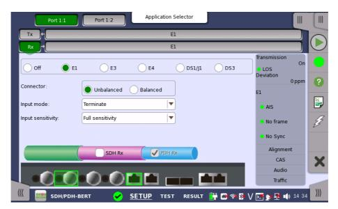
Switching between PDH Rx and DSn Rx is done in the SDH/SONET receiver setup screen.
