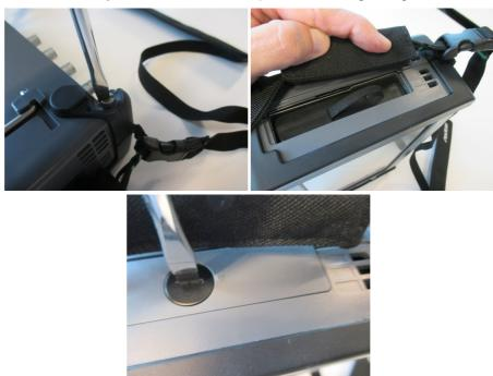
9. Attach the Network Master and MU100010A, insert the battery pack and mount the battery lid with the reverse sequence at the beginning.
