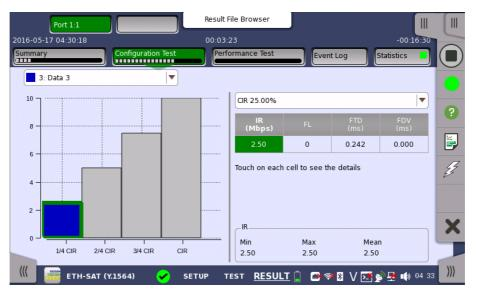
This screen presents the detailed Configuration Test results for a specific service. Use the drop-down menu at the top of the screen to select which service to view.
