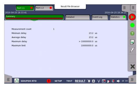
This screen presents a summary of the RTD test results, for all of the ports included in the test. For each port, the information consists of:
