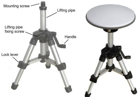
Names of Parts of Tripod for GNSS Antenna
