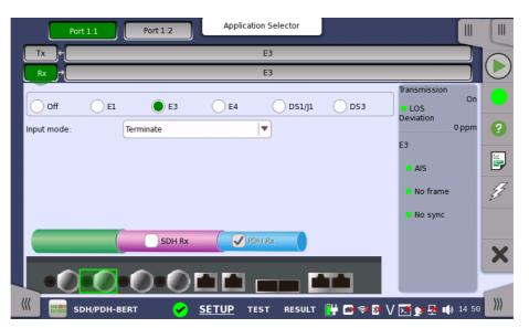
For the switching method between PDH Rx and DSn Rx, refer to <u>Physical Setup</u> in "E1 Setup and Status". Touch **E3** radio button. Touching **Off** radio button disables the receiver.
