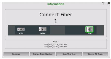
In the upper frame, the fiber number is displayed under **Connect Fiber** and the connecting connector on OTDR module is indicated. In the lower frame, file names which will be stored are displayed.
