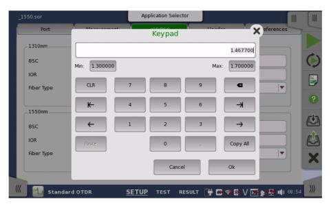
In general, a keypad consists of the character/number keys, a display field showing the current text/number entry, various editing-related keys. For number entries, the minimum and maximum values allowed are also shown. When you launch a keypad from a field, the current field value is shown in the keypad's display field.
