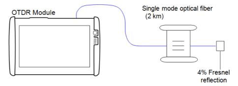
When testing the distance measurement accuracy of 850 nm and 1300 nm, change the optical fiber in Connection diagram to the multi-mode fiber (2 km).
