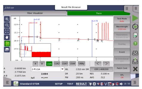
The LSA 2-Point Loss is the change in dB (Y-Axis) calculated between the two points. When the Cursor A, Y-Axis position is greater than the Cursor B, Y-Axis position, a positive loss measurement is displayed.
