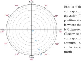
Radius of the circle corresponds to the elevation. The position at circle edge is where the elevation Clockwise angle corresponds to the azimuth. Top of the circle corresponds to
