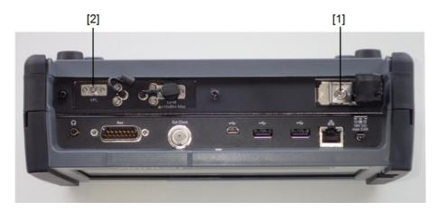
Figure 1: Locations of laser aperture (MU100020A)
