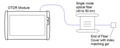
When testing the dynamic range of 850~nm and 1300~nm, change the optical fiber in Connection diagram to the multi-mode fiber (20 to 25~km).
