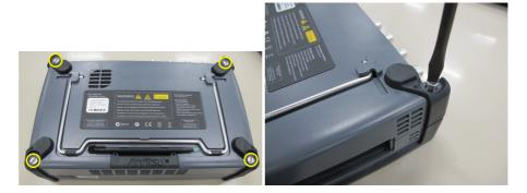
5. After loosing the four screws, lift up the 10G Multirate Module with holding both sides. If you cannot lift up, loosen the four screws again. You can see the panel as below.
