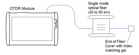
When testing the linearity of 850 nm, change the optical fiber in Connection diagram to the multi-mode fiber (20 to 25 km).
