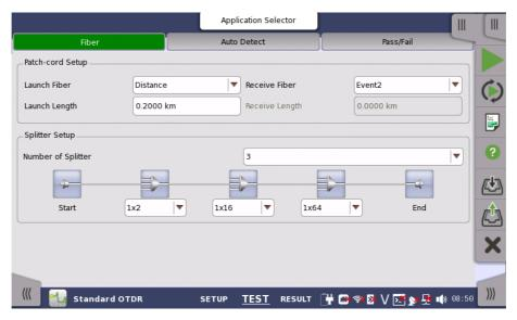
In addition to the various parameters, the **Test** screen also contains the <u>Application toolbar</u> and the navigation tabs for horizontal and vertical navigation.
