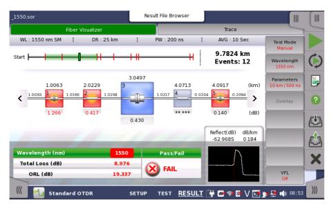
In addition to the results, whose presentation varies from application to application, the **Test results** screen also contains soft keys in right-hand. To save results to a file, touch on the Application toolbar.
