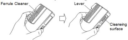
2. Hold the lever in the opened position, press the optical connector ferrule end into the cleaning surface, and then rub in one direction as shown in the following figure.
