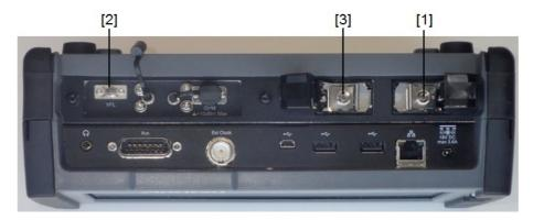
Figure 2: Locations of laser aperture (MU100021A)
