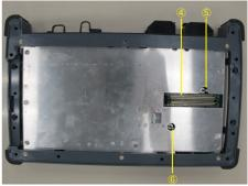
$3. \,$  Insert screws 1U in B0728A Rear Panel Kit to four corners of the rear panel.
