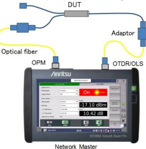
Loss is displayed as the differential between the reference and the measured power.
