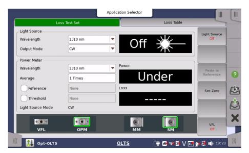
This screen allows you to control the light source and the power meter.
