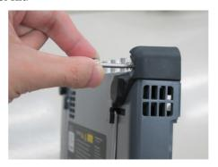
4. Attach 10G Multirate module to OTDR module. Place 10G Multirate module on the OTDR modules as to connect following pairs: 7 - 10, 8 - 11, 9 - 12. Be careful not to bump the guide pins (8, 9, 11 and 12) to the connectors (7 and 10).
