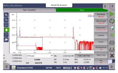
In the Trace screen, the fiber loss versus distance is shown in graphical. The following icons appear on the traces.
