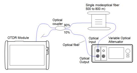
When testing the dead zone of 850 nm and 1300 nm, change the optical fiber and the optical coupler in Connection diagram to the multi-mode fiber. Use the variable optical attenuator for multi mode fiber.
