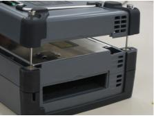
5. Tighten the four screws.
