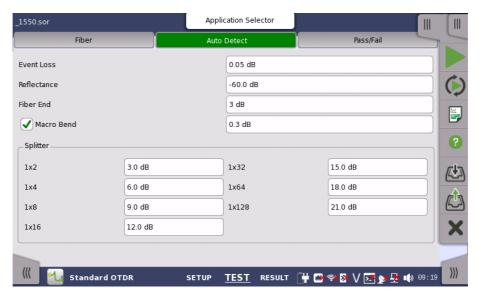
Set thresholds to detect events automatically in Auto Detect screen. Events that exceed the Auto Detect parameter settings are reported in the Event Analysis table.
