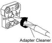
3. Press the tip of a new (dry) adapter cleaner into the ferrule end surface and then wipe in one direction 2 or 3 times to dry the surface.
