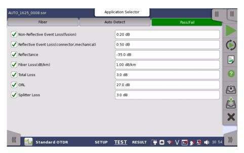
This screen allows users to set thresholds to Pass/Fail tests.
