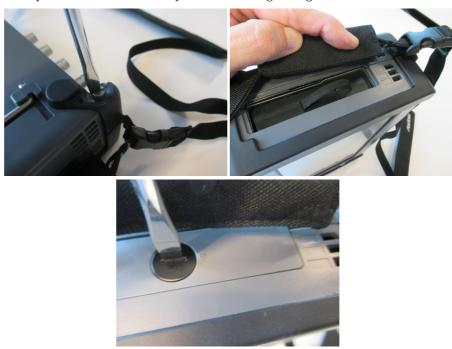
9. Attach MT1000A and MU100010A , insert the battery pack and mount the battery lid with the reverse sequence at the beginning.
