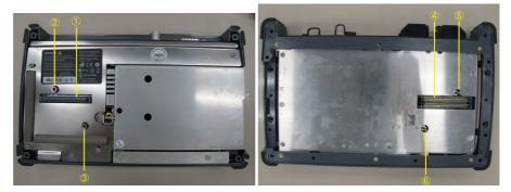
3. Insert screws 1U in B0728A Rear Panel Kit to four corners of the rear panel.
