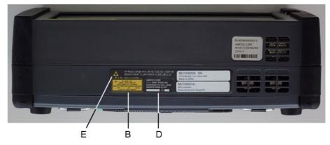
Figure 6: Locations of labels (Bottom side of MU100020A, MU100021A, MU100022A, MU100023A)
