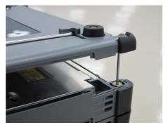
5. Tighten the four screws.
