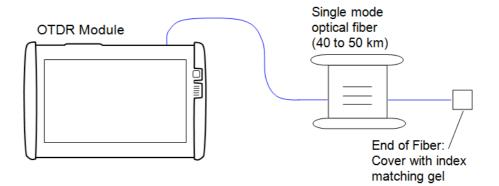
Connection diagram for wavelengths other than 1650 nm
