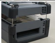
5. Tighten the four screws.
