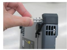
4. Attach 10G Multirate module to OTDR module. Place 10G Multirate module on the OTDR modules as to connect following pairs: 7 - 10, 8 - 11, 9 - 12. Be careful not to bump the guide pins (8, 9, 11 and 12) to the connectors (7 and 10).
