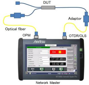
Loss is displayed as the differential between the reference and the measured power.
