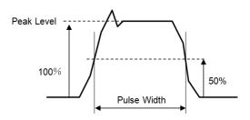
Width of the waveform to be measured
