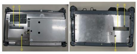
3. Remove four screws of 10G Multirate module and replace to screws 2U in B0728A Rear Panel Kit.
