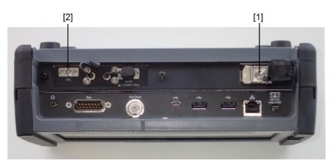
Figure 1: Locations of laser aperture (MU100020A)
