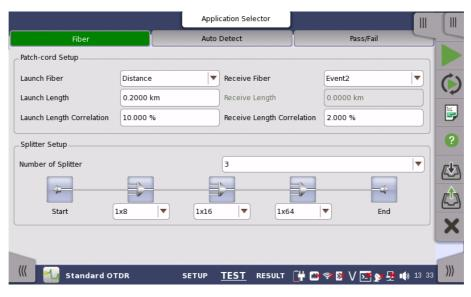
In addition to the various parameters, the **Test** screen also contains the <u>Application toolbar</u> and the navigation tabs for horizontal and vertical navigation.
