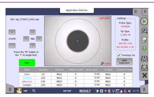
This screen displays the image taken by the fiber scope. Analyzing an image of the fiber edge surface is also available.
