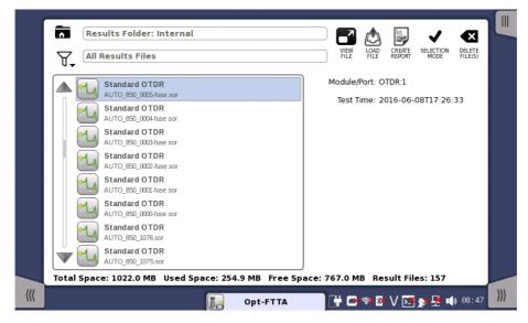
Creating a *workspace* for a previous test allows you to view the test results in the GUI. You are brought directly to the *Test Results* screen when you touch the **View/Load File** button, but can navigate to the other screens in the workspace from there.
