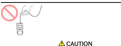
Be careful not to hit the end of an optical connector against anything hard such as the floor or a desk by dropping the optical fiber cable.
