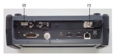
Figure 3: Locations of laser aperture (MU100022A)
