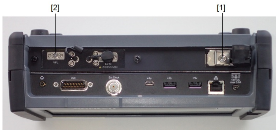
Figure 1: Locations of laser aperture (MU100020A)
