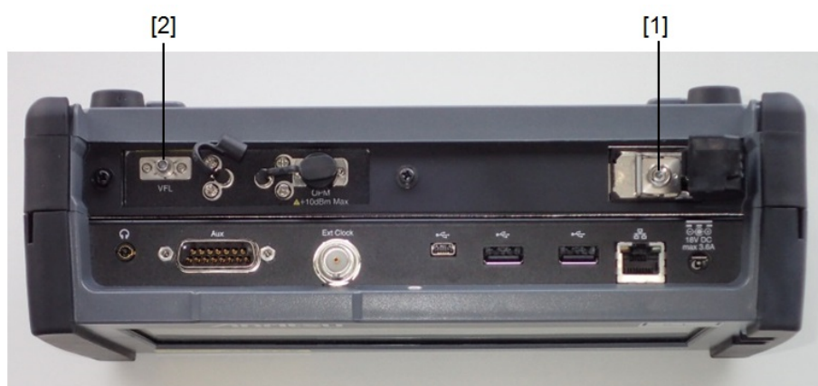
Figure 3: Locations of laser aperture (MU100022A)
