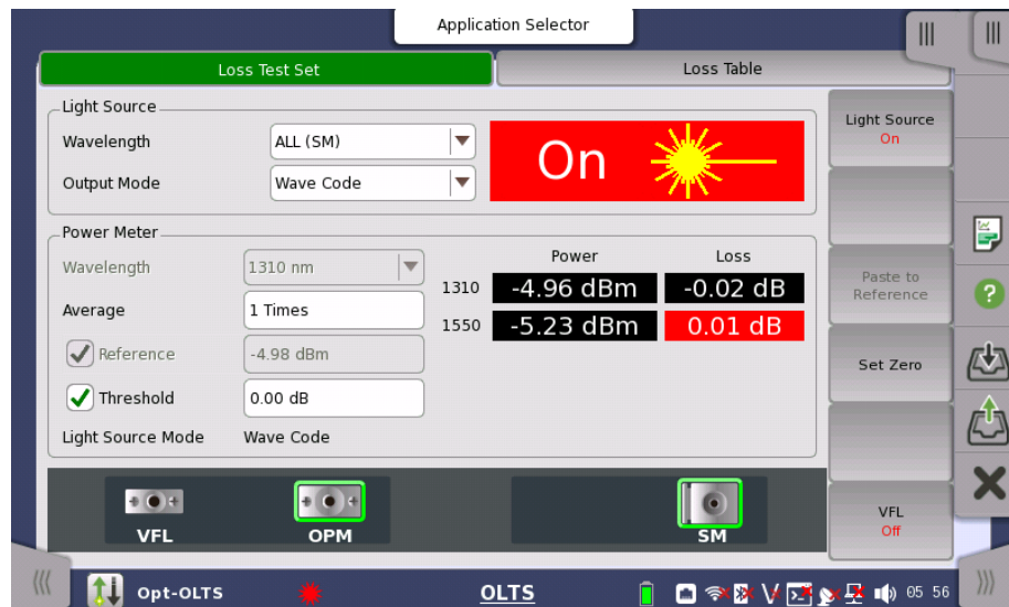
Receiving Light Modulated by Wave Code
