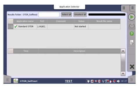
This screen displays the Pass/Fail results and status of the scenario execution. To run the scenario, touch  $\bigcirc$  in the Application Toolbar.
