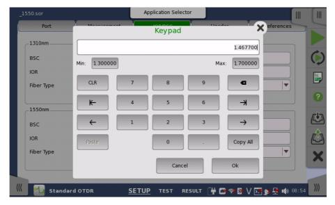
In general, a keypad consists of the character/number keys, a display field showing the current text/number entry, various editing-related keys. For number entries, the minimum and maximum values allowed are also shown. When you launch a keypad from a field, the current field value is shown in the keypad's display field.
