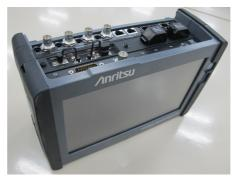
$6. \ \mbox{After attaching the modules, connect the AC cord or install the battery packs.}$
