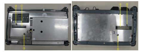
3. Insert screws 1U in B0728A Rear Panel Kit to four corners of the rear panel.
