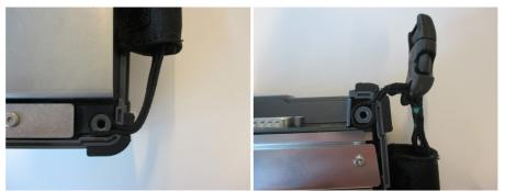
$\ensuremath{\mathsf{7.}}$  Remove the buckle cap from the handle and the carrying strap.
