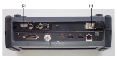
Figure 1: Locations of laser aperture (MU100020A)
