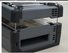
5. Tighten the four screws.
