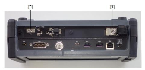
Figure 3: Locations of laser aperture (MU100022A)
