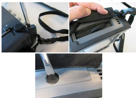
9. Attach the Network Master and MU100010A , insert the battery pack and mount the battery lid with the reverse sequence at the beginning.
