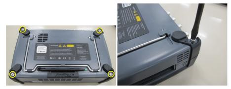
5. After loosing the four screws, lift up the 10G Multirate Module with holding both sides. If you cannot lift up, loosen the four screws again. You can see the panel as below.
