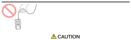
Be careful not to hit the end of an optical connector against anything hard such as the floor or a desk by dropping the optical fiber cable.
