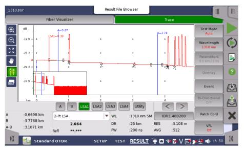
The LSA 2-Point Loss is the change in dB (Y-Axis) calculated between the two points. When the Cursor A, Y-Axis position is greater than the Cursor B, Y-Axis position, a positive loss measurement is displayed.
