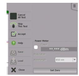
To measure the optical power, touch the tab at right-top to expand <u>Application</u> <u>Toolbar</u>.
