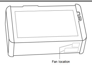
In this instrument, cooling air is taken in through the side panel, and hot air is exhausted through the bottom panel. When using MT1000A on a desk, open the <u>support stand</u> on the rear the panel
