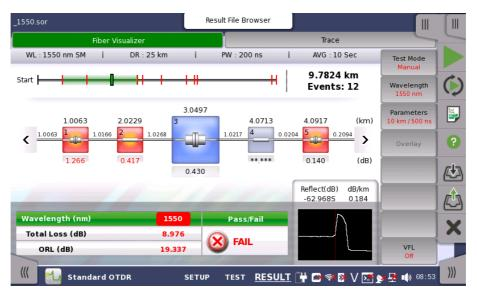
In addition to the results, whose presentation varies from application to application, the **Test results** screen also contains soft keys in right-hand. To save results to a file, touch in the <u>Application toolbar</u>.
