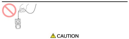
Be careful not to hit the end of an optical connector against anything hard such as the floor or a desk by dropping the optical fiber cable.
