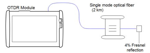
When testing the distance measurement accuracy of 850 nm and 1300 nm, change the optical fiber in Connection diagram to the multi-mode fiber (2 km).
