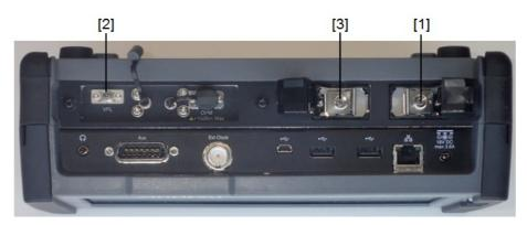
Figure 2: Locations of laser aperture (MU100021A and MU100023A)
