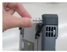
4. Attach 10G Multirate module to OTDR module. Place 10G Multirate module on the OTDR modules as to connect following pairs:
