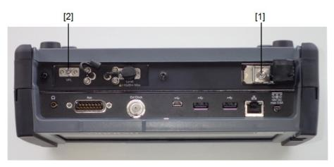
Figure 1: Locations of laser aperture (MU100020A)
