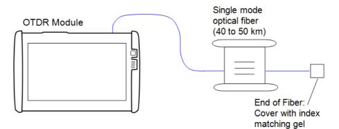
Connection diagram for wavelengths other than 1650 nm
