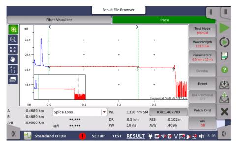
In the Trace screen, the fiber loss versus distance is shown in graphical. The following icons appear on the traces.
