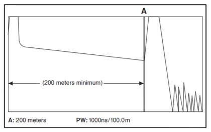
8. Zoom in on the trace to place Cursor A as close as possible to the rising edge of the reflection. Cursor A must be placed on a linear section of the waveform backscatter and NOT the rising edge of the reflection. (See the figure in step 7 which uses a 1  $\mu$  s pulse width and yields a 200 meter minimum distance between origin and Cursor A placement.)
