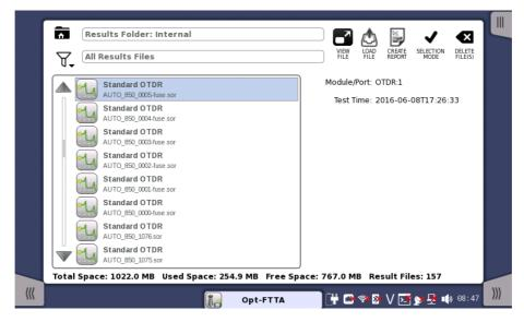
Creating a *workspace* for a previous test allows you to view the test results in the GUI. You are brought directly to the *Test Results* screen when you touch the **VIEW FILE/LOAD FILE** button, but can navigate to the other screens in the workspace from there.
