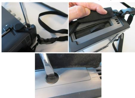
9. Attach the Network Master and MU100010A , insert the battery pack and mount the battery lid with the reverse sequence at the beginning.
