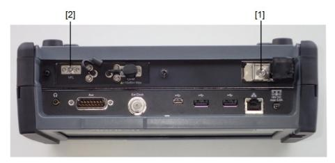
Figure 3: Locations of laser aperture (MU100022A)
