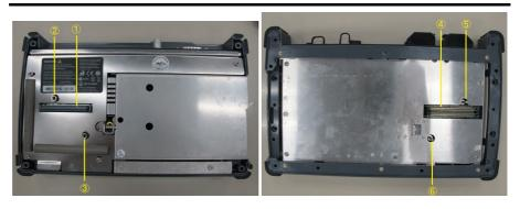
$3. \,$  Insert screws 1U in B0728A Rear Panel Kit to four corners of the rear panel.
