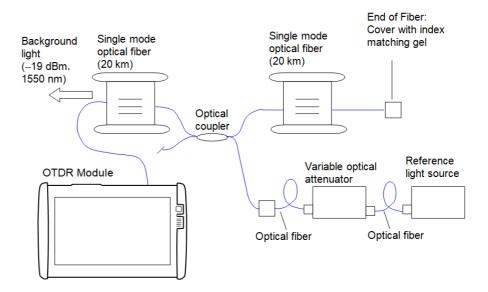
Connection diagram for 1650 nm wavelength
