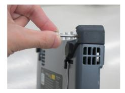
4. Attach 10G Multirate module to OTDR module. Place 10G Multirate module on the OTDR modules as to connect following pairs: 7 - 10, 8 - 11, 9 - 12.
