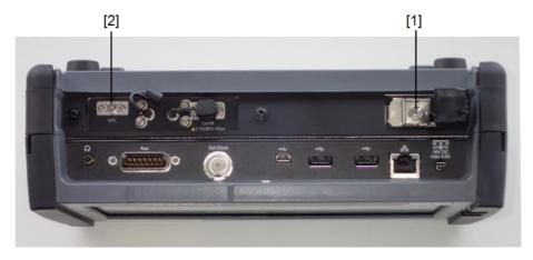
Figure 1: Locations of laser aperture (MU100020A)
