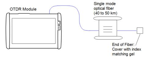
When testing the linearity of 850 nm, change the optical fiber in Connection diagram to the multi-mode fiber (20 to 25 km).
