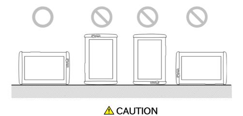
If the MT1000A is not installed in the "correct" orientation as above, a small shock may turn it over and harm the user.
