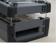
5. Tighten the four screws.
