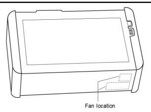
In this instrument, cooling air is taken in through the bottom panel. When using MT1000A on a desk, open the <u>support stand</u> on the rear the panel.
