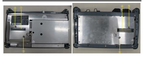
3. Remove four screws of 10G Multirate module and replace to screws 2U in B0728A Rear Panel Kit.
