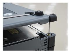
5. Tighten the four screws.
