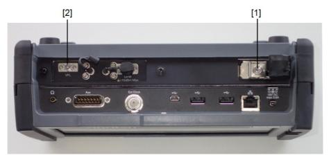
Figure 1: Locations of laser aperture (MU100020A)
