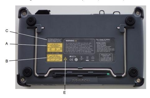
Figure 4: Locations of labels (MU100020A, MU100021A, MU100022A, MU100023A with Rear panel)
