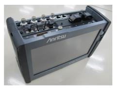
$6.\,$  After attaching the modules, connect the AC cord or install the battery packs.
