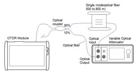
When testing the dead zone of 850 nm and 1300 nm, change the optical fiber and the optical coupler in Connection diagram to the multi-mode fiber. Use the variable optical attenuator for multi mode fiber.
