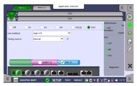
For the switching method between PDH Tx and DSn Tx, refer to <u>Physical Setup</u> in "E1 Setup and Status". Touch **DS3** radio button. Touching **Off** radio button disables the transmitter.
