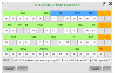
This dialog box presents detailed information about the overhead and allows you to configure it. Blue fields are OTU overhead. Green fields except FAS and MFAS are ODU overhead. Orange fields are OPU overhead.
