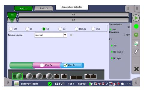
For the switching method between PDH Tx and DSn Tx, refer to <u>Physical Setup</u> in "E1 Setup and Status". Touch **E3** radio button. Touching **Off** radio button disables the transmitter.
