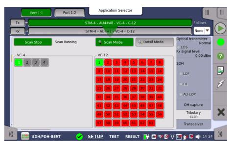
This screen allows to measure the alarms and errors of all VC-containers in the High order or the Low order at the same time. Note that the Low order scan is performed against the High order channel which you have selected.
