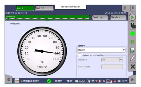
To view throughput information, select **Throughput** in the drop-down menu and then expand the dial. Use the drop-down menu above the expanded dial to select the relevant layer. When **Ethernet** is selected on the 'Threshold' of Test Setup screen, the **Ethernet** information appears in the upper right-hand corner, shows pass/fail status summary. Touching the **Details** button allows you to inspect the individual pass/fail status.
