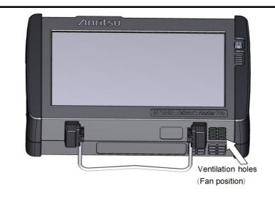
In the Network Master, cooling air is taken in through the bottom panel, and hot air is exhausted through the top panel. When using MT1040A on a desk, open the <u>support stand</u> on the rear panel or the bottom panel.
