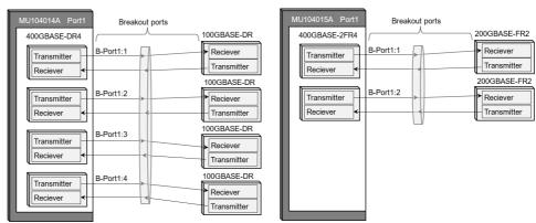
Breakout ports of MU104014A (QSFP-DD) Breakout ports of MU104015A (OSFP)
