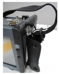
4. Fold the strap back through the buckle and tie it inside the handle.
