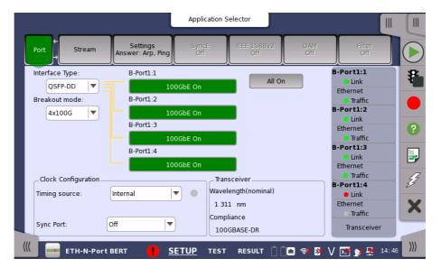
Interface Type and Breakout mode are set as below depending on the module to be used.
