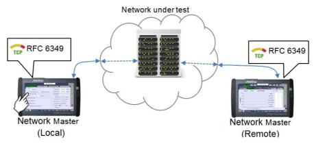
The required setup to perform RFC 6349 test is transferred from the 'local' Network Master to 'remote' Network Master when the test is started.
