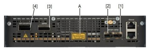
Figure 2: Locations of Laser Beam Aperture (MU104014A)
