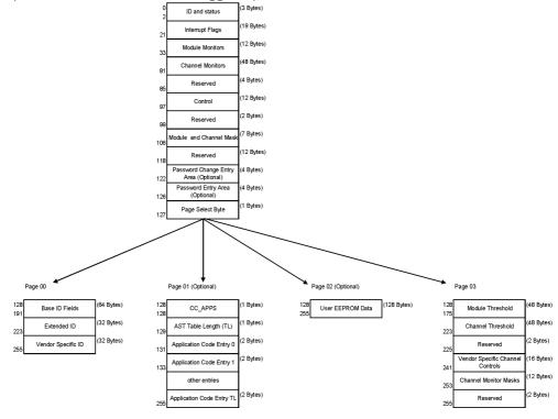
Registers in the transceiver are defined in *INF-8438i Specification for QSFP* (Quad Small Form factor Pluggable) Transceiver.
