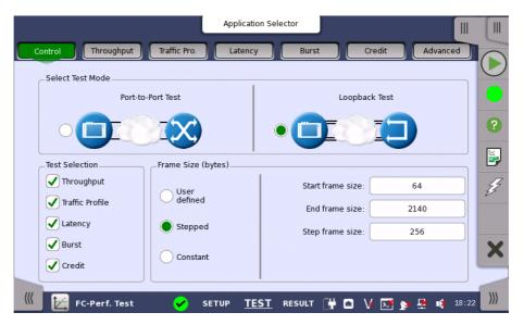
Specify the test mode and select the test to be performed in this screen.
