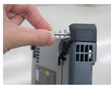
4. Attach the 10G Multirate module to the MU100090A. Place the 10G Multirate module on the MU100090A so as to connect the following pairs: 7 - 10, 8 - 11, 9 - 12.
