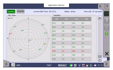
This screen displays positions of satellite and the logged data. Touch a left top button to switch the result to display.
