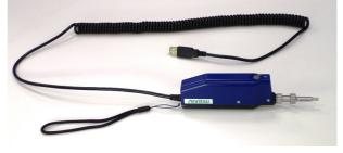
Connect the USB connector of the Video Inspection Probe to Network Master.
