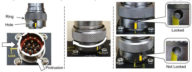
Check one of the yellow markers on the DC plug is aligned to the Lock marker on the connector panel. The DC plug is not locked unless the protrusions fit into the holes.
