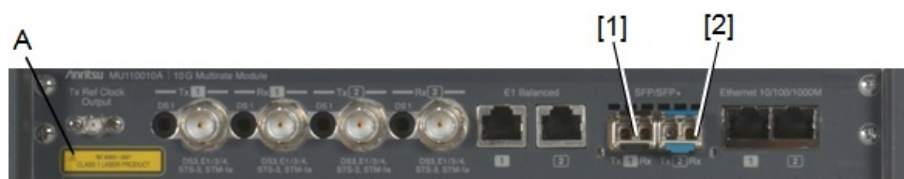
Figure 1: Locations of laser beam aperture (MU110010A)
