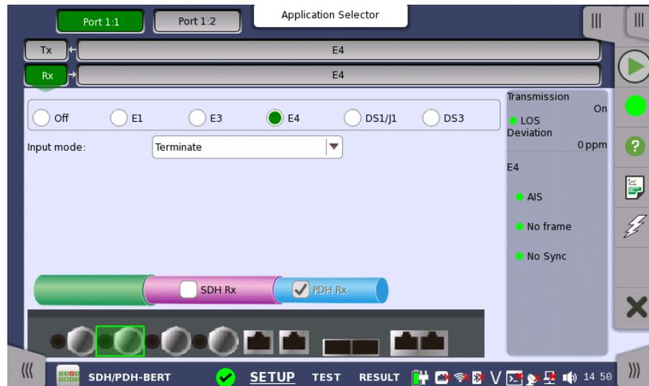
For the switching method between PDH Rx and DS<sub>n</sub> Rx, refer to [Physical Setup](#) in "E1 Setup and Status". Touch **E4** radio button. Touching **Off** radio button disables the receiver.
