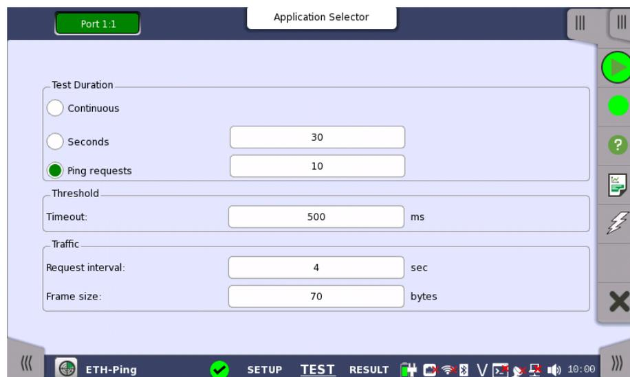
This screen allows you to configure the Ping test conditions for the currently selected port.
