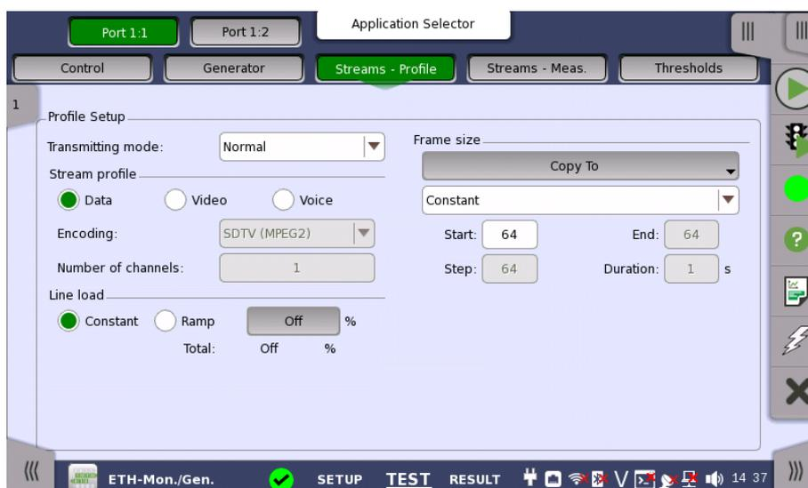
This screen contains the parameters for specifying a profile and pattern for each stream and for specifying which measurements are made.
