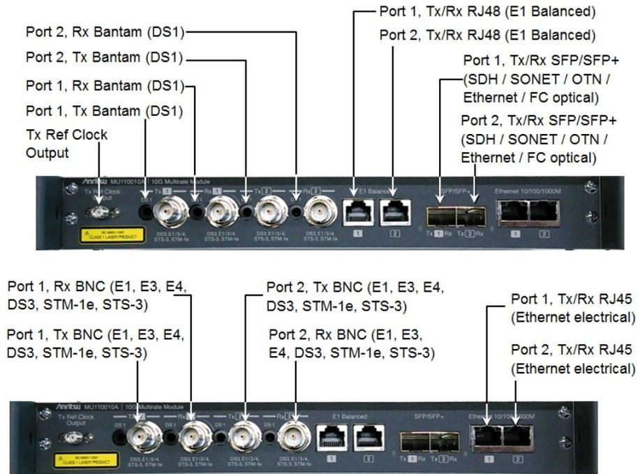
Tx Ref Clk Output: This connector is used for reference clock output.
