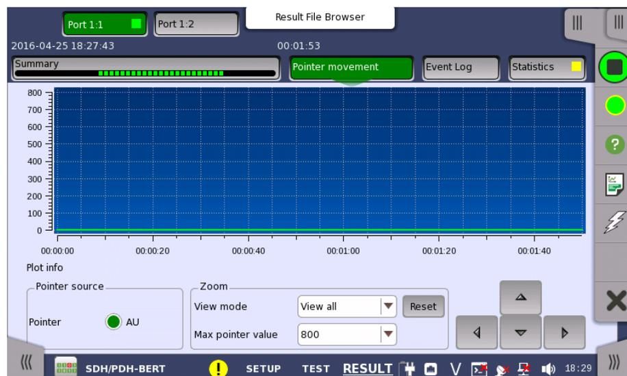
This screen presents a detailed analysis of pointer movements in the monitored signal. The results are displayed as a graph, showing the positions of a specific pointer over time.
