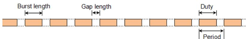
The value set to the **Gap length** field is an average of inter burst gaps.
