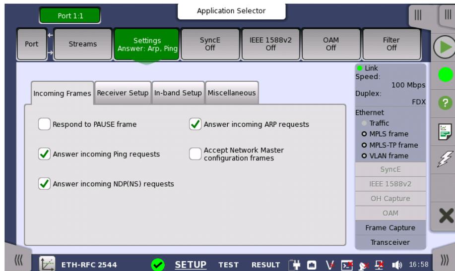
This screen allows you to specify how the Network Master handles incoming frames on the currently selected Ethernet port. It can also be used to inspect the current status of the selected port.
