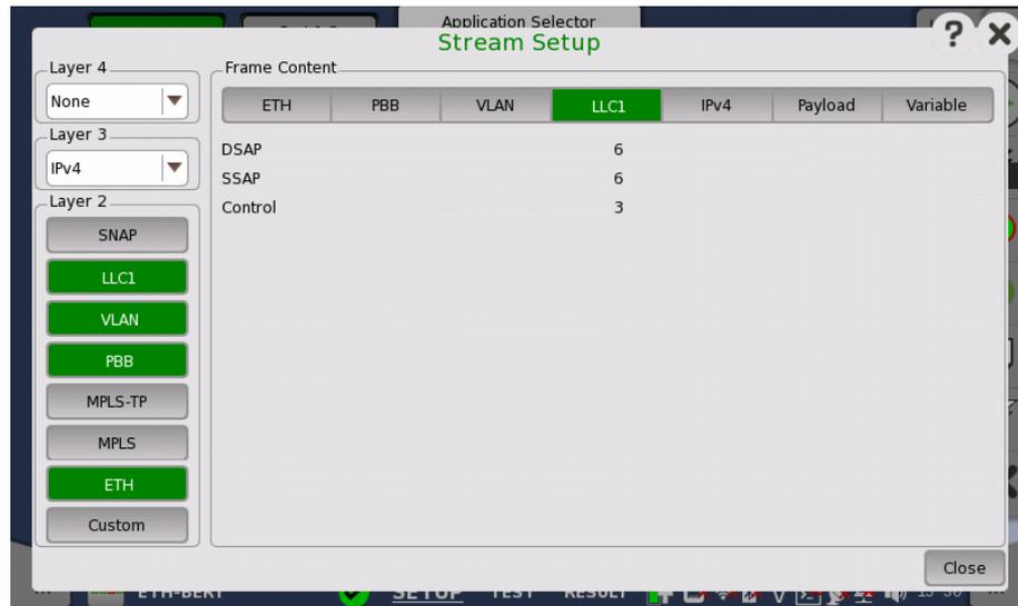
The **DSAP**, **SSAP** and **Control** fields are set automatically, based on the upper protocol layer.
