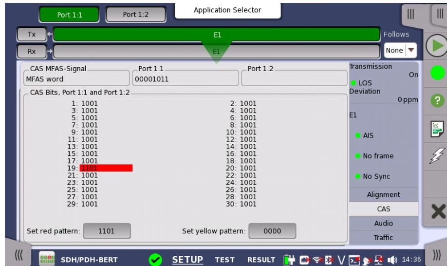
This screen gives information on the CAS (Channel Associated Signaling) signaling when available. It displays the state of the four signaling bits in both directions for all 30 channels. Activity is indicated with bold characters.
