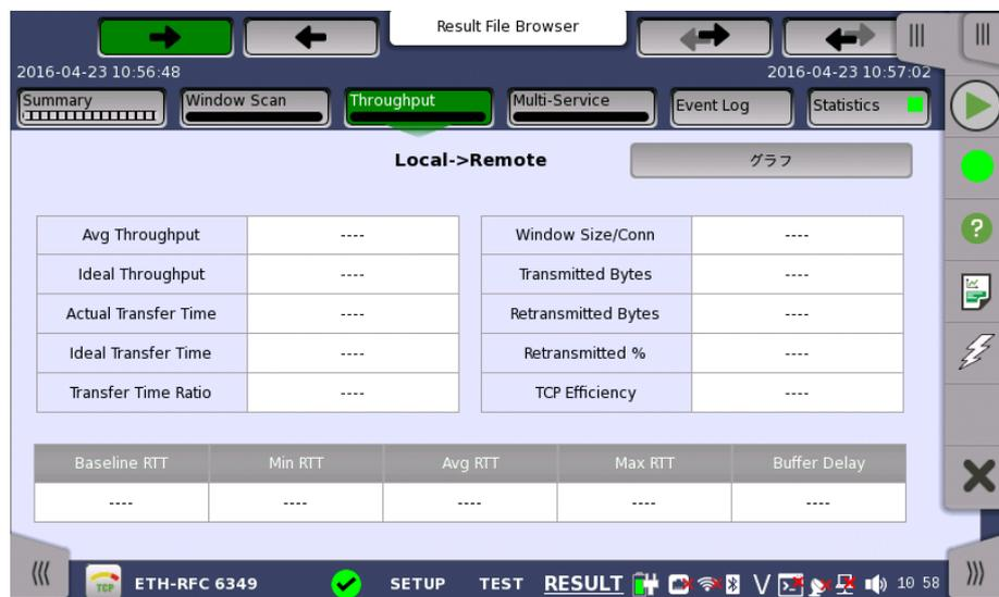
This screen presents the Throughput results in graph or table. Touch the **Graph** and **Table** buttons to switch between the tabular form and a graphical presentation of the results.
