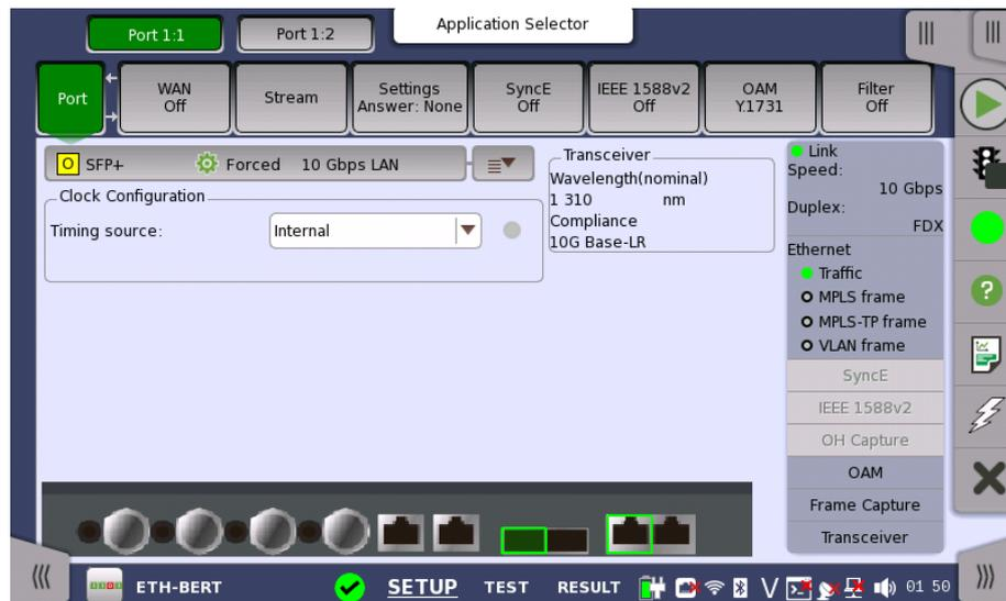
This screen allows you to specify the physical port configuration of the currently selected [Ethernet](#) port. It can also be used to inspect the current status of the selected port.
