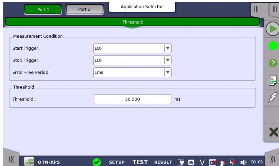
This screen contains the parameters for setting up the threshold values for errors and Pass/Fail status.
