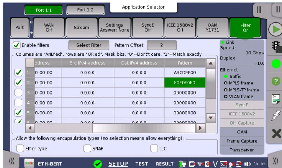
This screen allows you to set up filters and masks for the reception of Ethernet frames. It can also be used to inspect the current status of the selected port.
