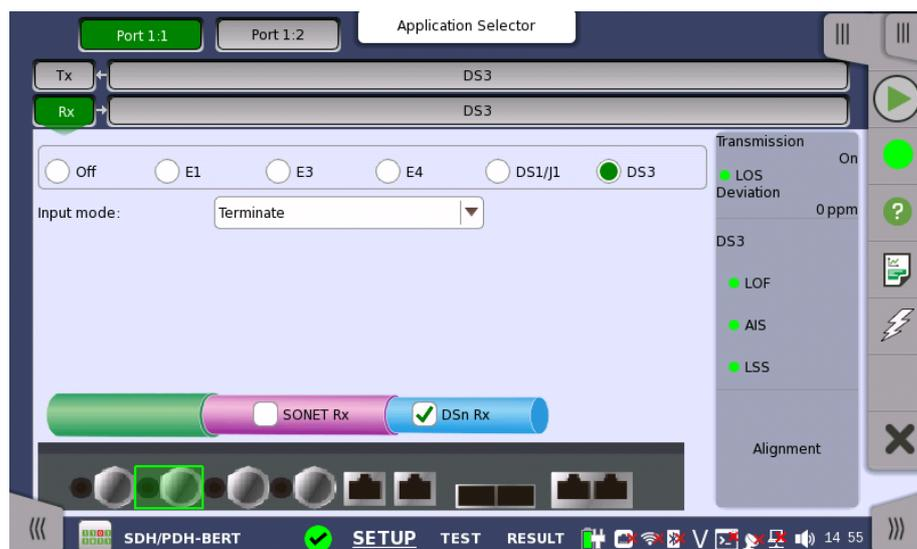
For the switching method between PDH Rx and DSn Rx, refer to [Physical Setup](#) in "E1 Setup and Status". Touch **DS3** radio button. Touching **Off** radio button disables the receiver.
