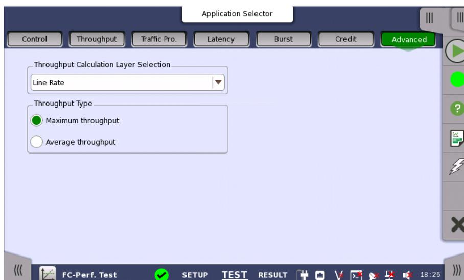
This screen sets the measurement method of *Measured Throughput* for the results of subsequent tests. The displays of the measurement results are not changed even if the Advanced settings are changed after completing the measurement.
