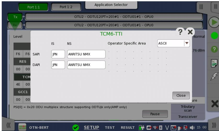
In the byte-specific dialog box, select the display format (ASCII or Hex) using the **Operator Specific Area** drop-down menu.
