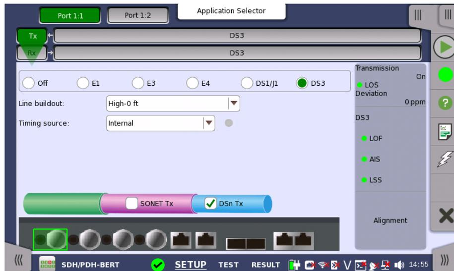
For the switching method between PDH Tx and DS<sub>n</sub> Tx, refer to [Physical Setup](#) in "E1 Setup and Status". Touch **DS3** radio button. Touching **Off** radio button disables the transmitter.
