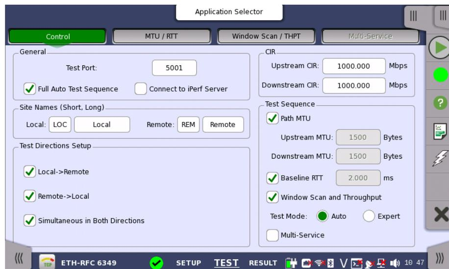
This screen allows you to specify your test mode and select which RFC 6349 tests to carry out.
