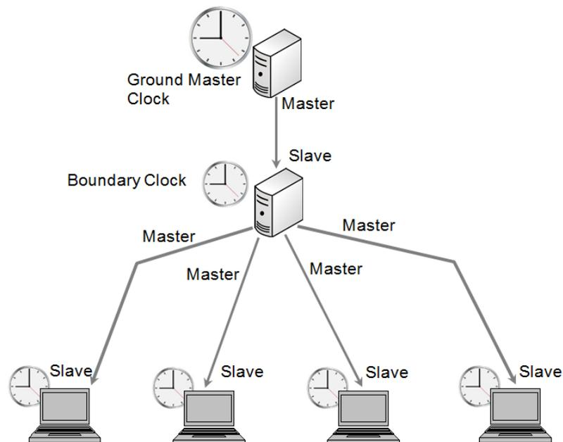
The clock may be set up in either normal or unicast mode.
