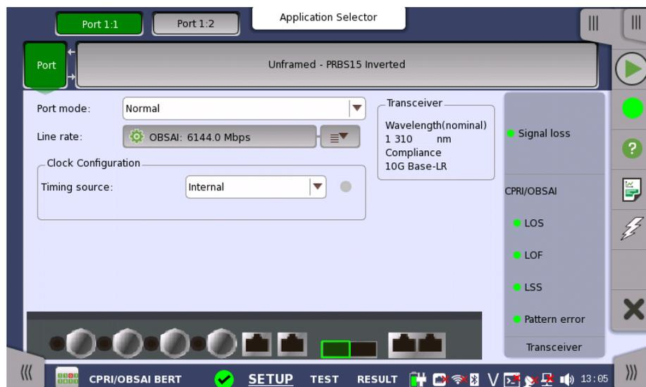
This screen allows you to specify the physical port configuration of the currently selected CPRI/OBSAI port. It can also be used to inspect the current status of the selected port.
