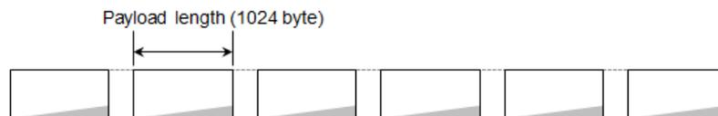
When the check box *is* selected, Payload pattern is divided and set to the payload in Ethernet frames so that the payload pattern is successive through Ethernet frames.
