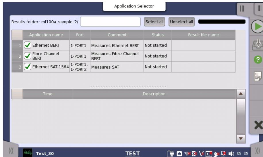
This screen displays the Pass/Fail results and status of the scenario execution. Select the check box for the application name you want to run.
