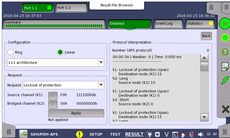
This screen shows a protocol interpretation for the selected port (i.e. detailed decoding information about K1 and K2 during the test). It also contains a set of parameters that allow you to configure the requests used in the test.
