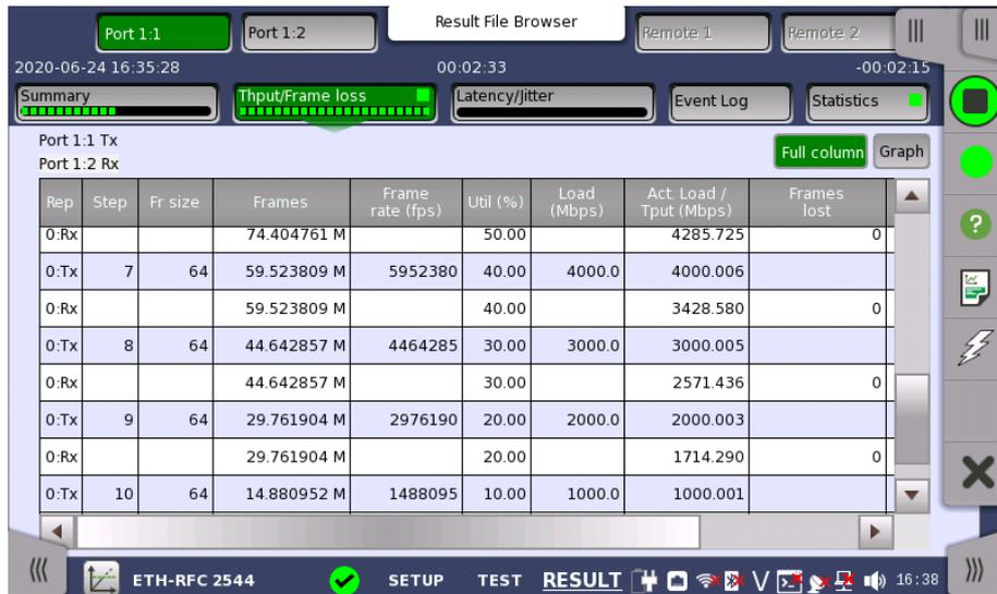
This screen presents the results from the Throughput and frame loss test.
