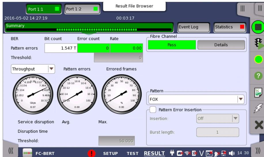
This screen contains a summary of the results of the Fibre Channel BERT test. The information includes such things as number of pattern errors, average and maximum disruption time, and number of exceeded thresholds.
