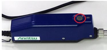
When using G0382A, pressing the M button on VIP starts capturing and analyzing an image.
