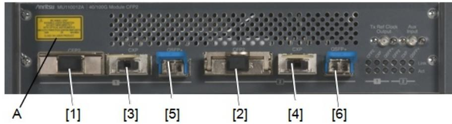
Figure 3: Locations of Laser Beam Aperture (MU110012A)
