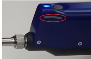
If it cannot be recognized that the fiber edge surface is in the image, VIP may not perform autofocus. In that case, get a focus using < or > button on G0382A.
