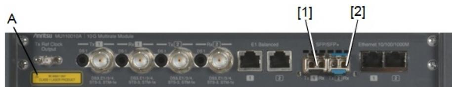
Figure 1: Locations of Laser Beam Aperture (MU110010A)
