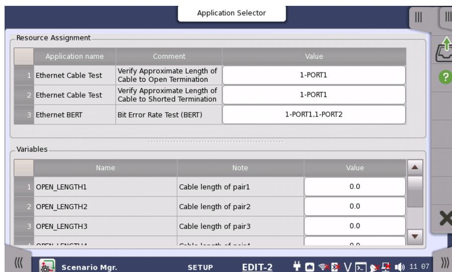
Touch the **SETUP** at the bottom of the screen to return to the setup screen.
