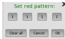
The color pattern consists of four binary digits. The minimum and the maximum acceptable value is 0000 and 1111, respectively. Touch the digit buttons to set the relevant value and then touch **Ok**.
