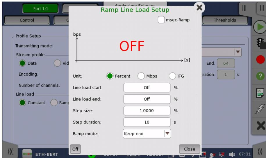
The line load unit can be specified from **Percent**, **Mbps**, and **IFG**. When IFG (Inter frame gap) is specified to the unit, 12 byte setting means the 100% utilization. The value set to the field is an average of Inter frame gap. When Transmission mode is **Normal**, 100% or more line load can be set in specific case.
