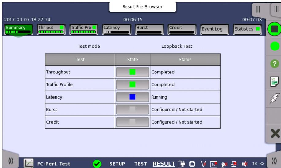
This screen presents the current status of the test(s) (**Configured / Not started**, **Running**, **Completed** or **Not Configured**). Touching the State button of the specific test displays the screen where the detailed result information is displayed.
