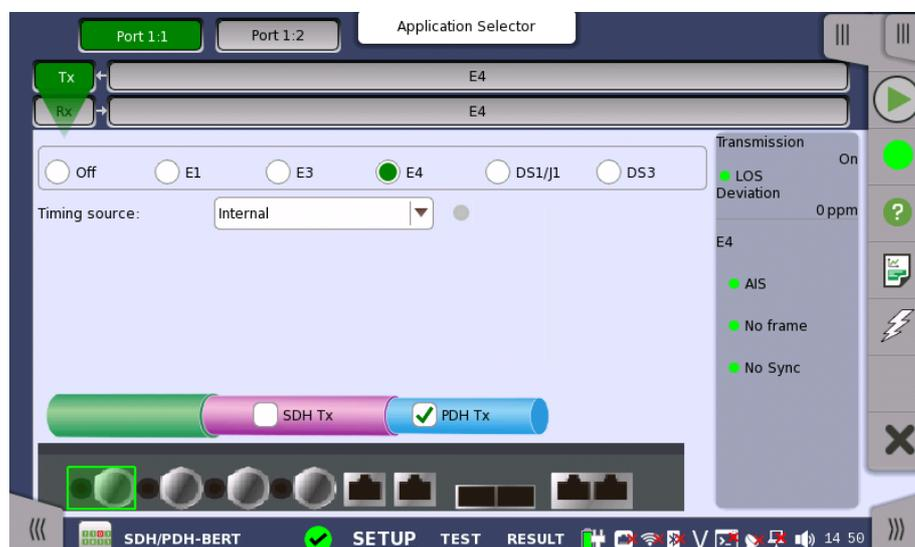
For the switching method between PDH Tx and DSn Tx, refer to [Physical Setup](#) in "E1 Setup and Status". Touch **E4** radio button. Touching **Off** radio button disables the transmitter.
