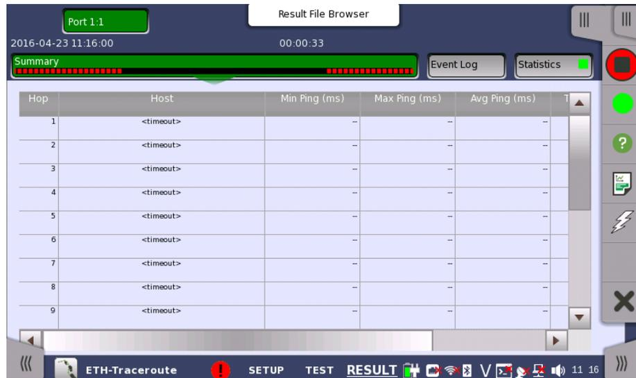
This screen shows the status/results of a running Traceroute test, or the results of the most recently completed test.
