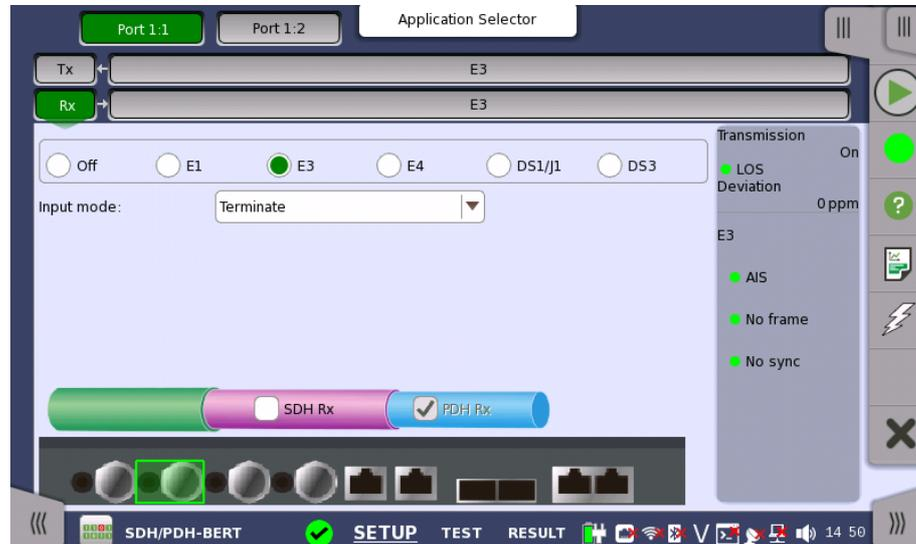
For the switching method between PDH Rx and DS<sub>n</sub> Rx, refer to [Physical Setup](#) in "E1 Setup and Status". Touch **E3** radio button. Touching **Off** radio button disables the receiver.
