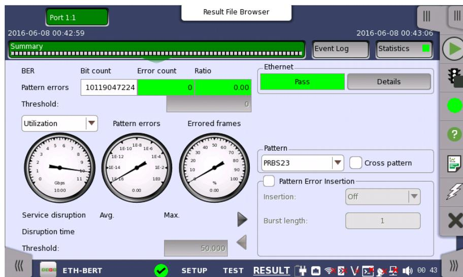
This screen contains a summary of the results of the Ethernet BERT test. The information includes such things as number of pattern errors, average and maximum disruption time, and number of exceeded thresholds.
