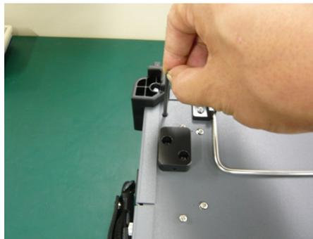
6. After loosening the four screws, lift up the Power Supply Module with holding both sides. You can see the side panel of the Multirate module as below.
