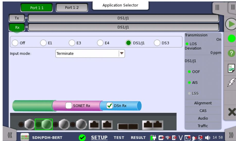
For the switching method between PDH Rx and DSn Rx, refer to [Physical Setup](#) in "E1 Setup and Status". Touch **DS1/J1** radio button. Touching **Off** radio button disables the receiver.
