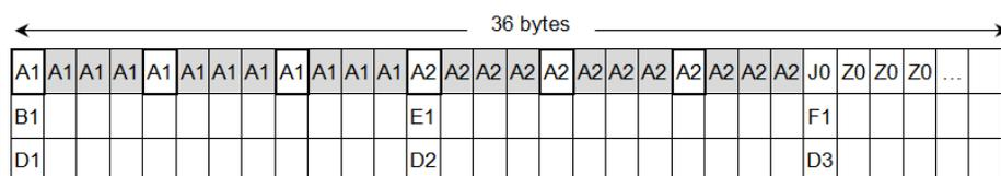
\*: For STM-256, SOH Editor can edit each three bytes both side of the boundary of A1 bytes and A2 bytes. The other A1A2 bytes in gray cell are fixed to F6h or 28h.
