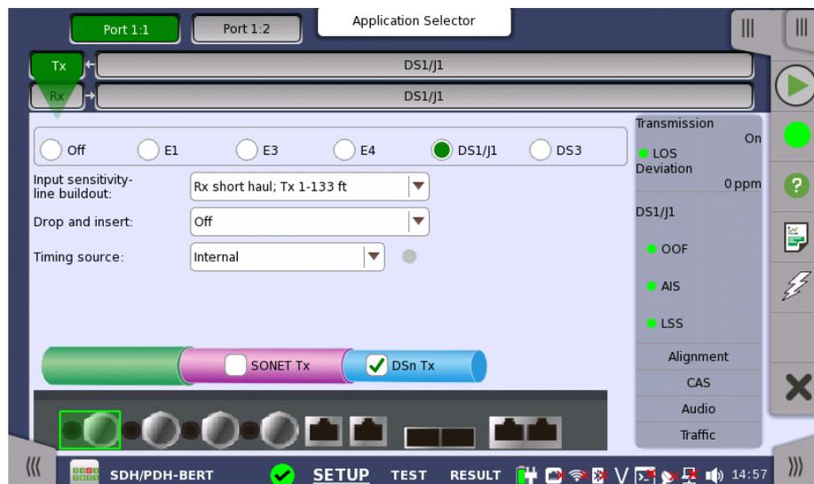
For the switching method between PDH Tx and DSn Tx, refer to [Physical Setup](#) in "E1 Setup and Status". Touching **Off** radio button disables the transmitter.
