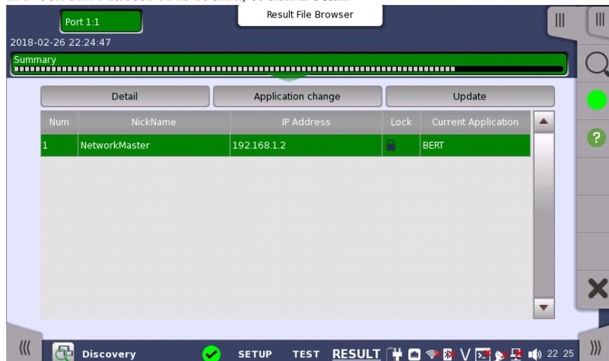
6. Select **RFC2544** as the application to run on Network Master A. Enter a MAC address, IP addresses, and password used for RFC 2544 test of Network Master A.
