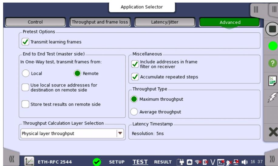
This screen allows you to specify various advanced settings for the RFC 2544 test(s).
