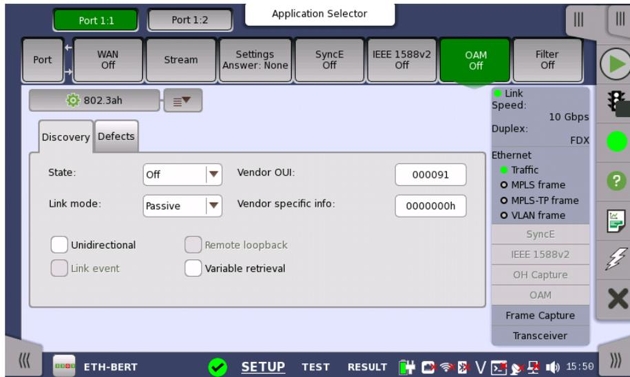
OAM (Operation, Administration and Management) is a group of management functions that provides system or network fault indication, performance monitoring, security management, diagnostic functions, configuration and user provisioning.
