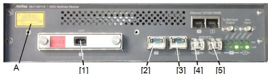
Figure 2: Locations of Laser Beam Aperture (MU110011A)
