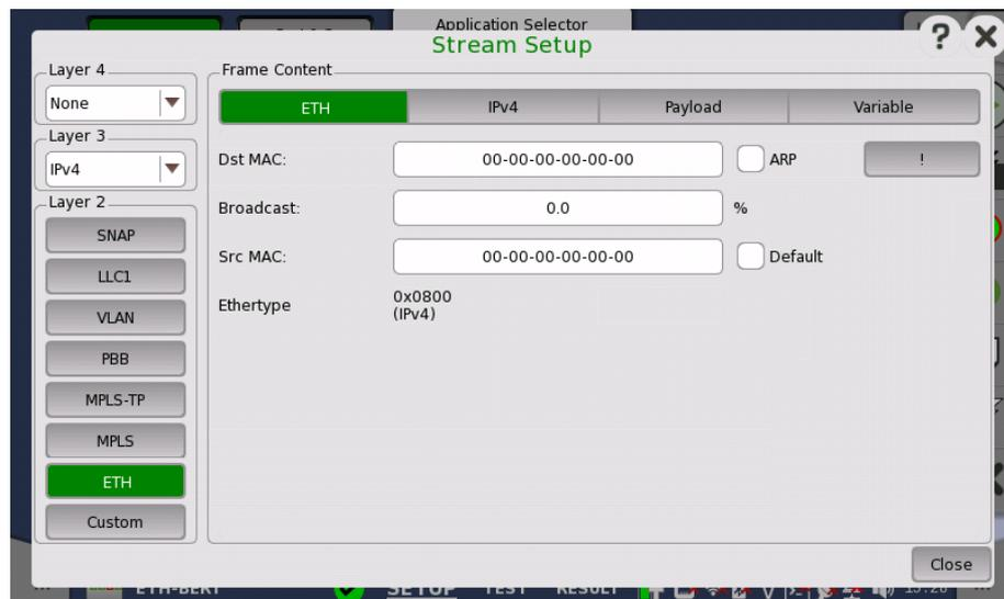
The layer buttons are arranged in order from bottom to top and from left to right. The TCP/UDP protocols are the uppermost layer and Ethernet the lowermost as depicted below compared to the OSI model.
