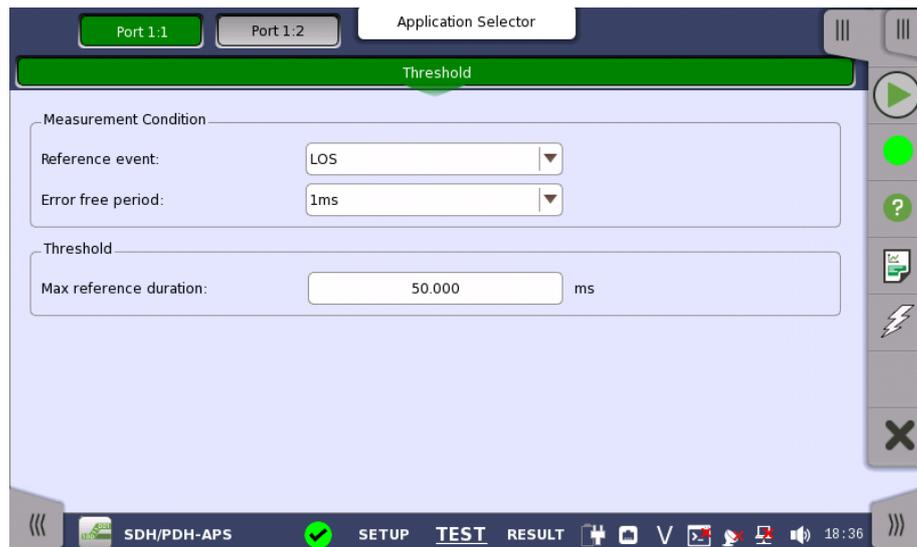
This screen contains the parameters for setting up the threshold values for alarms/errors and Pass/Fail status.
