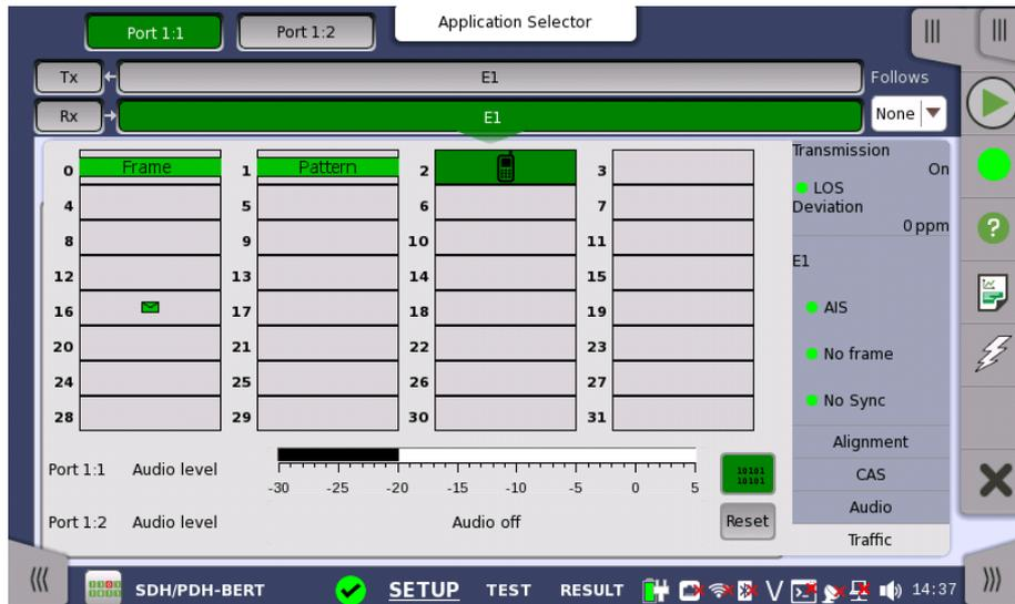
This screen shows the activity of the speech channels represented on the 2 Mbps line. You can switch between a traffic display and a view of the time slot content.
