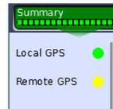
When Test Sync. Mode is set to **GPS** on Control screen, status for the GPS time synchronization is displayed at the top of the screen with colored Lamps - one Lamp for the local side and one for the remote side.
