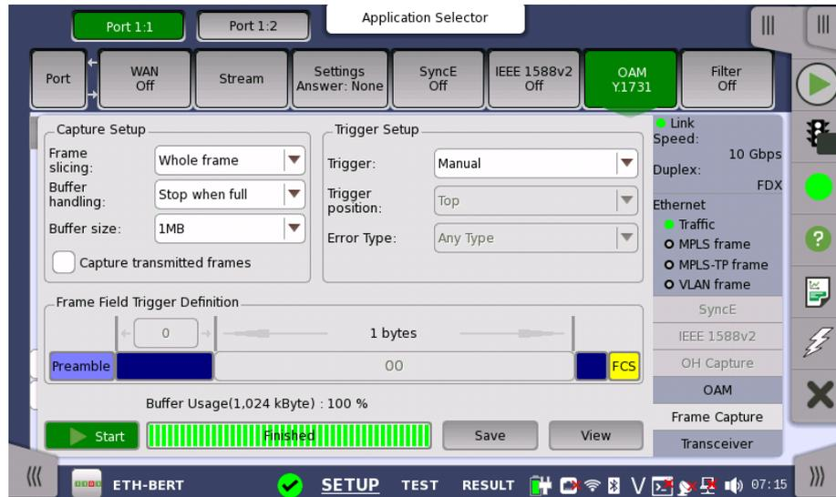
This screen allows you to set up and execute capture of transmitted frames.
