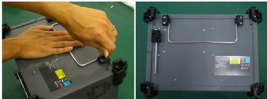
5. After attaching the modules, connect the AC cable or install the battery packs.
