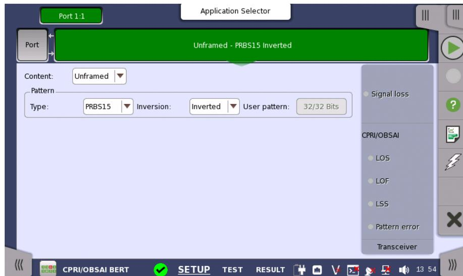
This screen allows you to specify the frame structure of the currently selected port.
