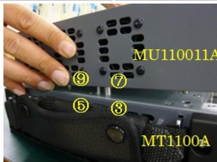
3. Tighten the four screws (shown in yellow circle) using Z1862A, with holding MU110011A by the other hand. Tighten screws enough to prevent the module from dropping off.
