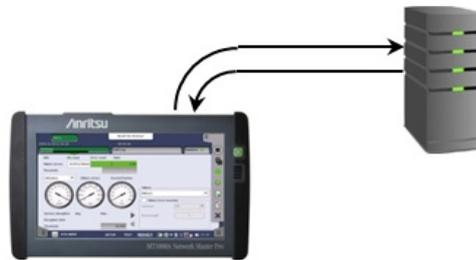
**Fabric** is the connection using fibre channel switch. Touch **Fabric Login** button to access to the fabric login server.
