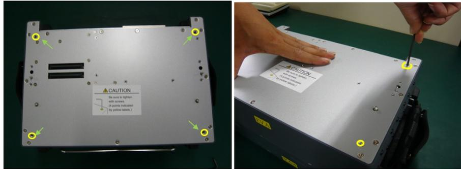
4. Place MU110001A on MU110011A. The attaching procedure of MU110001A is the same as attaching MU110011A to MT1100A.
