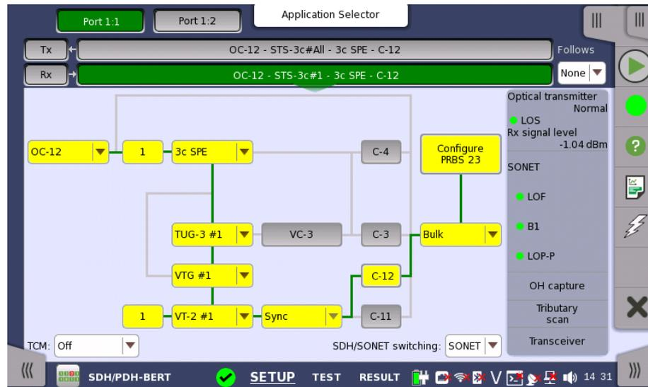
The manner of setting up the SONET interface of receiver is the same as that of transmitter. Refer to [SONET Frame Setup](#).
