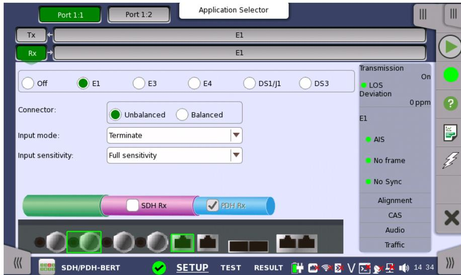
Switching between PDH Rx and DS<sub>n</sub> Rx is done in the SDH/SONET receiver setup screen.
