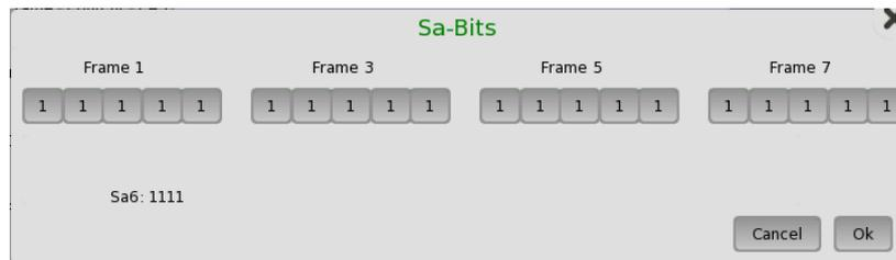
In the **Sa-Bits** dialog box, change the individual Sa-bits by touching on the relevant bit keys - this will toggle the bit key's binary value from logic 1 to 0 or vice versa. Touch **Ok** to accept the changes and close the dialog.
