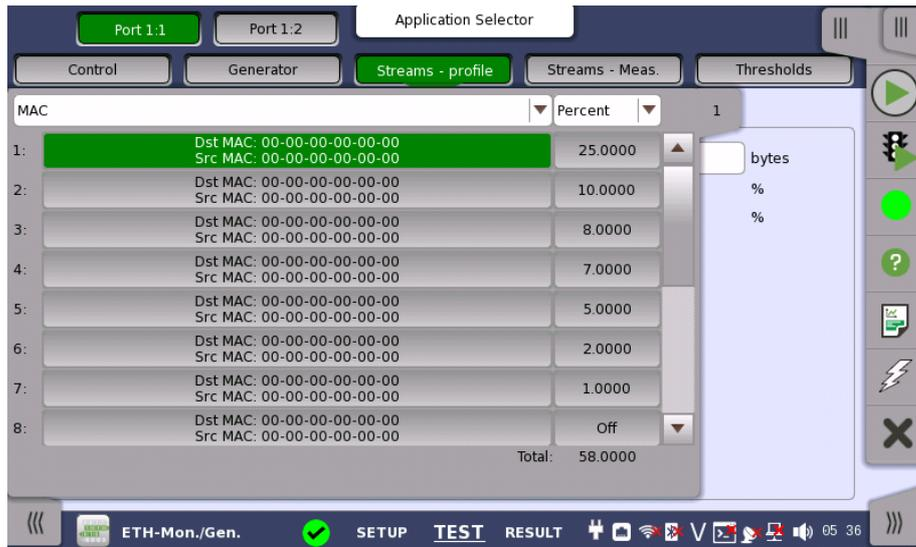
At the top of the slide-out list you can switch between MAC, IP, and VLAN information as stream identification.
