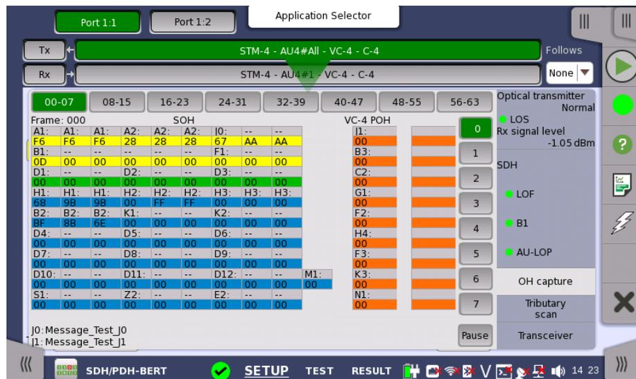
This screen shows SDH capture status information for one frame at a time. The frame number captured in one time is 64. Touch the frame selection buttons to select which frame to display.
