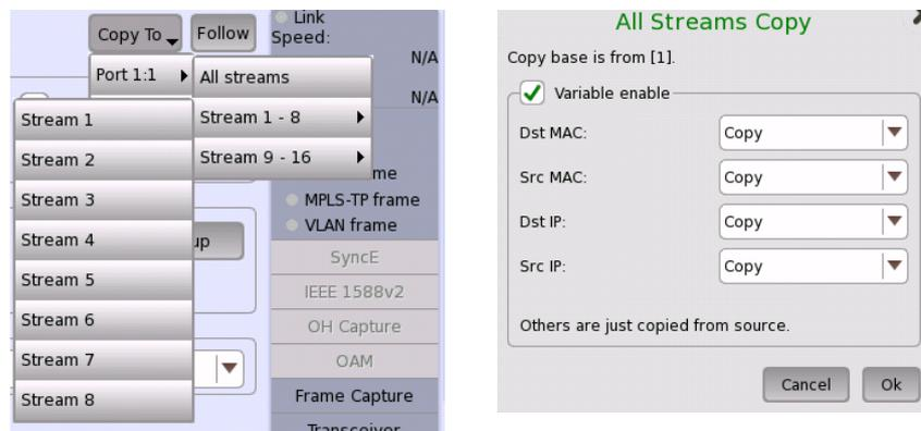
When copying settings to all streams, it is available to change MAC or IP address with selecting **Variable enable** check box. If the check box is not selected, same address is copied to all streams.
