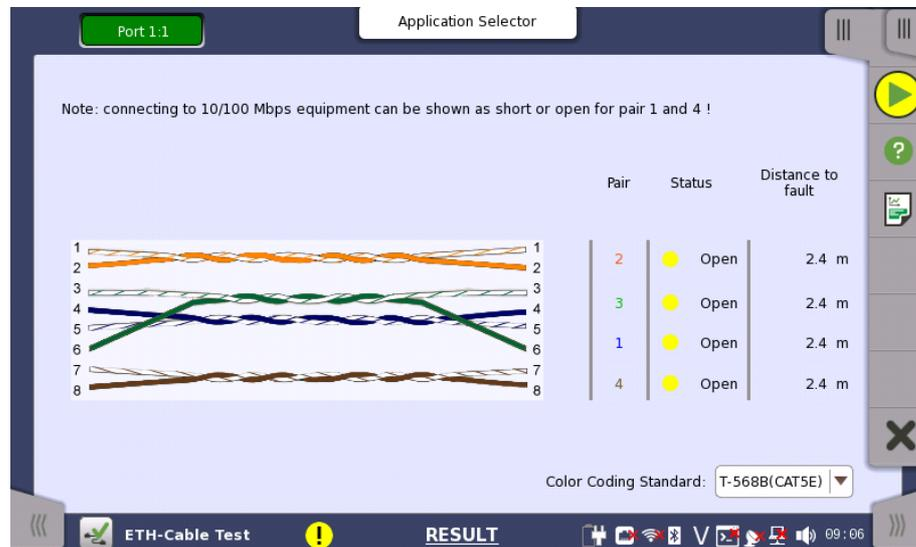
This screen allows you to control and monitor an [Ethernet Cable Test](#).
