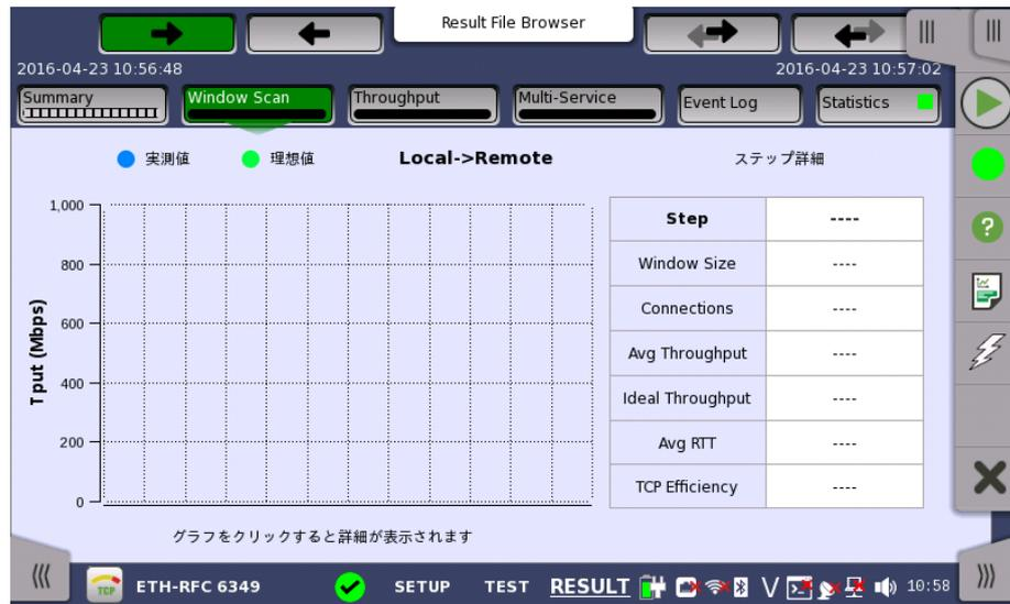
This screen presents the results from the Window Scan test. The ideal throughput and the actual throughput are shown in the chart. If touching on the Graph bars, step details appear in the right hand table.
