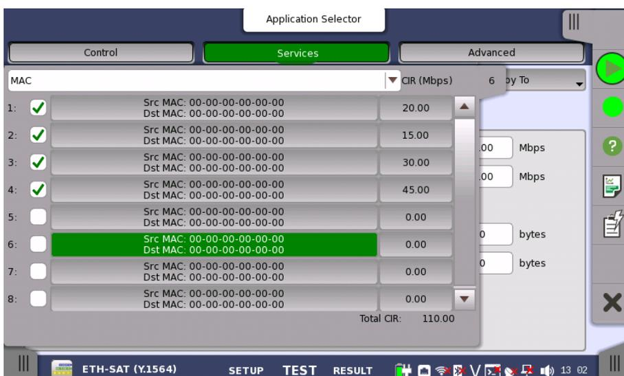
Use the **Enabled** check box to enable/disable the service specified in the **Service** field.
