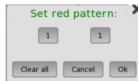
The color pattern consists of four binary digits for ESF/J1 frame. For SF/D4 frame, it consists of two binary digits. The minimum acceptable value is 00 or 0000, and the maximum acceptable value is 11 or 1111. Touch the digit buttons to set the relevant value and then touch **Ok**.
