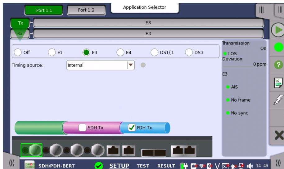
For the switching method between PDH Tx and DSn Tx, refer to [Physical Setup](#) in "E1 Setup and Status". Touch **E3** radio button. Touching **Off** radio button disables the transmitter.
