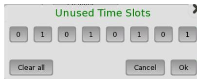
In the **Unused time slots** dialog box, change the individual bits by touching on the relevant bit keys - this will toggle the bit key's binary value from logic 1 to 0 or vice versa. Touch **Ok** to accept the changes and close the dialog box.
