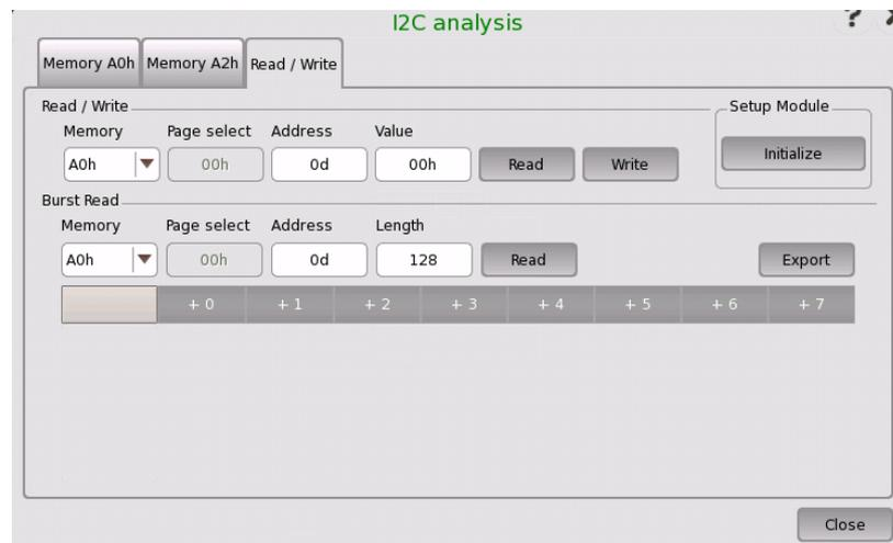
This dialog box allows reading/writing information into the registers of the optical transceiver via I<sup>2</sup>C (Inter-Integrated Circuit) interface.
