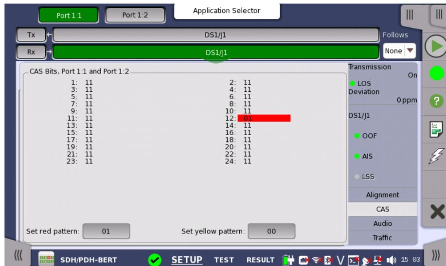
This screen gives information on the CAS (Channel Associated Signaling) signaling when available. It displays the state of the two signaling bits in both directions for all 24 channels. Activity is indicated with bold characters.
