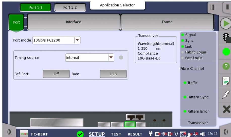
This screen allows you to specify the physical port configuration of the currently selected [Fibre Channel](#) port. It can also be used to inspect the current status of the selected port.
