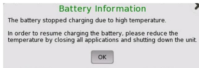
In order to resume battery charging as soon as possible, use the Network Master in the environment with lower ambient temperature. Or, close the application and shut down the Network Master.
