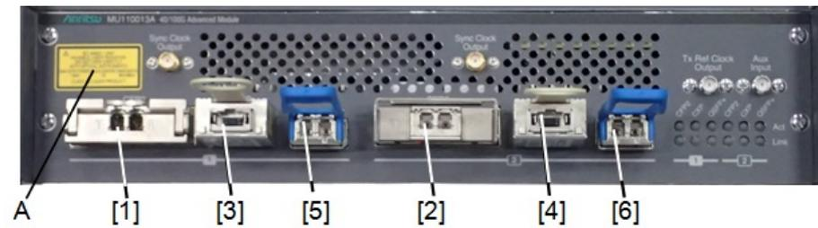
Figure 4: Locations of Laser Beam Aperture (MU110013A)
