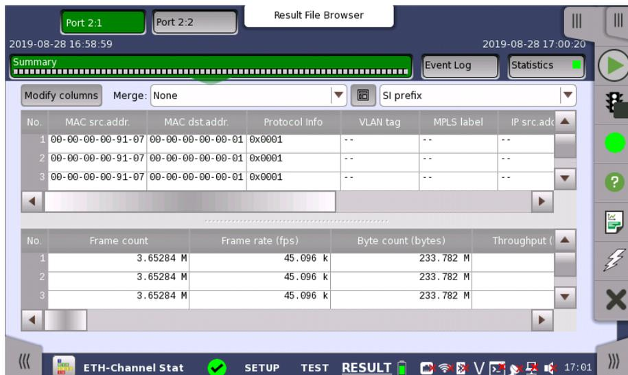
This screen presents the results of the Channel Statistics test. The screen contains two lists, one which lists the created channels and another which shows the results for each channel. Each channel is shown as a row in the two lists.
