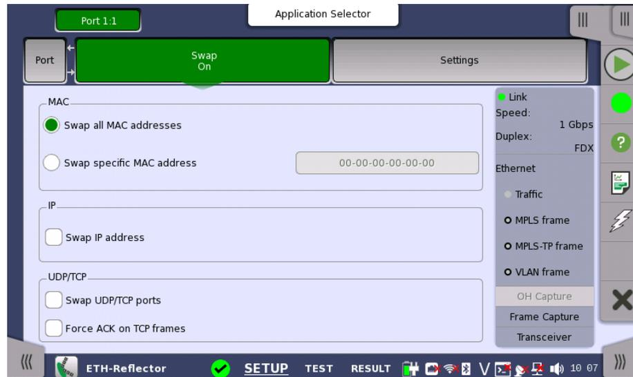
This screen is where you configure the traffic loop by specifying how addresses and/or ports are to be swapped and reflected.
