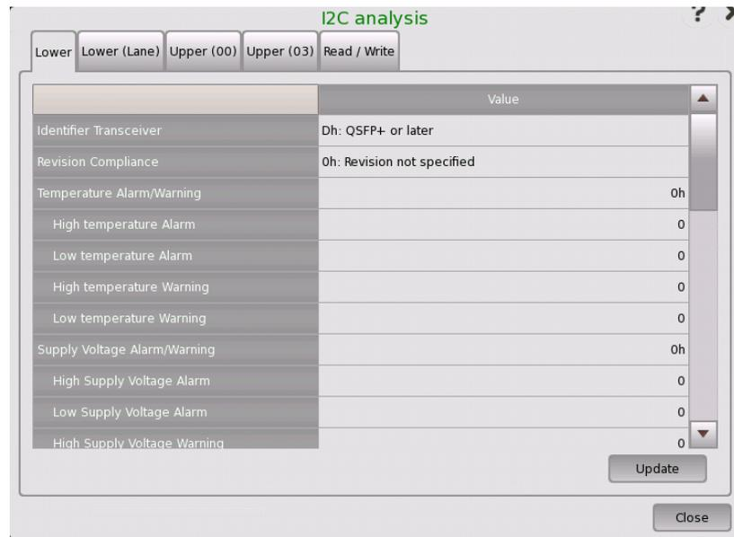
This dialog box allows reading/writing information into the registers of the optical transceiver via I<sup>2</sup>C (Inter-Integrated Circuit) interface.
