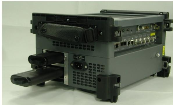
6. When installing the battery, note the direction of the battery terminals. With the instrument placed on its back - and the battery compartment in front of you - the terminals should be in the upper left corner.
