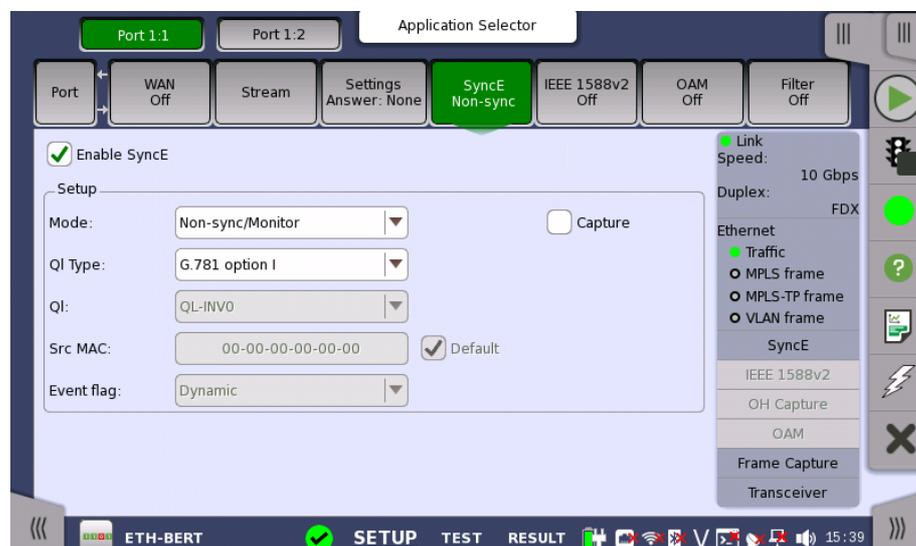
This screen allows you to configure the setup parameters related to Synchronous Ethernet. It can also be used to inspect the current status of the selected port.
