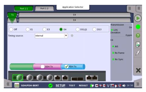
For the switching method between PDH Tx and DSn Tx, refer to <u>Physical Setup</u> in "E1 Setup and Status". Touch **E4** radio button. Touching **Off** radio button disables the transmitter.
