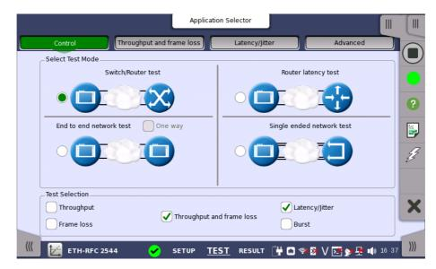
This screen allows you to specify your test mode and select which RFC 2544 tests to carry out.
