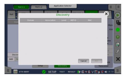
Devices will appear in the dialog's list as they are discovered. Select the device in the list and touch the **Add** button in the dialog box. The device is added to the list displayed on the Discovery view screen.
