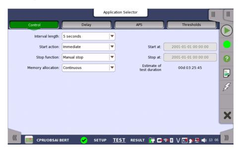
This screen contains the parameters that are generally required for BERT test.
