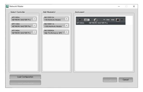
3. Set configuration of Network Master by clicking options in **Select Controller**, and **Add Module(s)**.
