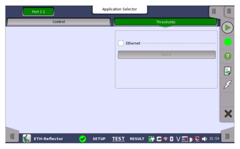
This screen allows you to set up a number of special monitoring items related to the various interface types. When specified and enabled, these threshold values (i.e. limits) for errors and Pass/Fail status will be used during the monitoring.
