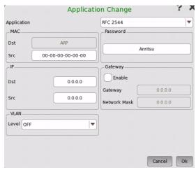
7. Touch **OK**. It takes a few minutes until the application of Network Master A is changed. MAC address, IP addresses, VLAN settings, and Gateway settings set in the Application Change dialog box will be set to <u>Streams</u> of Network Master A.
