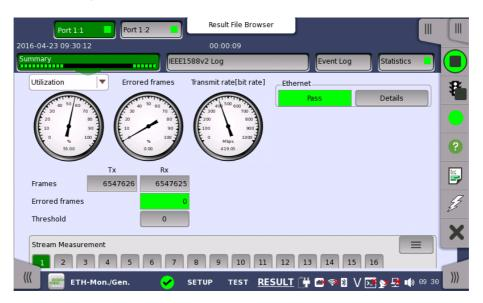
This screen contains a summary of the results of the Ethernet Monitor/Generate test. The information includes such things as number of errored frames and number of exceeded thresholds.
