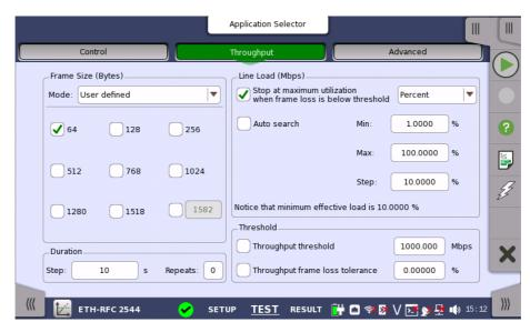
This screen allows you to configure the following parameters related to an RFC 2544 Throughput test:
