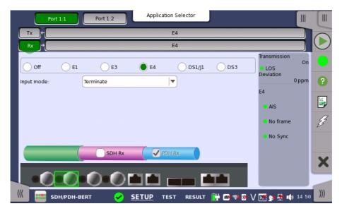
For the switching method between PDH Rx and DSn Rx, refer to <u>Physical Setup</u> in "E1 Setup and Status". Touch **E4** radio button. Touching **Off** radio button disables the receiver.
