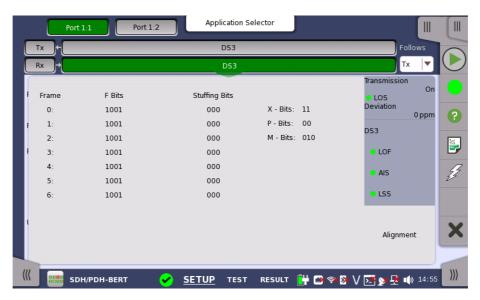
Alignment status when the frame type is M13
