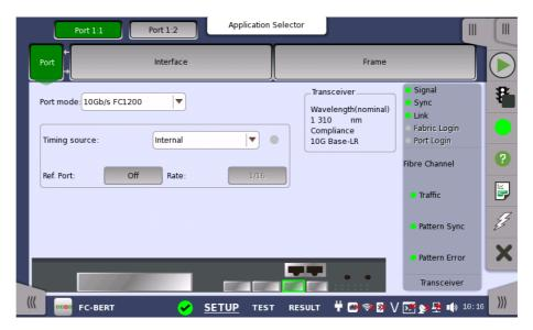
This screen allows you to specify the physical port configuration of the currently selected <u>Fibre Channel</u> port. It can also be used to inspect the current status of the selected port.
