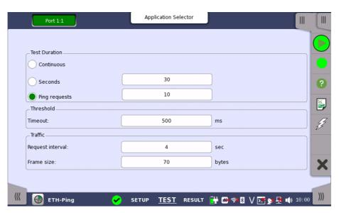
This screen allows you to configure the Ping test conditions for the currently selected port.
