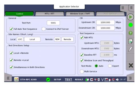
This screen allows you to specify your test mode and select which RFC 6349 tests to carry out.
