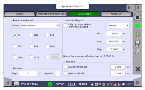
This screen allows you to configure the parameters related to an RFC 2544 Latency/Jitter test:
