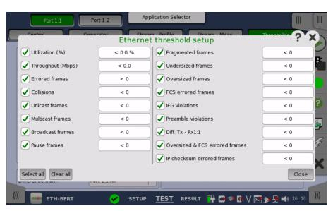
In the dialog box, select the check boxes for the relevant thresholds and then touch the **Close** button to list them on the **Thresholds** screen. You can select/deselect all check boxes in the dialog box by using the **Select all** / **Clear all** buttons. Touch the individual value fields either in the dialog box or in the list on the screen to specify the threshold values.
