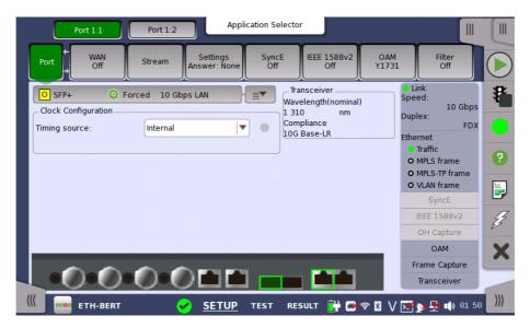
This screen allows you to specify the physical port configuration of the currently selected <u>Ethernet</u> port. It can also be used to inspect the current status of the selected port.
