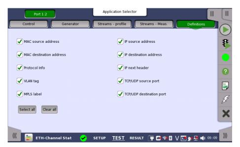
This screen is where you specify which frame characteristics are considered when performing the channel separation (i.e. which frame characteristics are active during the test). The maximum number of channels is 231.
