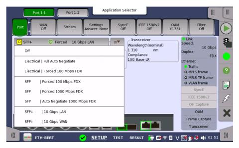
The quick setup menu contains a number of predefined port configurations (e.g. **Electrical | Forced 100 Mbps FDX**). The detailed mode dialog allows you to specify the configuration yourself.
