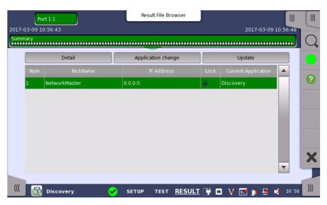
In this screen, up to 16 results of searching for Network Masters are displayed. If password is set to the Network Master, an icon appears in **Lock** row. Selecting a line by touching the table enables button operation.
