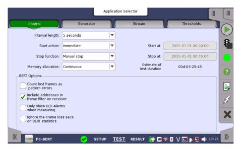
This screen contains the parameters that are generally required in a BERT test setup.
