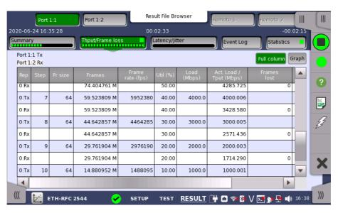
This screen presents the results from the Throughput and frame loss test.
