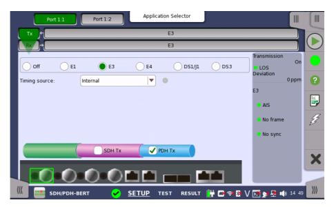
For the switching method between PDH Tx and DSn Tx, refer to <u>Physical Setup</u> in "E1 Setup and Status". Touch **E3** radio button. Touching **Off** radio button disables the transmitter.
