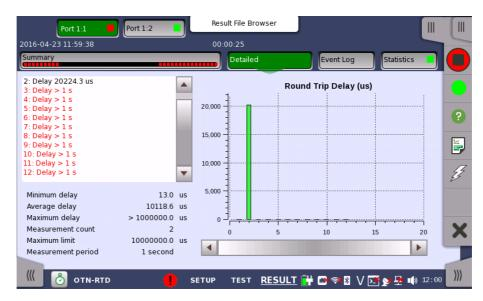
Buttons for selecting the relevant port are displayed at the top of the screen, with a color indication of the pass/fail status of the test.
