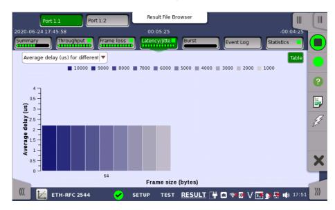
On the test-specific result screen, you switch between the two modes by using the  ${\bf Graph}$  and  ${\bf Table}$  buttons.
