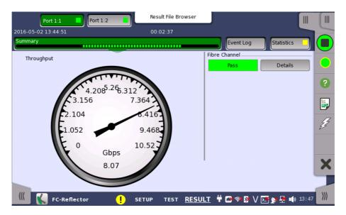
When **Fibre Channel** is selected on 'Threshold' of the Test Setup screen, the **Fibre Channel** information appears in the upper right-hand corner, shows pass/fail status summary. Touching the **Details** button allows you to inspect the individual pass/fail status.
