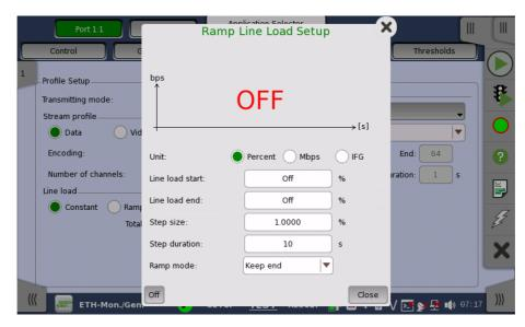
The line load unit can be specified from **Percent**, and **Mbps**. Touching **Off** at left-bottom stops sending the stream.
