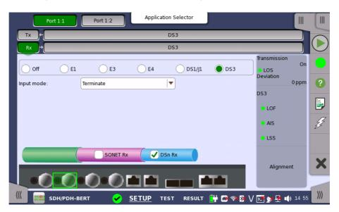
For the switching method between PDH Rx and DSn Rx, refer to <u>Physical Setup</u> in "E1 Setup and Status". Touch **DS3** radio button. Touching **Off** radio button disables the receiver.
