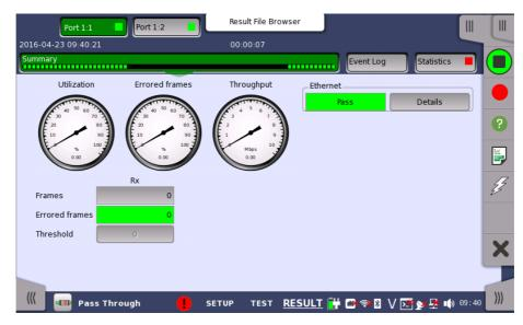
This screen contains a summary of the results of the Ethernet Pass Through test. The information includes such things as number of errored frames and number of exceeded thresholds.
