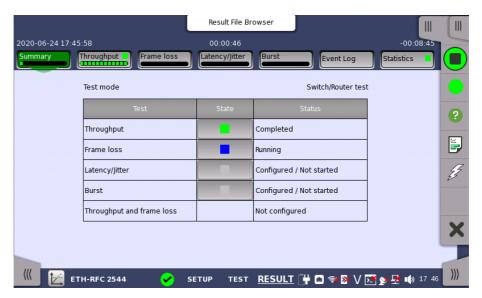
This screen presents the current status of the test(s) (Configured / Not Started, Running, Completed or Not Configured). Touching the status button for a specific test will display the result screen of the test.
