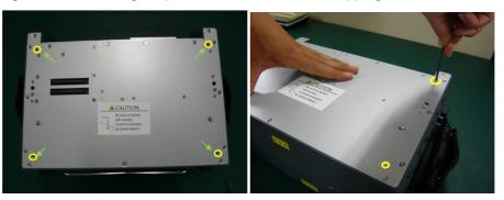
4. Place MU110001A on MU110011A. The attaching procedure of MU110001A is the same as attaching MU110011A to MT1100A.
