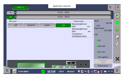
This screen allows you to make the physical setup of the receiver in OTN mode. It can also be used to inspect the current status of the selected port by the button in Navigation area.
