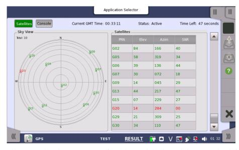
This screen displays positions of satellite and the logged data. Touch a left top button to switch the result to display.
