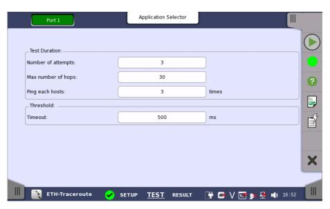
This screen allows you to configure the parameters related to a <u>Traceroute</u> test.
