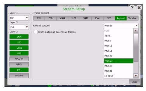
Open the Payload pattern drop-down menu to select the relevant pattern.
