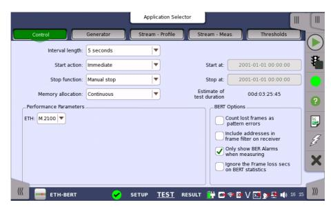
This screen contains the parameters that are generally required in a test setup.
