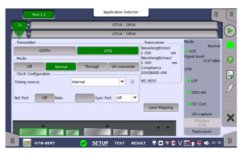
This screen allows you to enable the optical interface of the OTN transmitter. It can also be used to inspect the current status of the selected port by the button in Navigation area.
