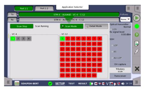
This screen allows to measure the alarms and errors of all VC-containers in the High order or the Low order at the same time. Note that the Low order scan is performed against the High order channel which you have selected.
