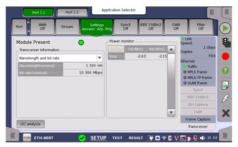
This screen presents status information about the optical transceiver (Pluggable module installed on the connector panel).
