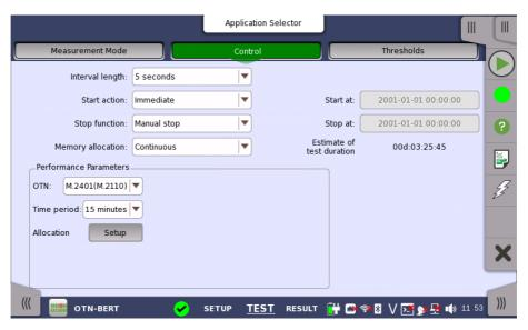
This screen allows you to configure the test mode and other general parameters related to the test.
