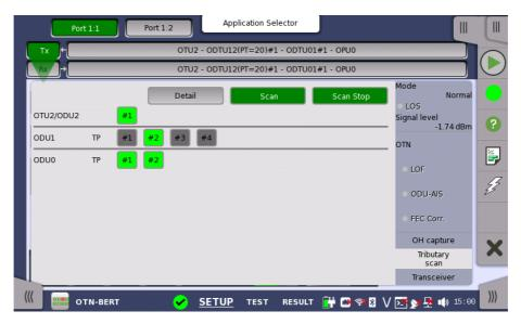
A *Tributary scan* detects errors and alarms over multiple Tributary Ports depending on the current mapping settings at the receiver port. The screen displayed by the **Tributary scan** button can be used to acquire the tributary status information.
