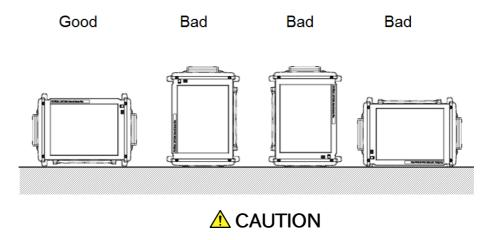
If the MT1100A is not installed in the "correct" orientation as above, a small shock may turn it over and harm the user.
