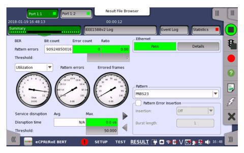
This screen contains a summary of the results of the eCPRI/RoE BERT test. The information includes such things as number of pattern errors, average and maximum disruption time, and number of exceeded thresholds.
