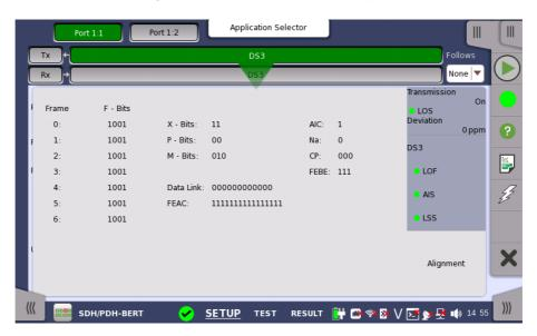
Alignment status when the frame type is C-bit
