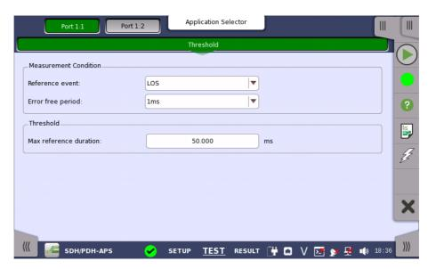
This screen contains the parameters for setting up the threshold values for alarms/errors and Pass/Fail status.
