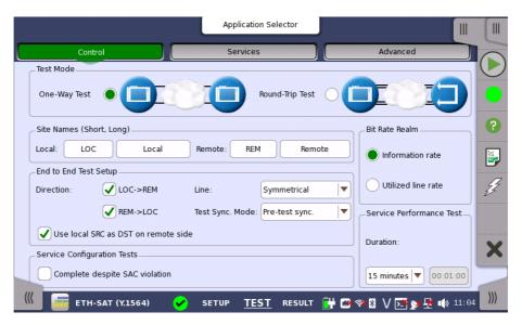
This screen allows you to configure the test mode and other general parameters related to a <u>Service Activation Test</u>.
