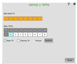
This dialog box allows you to define OTUk frame mapping.
