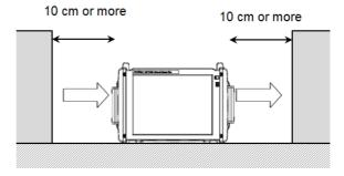
In this instrument, cooling air is taken in through the left side panel, and hot air is exhausted through the right side panel. When using two or more instruments side-by-side make sure that hot air exhausted from one unit is not taken into the adjacent unit, otherwise overheating may occur.
