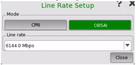
Touch **CPRI** or **OBSAI** and select a line rate. Select the bit rate of the line from the drop-down menu.
