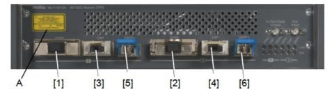
Figure 3: Locations of Laser Beam Aperture (MU110012A)
