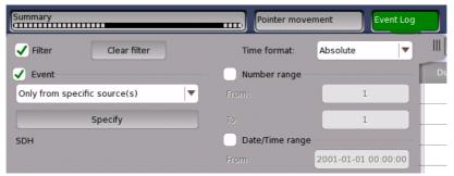
For an event to be displayed, it must pass the **Event** filter, the **Number range** filter and the **Date/Time range** filter if they are all enabled.
