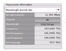
Touching **Channel** or **Wavelength** value opens the dialog box to set the wavelength.
