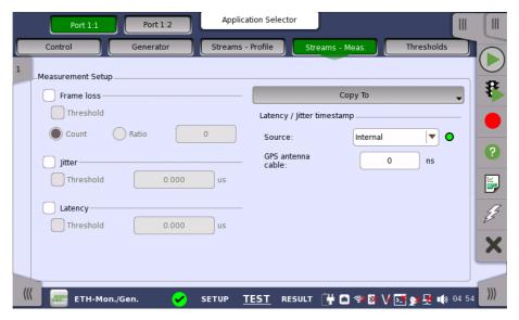
This screen allows you to configure Frame Loss, Jitter, and Latency.
