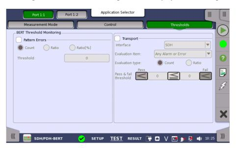
This screen contains the parameters for setting up the various threshold values (i.e. limits) for errors and Pass/Fail status that are used during the monitoring.
