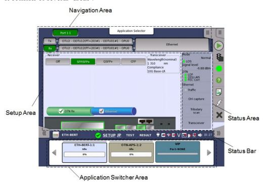
• The *navigation area* at the top of the screen contains a number of buttons representing a structure for the current interface, which allows you to select a specific port, transmitter/receiver and layer.
