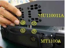
3. Tighten the four screws (shown in yellow circle) using Z1862A, with holding MU110011A by the other hand.
