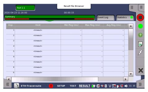
This screen shows the status/results of a running Traceroute test, or the results of the most recently completed test.
