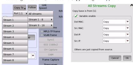
When copying settings to all streams, it is available to change MAC or IP address with selecting Variable enable check box. If the check box is not selected, same address is copied to all streams.
