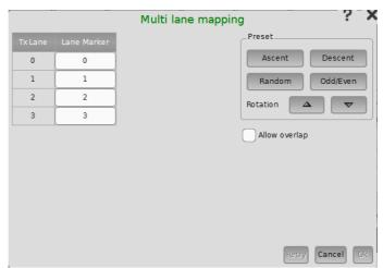
The number of lanes depends on the interface type. Touching Lane Marker field allows to set the PCS lane marker.
