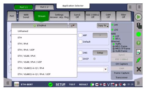
The quick selection menu contains a number of predefined frame configurations (e.g. ETH/VLAN/IPv4). The detailed mode dialog box allows you to specify the frame configuration yourself and also provides you with access to all configuration parameters available for the individual layers.
