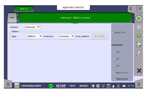
This screen allows you to specify the frame structure of the currently selected port.
