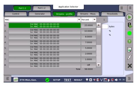
At the top of the slide-out list you can switch between MAC, IP, and VLAN information as stream identification.
