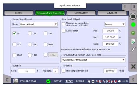
This screen allows you to configure the following parameters related to an RFC 2544 Throughput and Frame Loss test:
