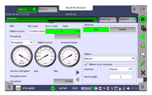
During a measurement, Measurement start time, Elapsed time, and Remaining time of measurement are displayed in Navigation area. Remaining time of measurement is not displayed if Stop function is set to **Manual stop** in Control screen.
