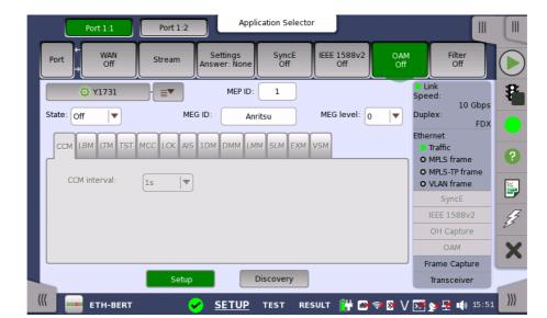
Y.1731 protocol setup Selecting the Y.1731 protocol will display the screen shown below.
