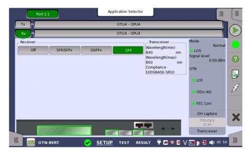
This screen allows you to make the physical setup of the receiver in OTN mode. It can also be used to inspect the current status of the selected port by the button in Navigation area.
