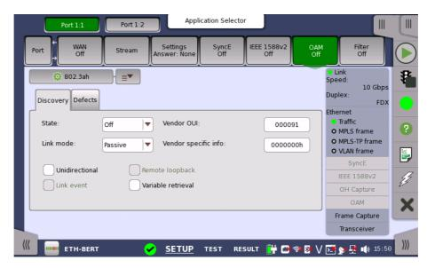
OAM (Operation, Administration and Management) is a group of management functions that provides system or network fault indication, performance monitoring, security management, diagnostic functions, configuration and user provisioning.
