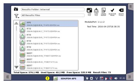
Creating a *workspace* for a previous test allows you to view the test results in the GUI and also to rerun the test if required (either with the same setup or with changed parameter settings). You are brought directly to the *Test Results* screen when you touch the **VIEW FILE/LOAD FILE** button, but can navigate to the other screens in the workspace from there.
