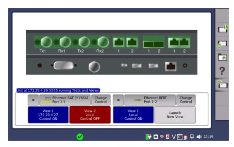
Each application is associated with up to two Views, Only one View can have control at a time. Having control gives user full access to all application functions, including modification of setting parameters, load and save functions, and running the test. Without control, users are only allowed to browse the current application settings and results.
