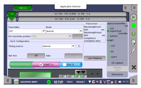
This screen allows you to enable the optical or electrical interface of the SONET transmitter. It can also be used to inspect the current status of the selected port.
