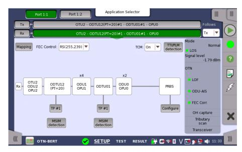
This screen allows you to configure OTUk frame of the currently selected receiver. It can also be used to inspect the current status of the selected port in a separate screen.
