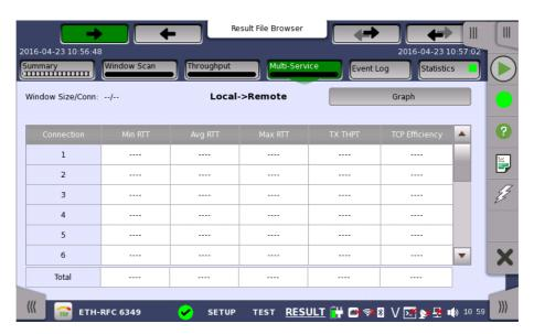
This screen presents results by each TCP connection of RTT, Throughput and TCP Efficiency. Use the **Graph** and **Table** buttons to switch between the tabular form and a graphical presentation of the results.
