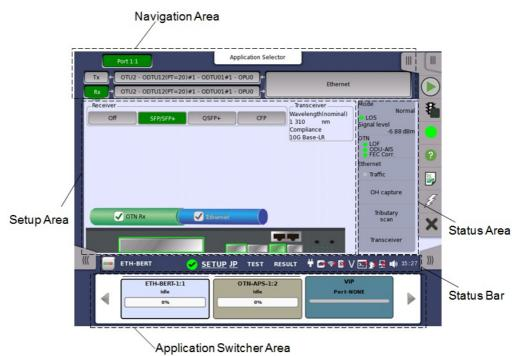
• The *navigation area* at the top of the screen contains a number of buttons representing a structure for the current interface, which allows you to select a specific port, transmitter/receiver and layer.
