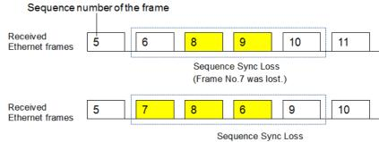
(Frame No.6 has delayed by two frames.)
