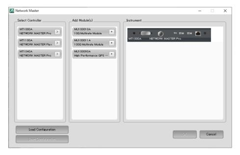
3. Set configuration of the Network Master by clicking options in **Select Controller**, and **Add Module(s)**.
