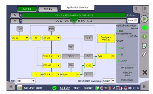
The general principle in setting up the SONET frame is to select the relevant values for the various containers in the multiplexing structure. This is done either via a drop-down menu or via a launched dialog box, by touching a drop-down menu or a button in the frame structure diagram.
