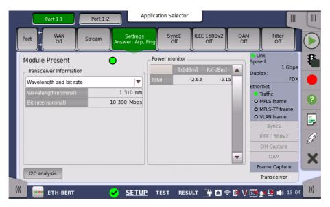
This screen presents status information about the optical transceiver (Pluggable module installed on the connector panel).
