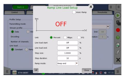
The line load unit can be specified from Percent, Mbps, and IFG.
