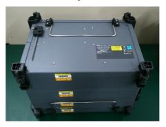
4. Insert Z1862A to holes (shown by the yellow circle) on rear side of the Power Supply Module.
