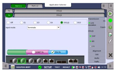
For the switching method between PDH Rx and DSn Rx, refer to <a href="Physical Setup">Physical Setup</a> in "E1 Setup and Status". Touch <a href="DS1/J1">DS1/J1</a> radio button. Touching <a href="Off">Off</a> radio button disables the receiver.
