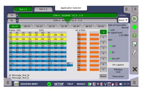
This screen shows SDH capture status information for one frame at a time. The frame number captured in one time is 64. Touch the frame selection buttons to select which frame to display.
