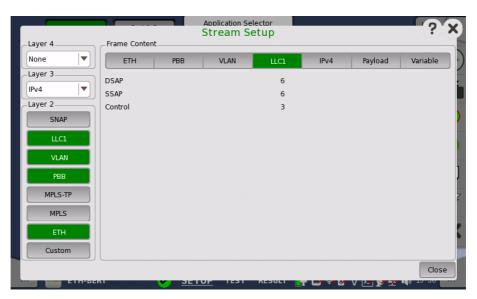
The **DSAP**, **SSAP** and **Control** fields are set automatically, based on the upper protocol layer.
