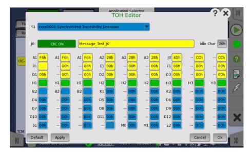
The setup principle is the same in this editor dialog box as in the SONET structure. Touching a button or opening a drop-down menu will open for new editor dialog boxes, new value selections etc.
