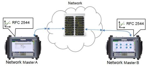
When the test mode is set to **Single ended network test** in the RFC 2544 application, test can be performed cooperating with opposed side reflecting equipment by switching Network Master B application to Reflector as shown in figure below.
