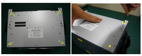
4. Place MU110001A on MU110011A. The attaching procedure of MU110001A is the same as attaching MU110011A to MT1100A.
