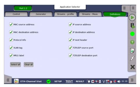
This screen is where you specify which frame characteristics are considered when performing the channel separation (i.e. which frame characteristics are active during the test). The maximum number of channels is 231.
