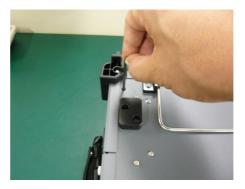
6. After loosing the four screws, lift up the Power Supply Module with holding both sides. You can see the side panel of the Multirate module as below.
