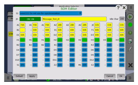
The setup principle is the same in this editor dialog as in the SDH structure. Touching a button or opening a drop-down menu will open for new editor dialog boxes, new value selections etc.
