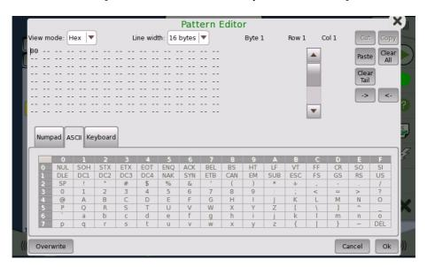
You use the numpad to edit the pattern in the *Hex* and *Bin* view modes, and use either the ASCII table or the keyboard to edit in *ASCII* view mode.
