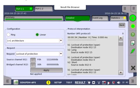
This screen shows a protocol interpretation for the selected port (i.e. detailed decoding information about K1 and K2 during the test). It also contains a set of parameters that allow you configure the requests used in the test.
