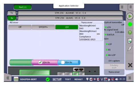
This screen allows you to make the physical setup of the receiver in SDH mode. It can also be used to confirm the current status of the selected port.
