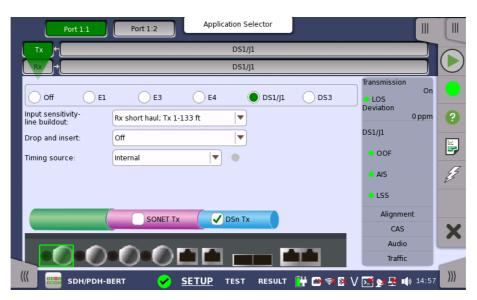
For the switching method between PDH Tx and DSn Tx, refer to <u>Physical Setup</u> in "E1 Setup and Status". Touching **Off** radio button disables the transmitter.
