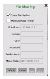
• IP Address: The IP address of the networked PC
