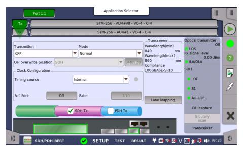
This screen allows you to enable the optical or electrical interface of the SDH transmitter. It can also be used to confirm the current status of the selected port.
