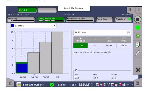
Touching the **Configuration Test** button in the navigation area will display the screen shown below.
