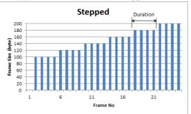
If the traffic duration is set to *Continuous* on the **Generator** screen, the step sequence will be repeated indefinitely. If traffic duration is set to *a number of seconds*, the step sequence will be terminated when the specified total period has elapsed. Similarly for traffic duration set to *a number of frames*, the step sequence will be terminated when the total number of transmitted frames reaches the specified count.
