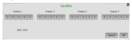
In the Sa-Bits dialog box, change the individual Sa-bits by touching on the relevant bit keys - this will toggle the bit key's binary value from logic 1 to 0 or vice versa. Touch Ok to accept the changes and close the dialog.
