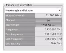
Touching **Channel** or **Wavelength** value opens the dialog box to set the wavelength.
