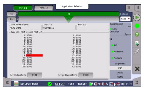
This screen gives information on the CAS (Channel Associated Signaling) signaling when available. It displays the state of the four signaling bits in both directions for all 30 channels. Activity is indicated with bold characters.
