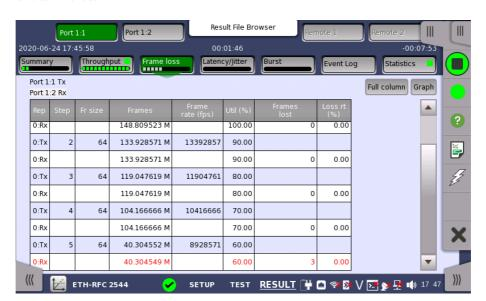
This screen allows you to configure the following parameters related to an RFC 2544 Frame Loss test:
