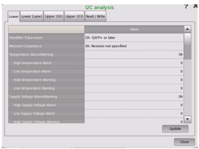
This dialog box allows reading/writing information into the registers of the optical transceiver via  $\rm I^2C$  (Inter-Integrated Circuit) interface.
