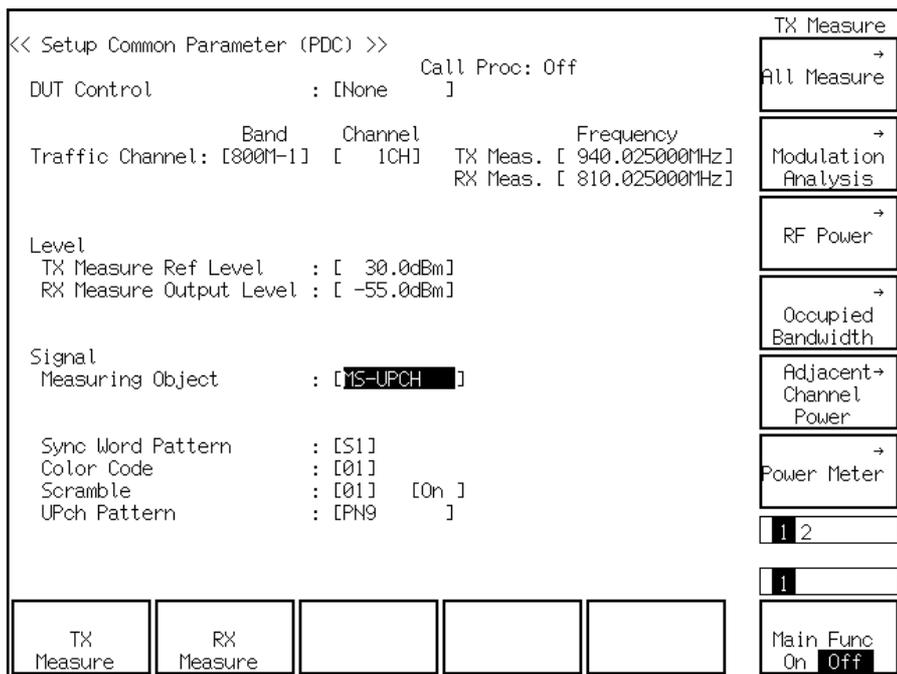
Setup Common Parameter screen when MS-UPCH is selected for Measuring Object
